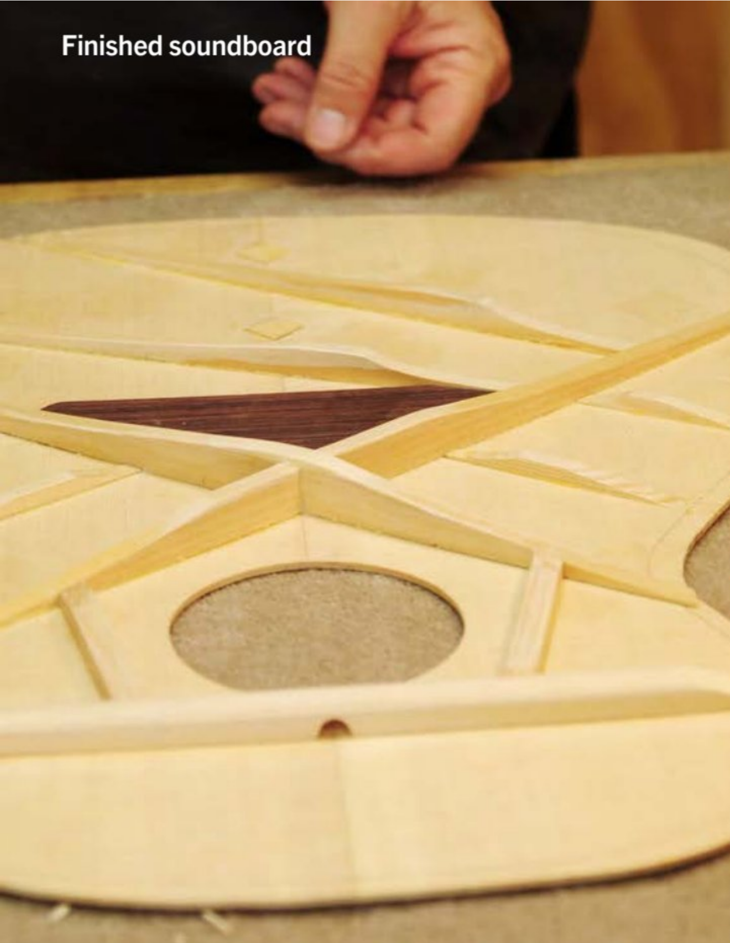
Checking notches for top bracing to allow top to sit down on sides
