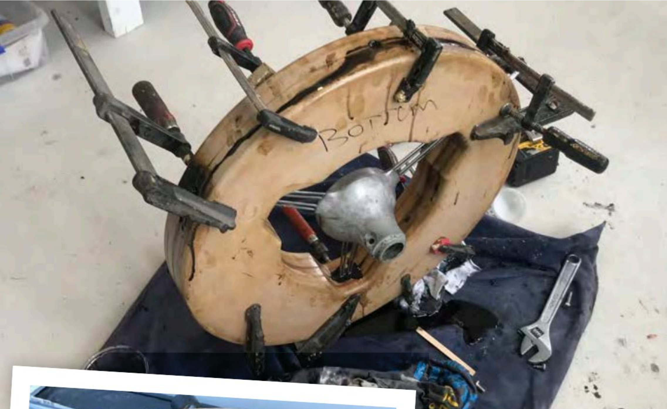
Older style wire-sprung wheel-rim repair process: well clamped
