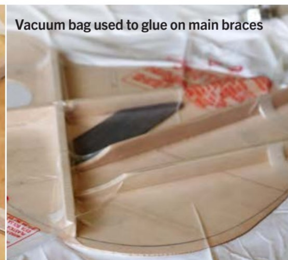
Glue on main X-brace and harmonic bar prior to vacuum bagging
