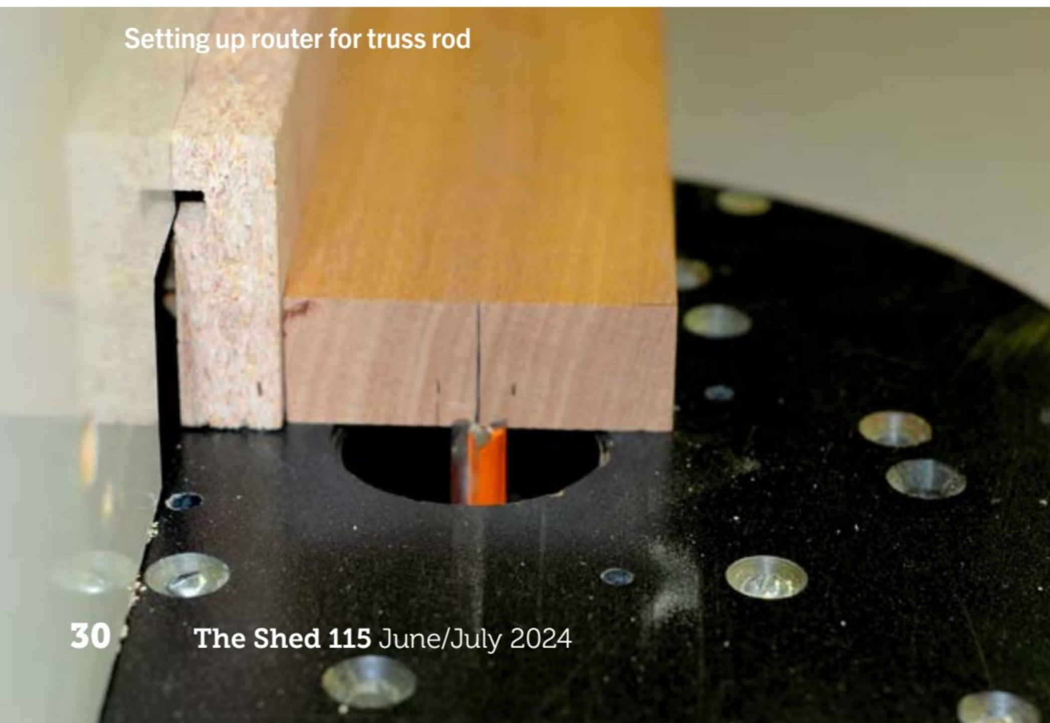
Showing scarf joint planed, reinforcing wings on, and truss rod slot
