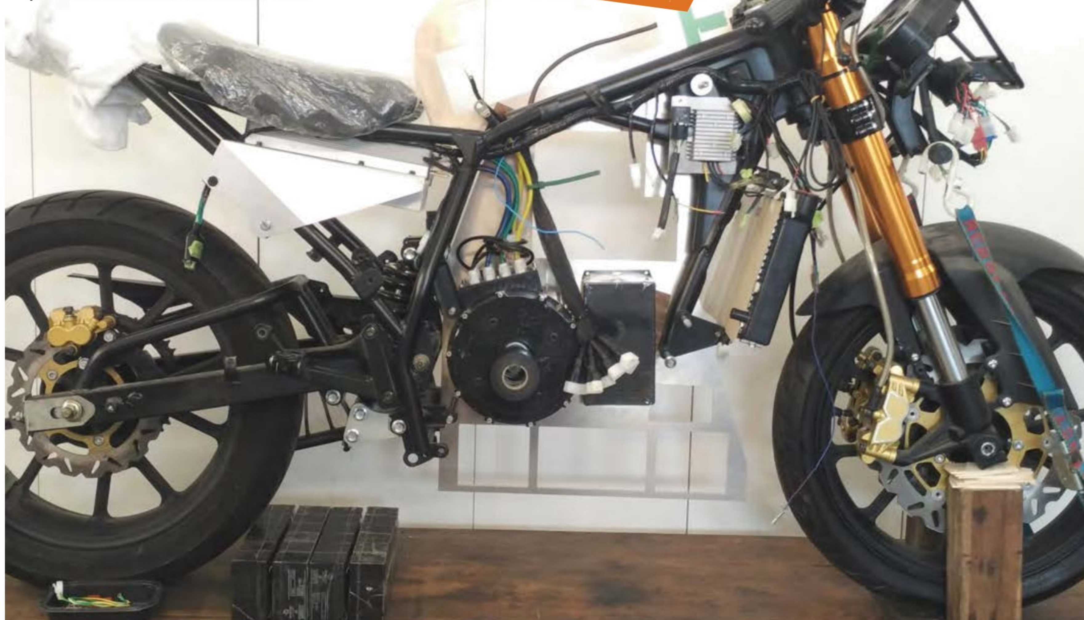
Donor bike with water-cooled three-phase electric motor and radiator fitted
