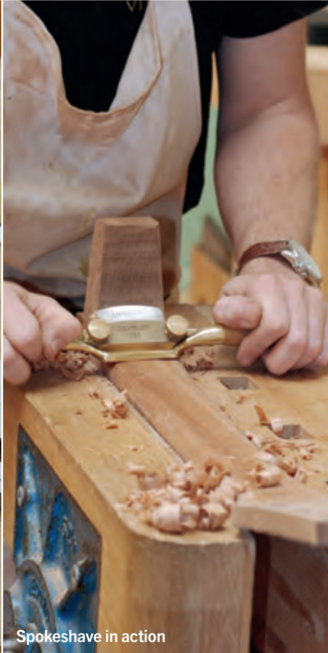
Planing tapers into sides of heel
