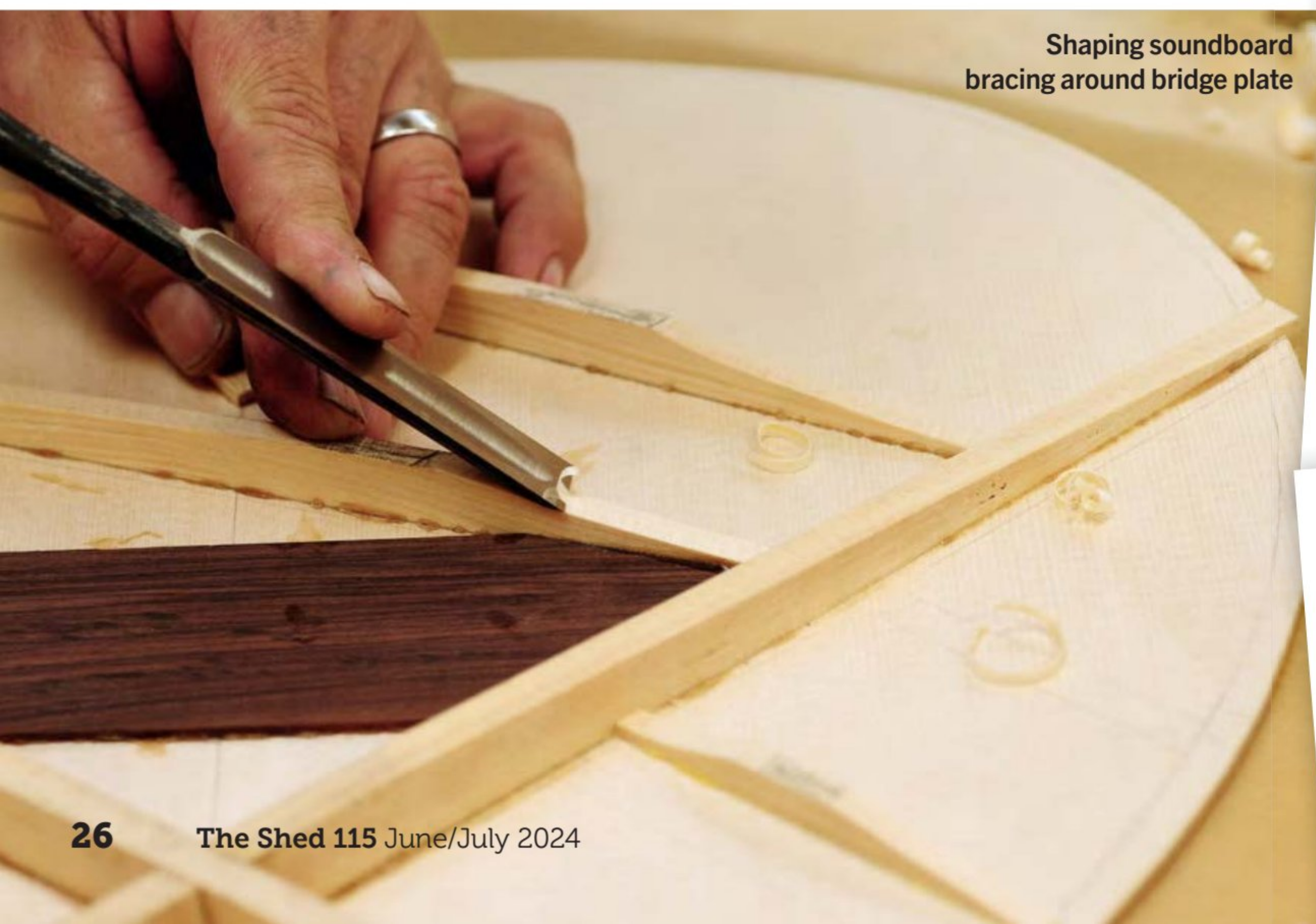
Soundboard braces scalloped and tapered
