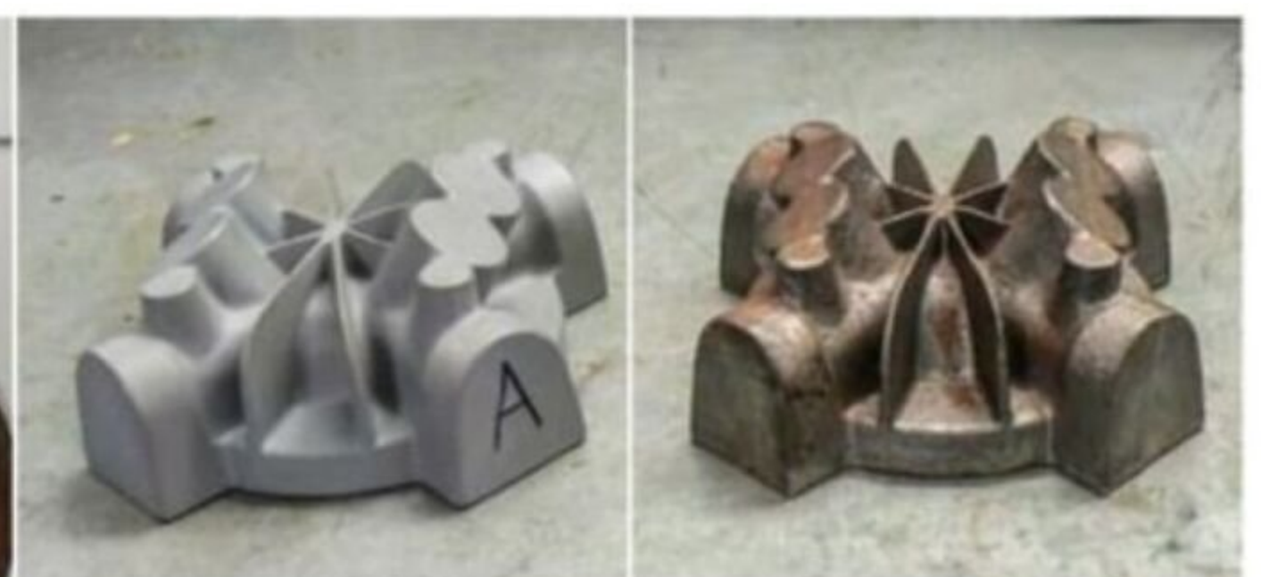
Above: The wooden pattern for the head of the board-track racer's engine (left) and an unfinished cast iron head (right)
