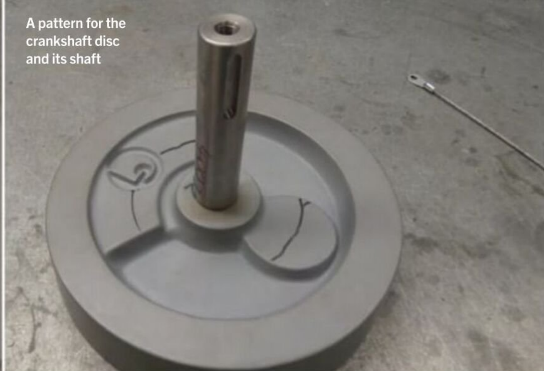
The pattern for one of the crankshaft's discs; Chris Gordon's symbol – a G-shaped arrow – is cast into the discs and the crankcase
