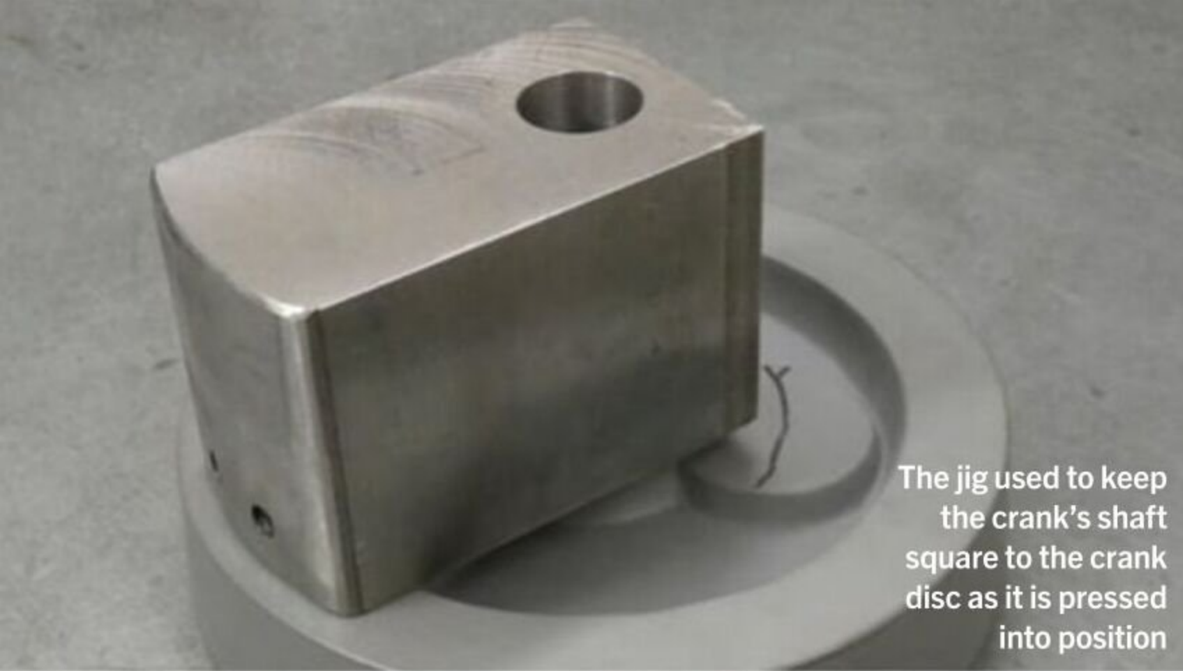
The jig used to hold the crank discs in position as the crankshaft's components are pressed together; a force of nine tonnes is needed
