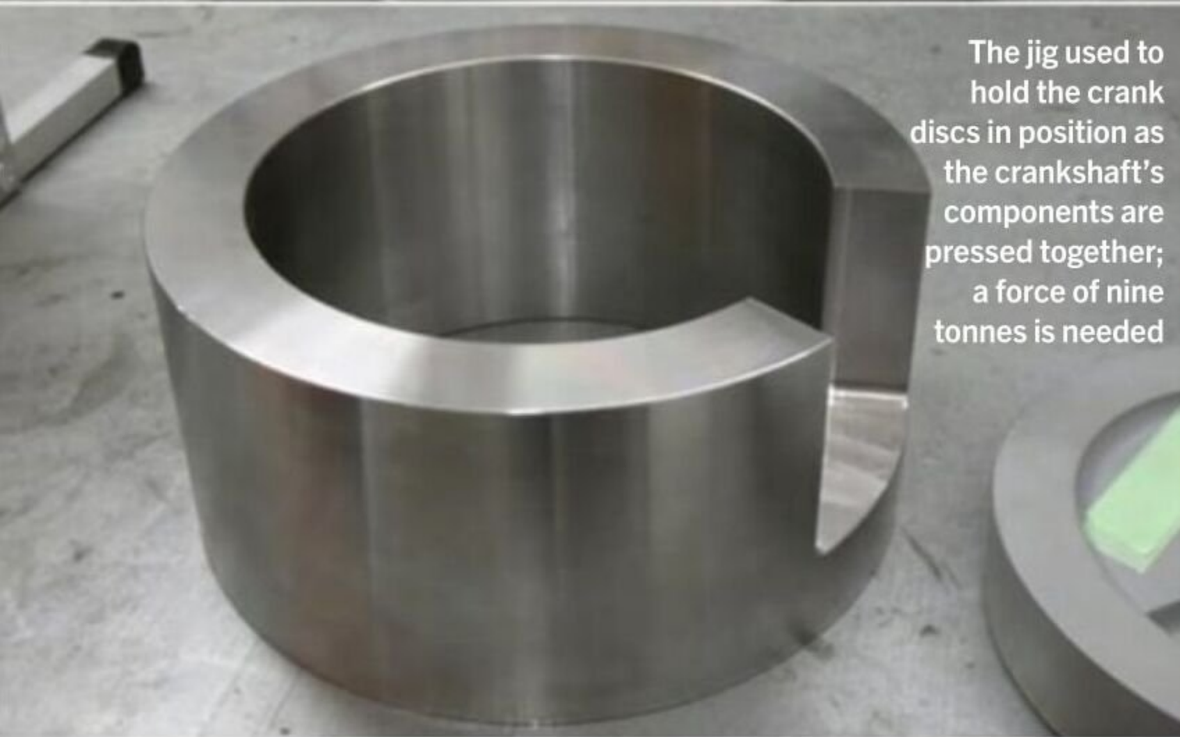
The jig used to keep the crank's shaft square to the crank disc as it is pressed into position
