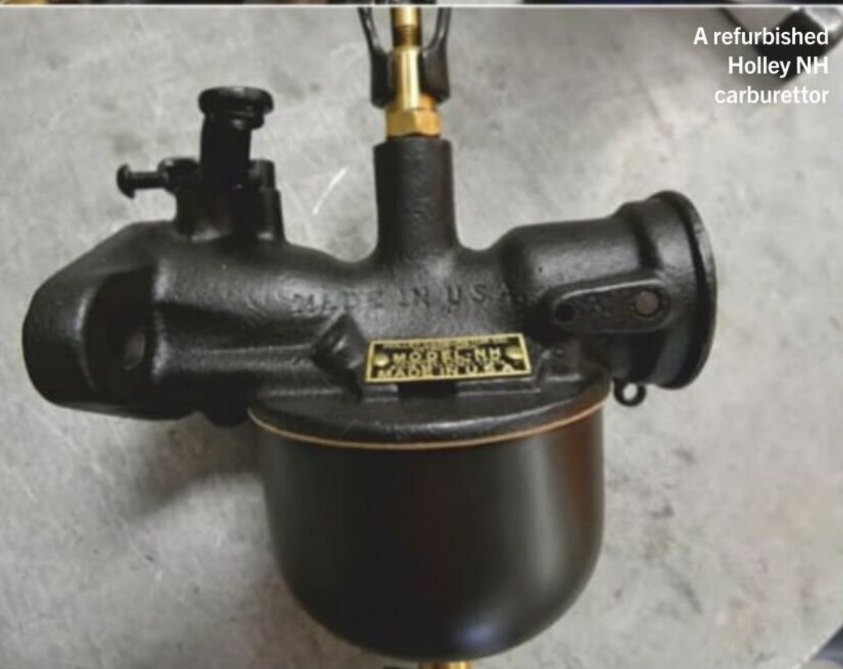
The Holley NH carburettor was original equipment on Henry Ford's Model T
