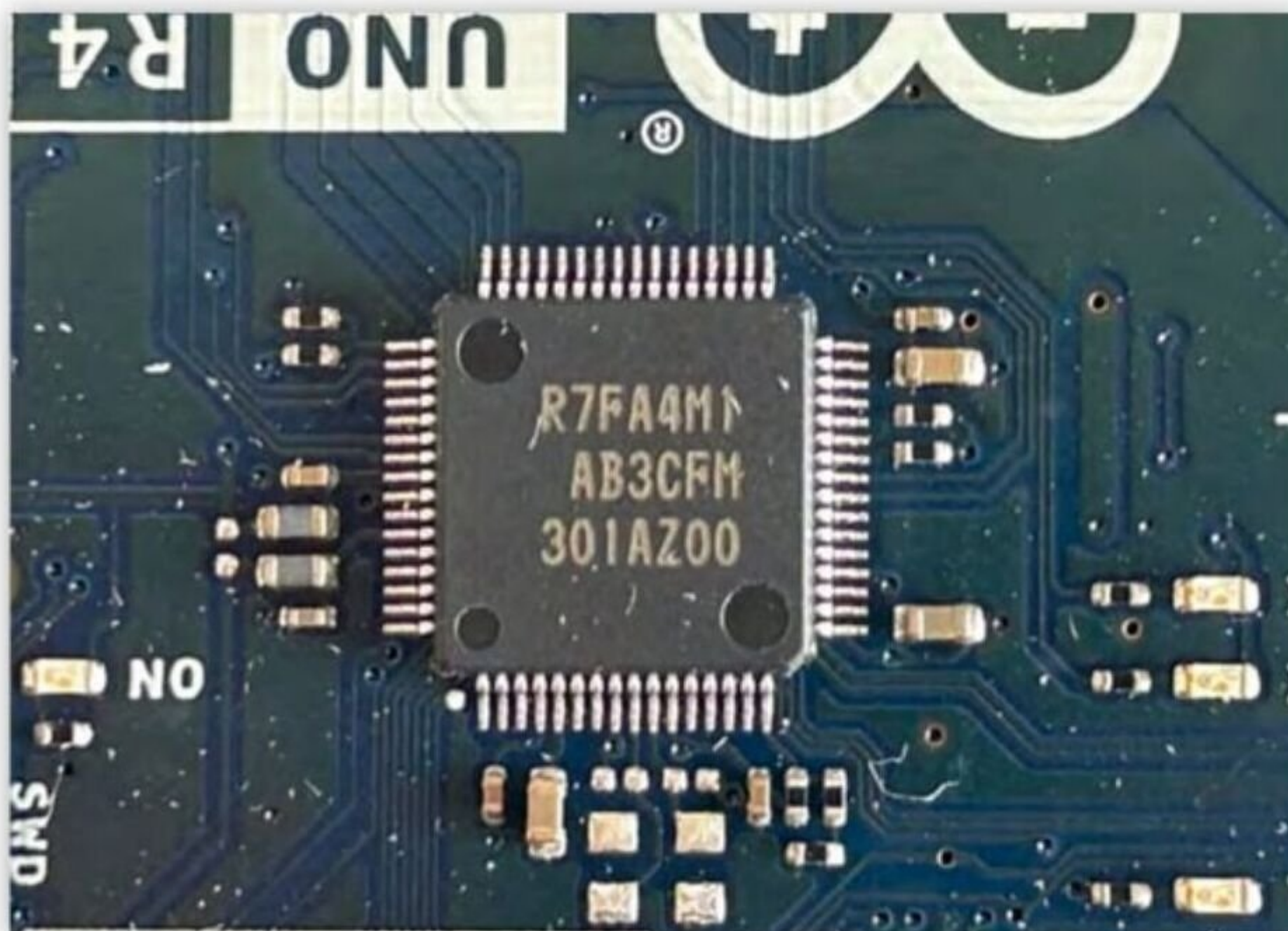
A detail of the ARM microcontroller – the core of the two Arduino models – including a DAC channel for audio conversion
