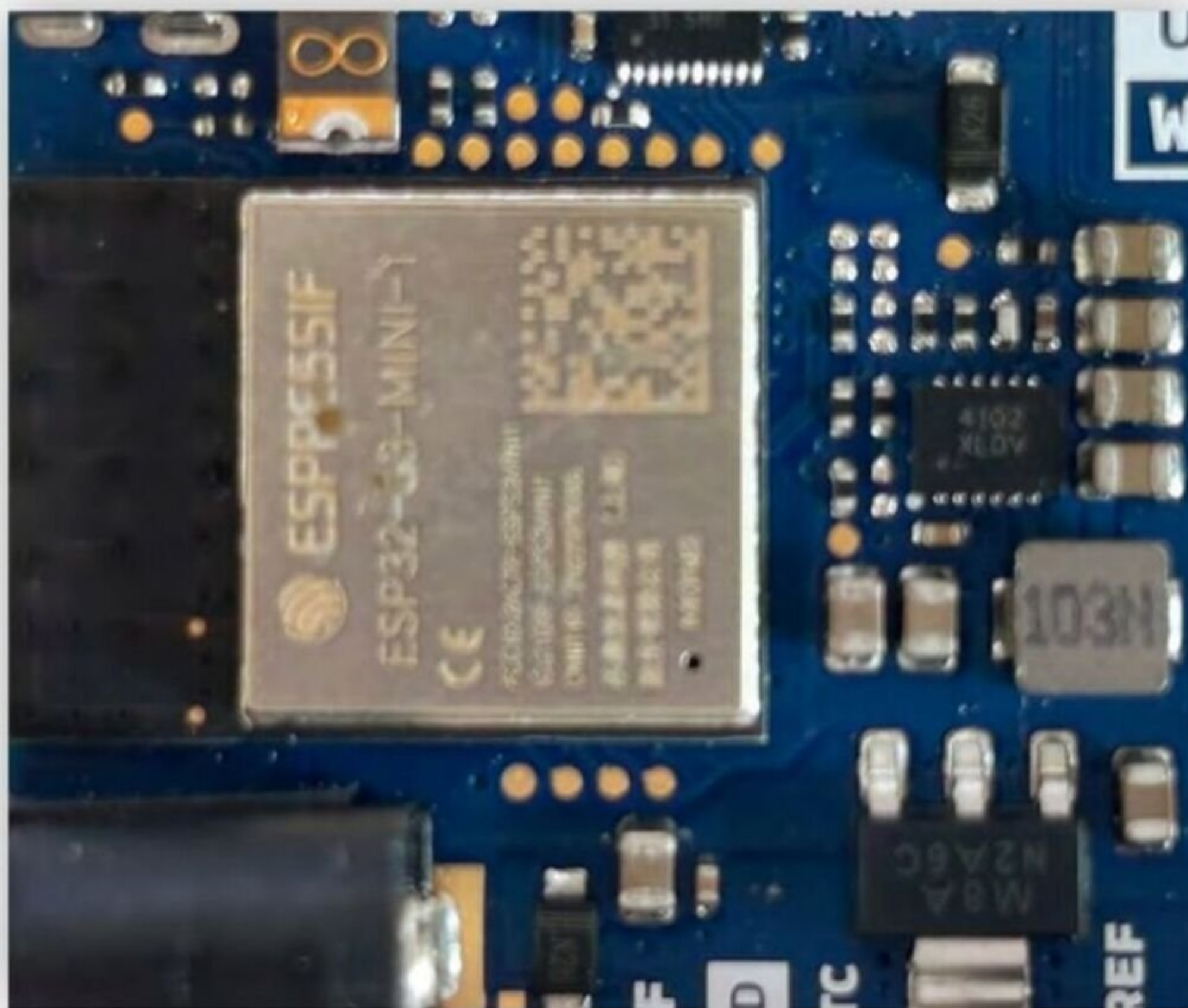
A detail of the Arduino UNO R4 Wifi – the most advanced model – showing the ESP32-S3 soldered on the board
