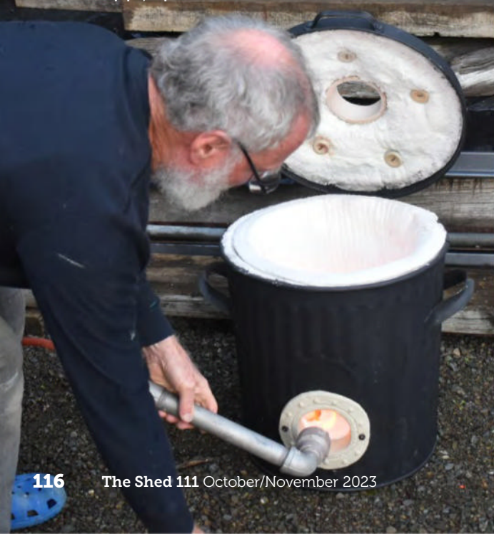
The “very commercial” burner, which Trevor made from a pipe, is placed in the base of the kiln
