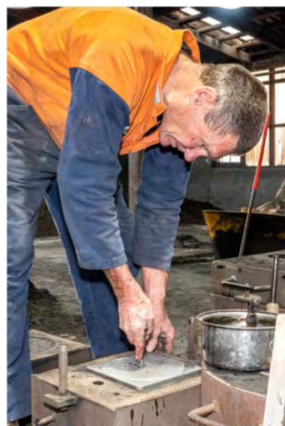
Lifting the top part of the casting box (the cope) off the pattern
