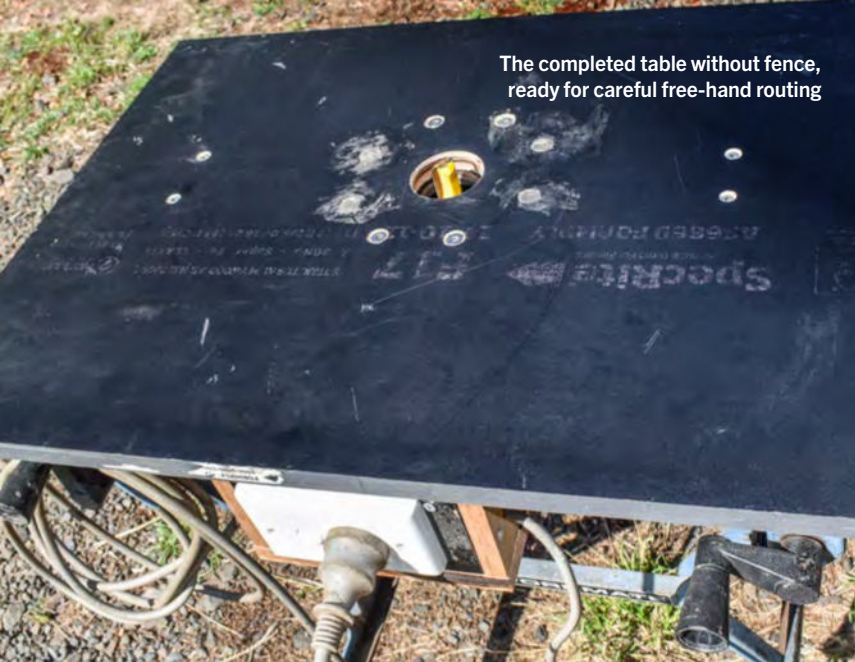
A view of the adjustment ring, the power-point box, and the router support
