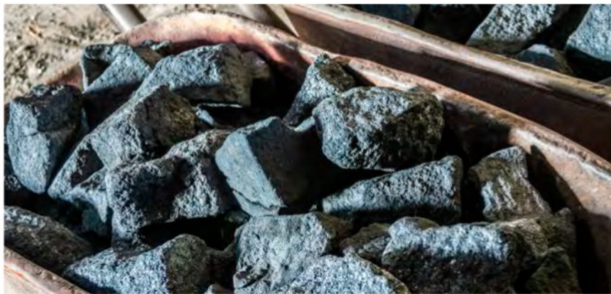
The coke used to melt the cast iron
