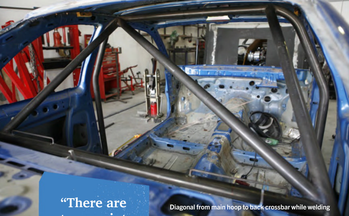
Diagonal crossbar and backstay joint
