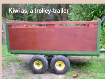
An angle frame bolted on for strength
