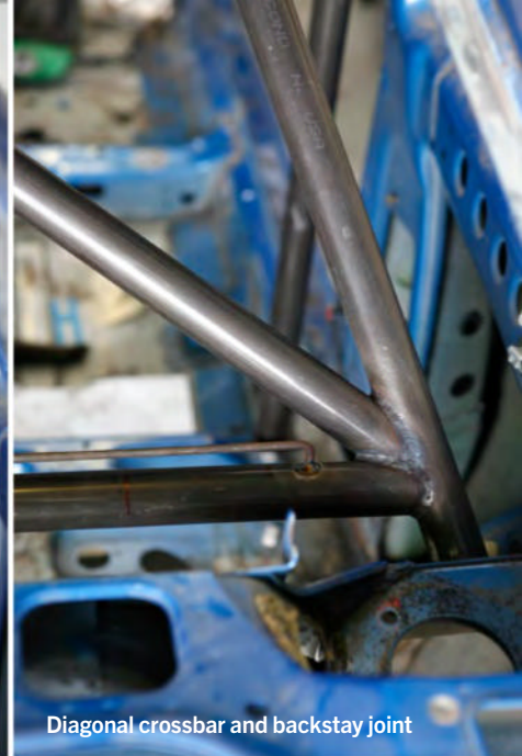
Diagonal from main hoop to back crossbar while welding
