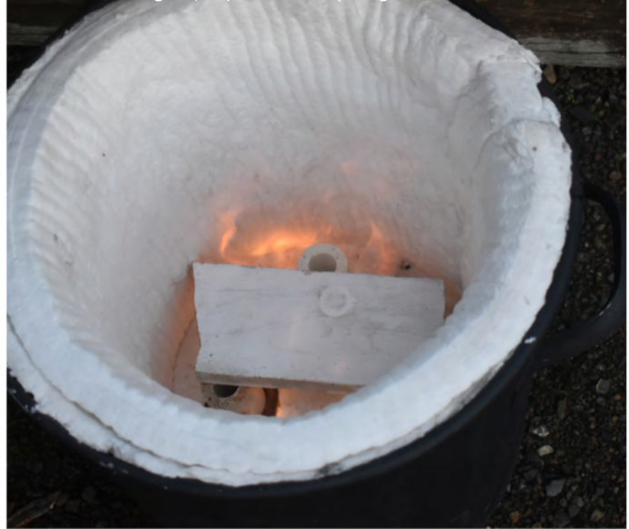
A brick of ceramic clay gives something for a pot to sit on while it’s fired. It’s amazing stuff, “a spin-off from the space age”
