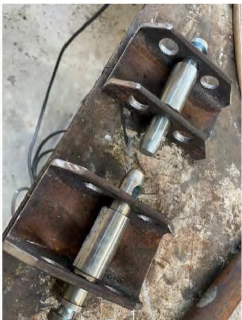
Making the quad bike attachment brackets for the linchpin connections
