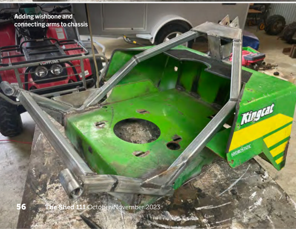
Initial positioning of the new chassis over the cutting deck
