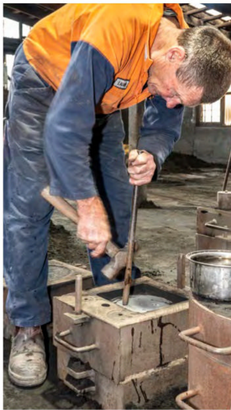
Lifting a pattern from the casting box
