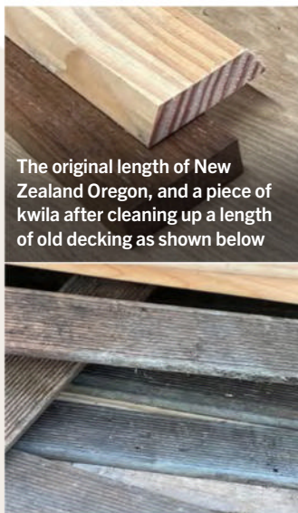
The New Zealand Oregon and kwila just prior to going through the thicknesser. I was trying to see if by propping the ends I could make them thinner and keep the middle thicker, a technique I'd seen in a YouTube clip
