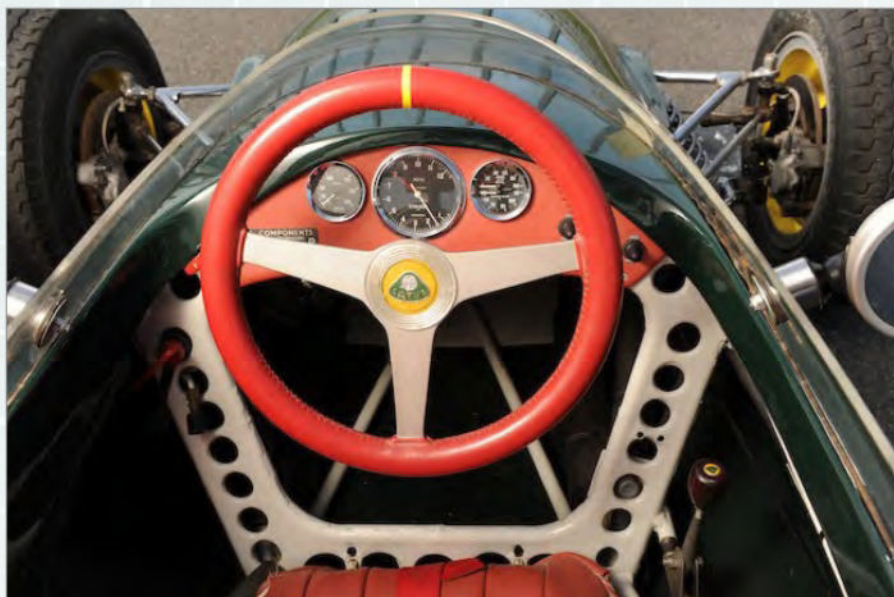
Fig. 1. A 1961 Lotus 20 with dimpled hole bulkhead
