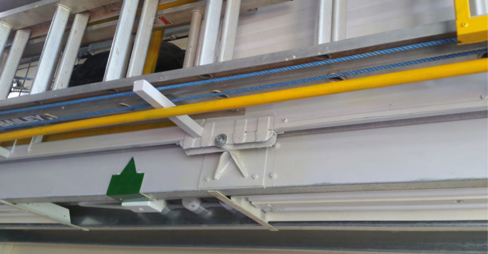
Photo 46 — The pivot for the ladder storage, and one of the pegs supporting the stored ladder
