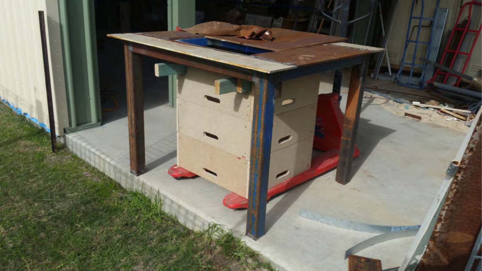
Photo 36 – The stands can be configured to allow the jack to lift any bench easily
