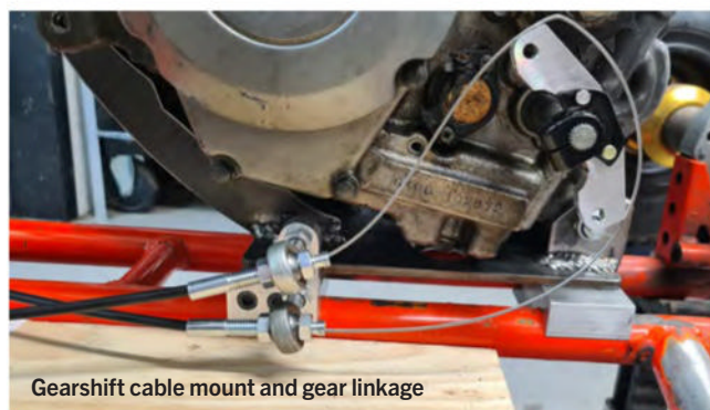
Cable operated paddle gear shifter components
