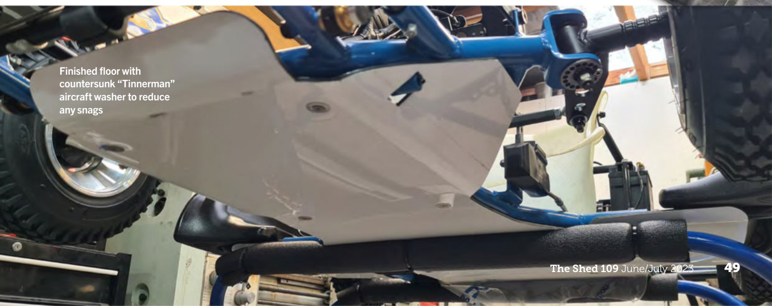
Making up the new full size floor pan from an ACM sheet
