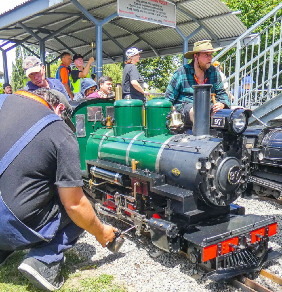
A steam locomotive needs constant attention: steaming coal and water have to be continually replenished, and the oil can is regularly in action
