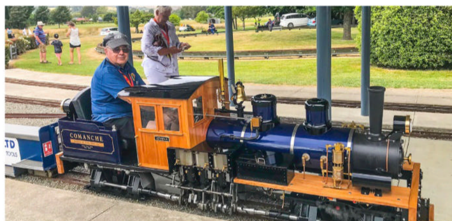
Designer Dave Giles at the controls of a Shay locomotive built by a CSME member. Dave's design is based on a North American geared logging locomotive. He has personally built eight of these very large devices, each taking two years of 40-hour weeks
