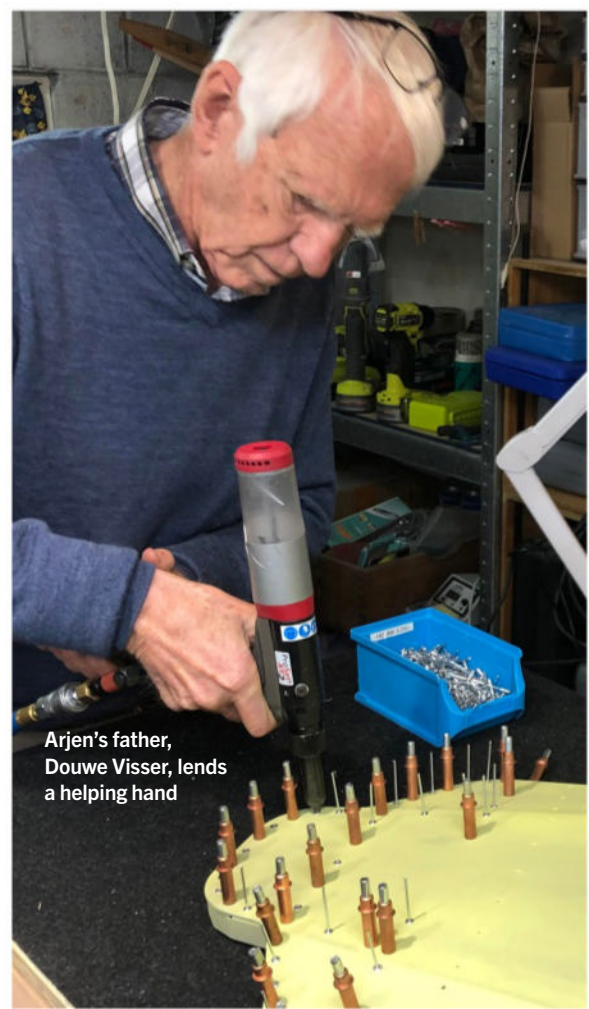
Clecos (copper and black-coloured clamps) are used to hold everything in place before riveting
