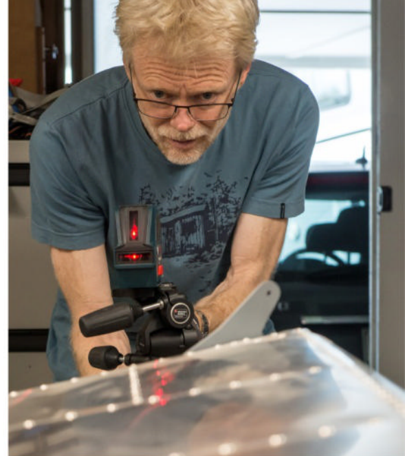
Using a regular builder's laser tool is essential to ensuring all flying surfaces are straight and true
