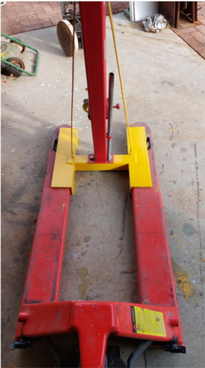
Photo 6: The base has a working clearance between the tines of the pallet jack so it can be picked up easily
