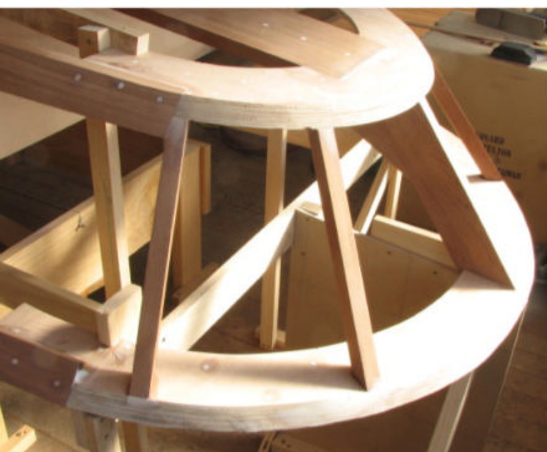
The stern framing is covered in three layers of thin plywood
