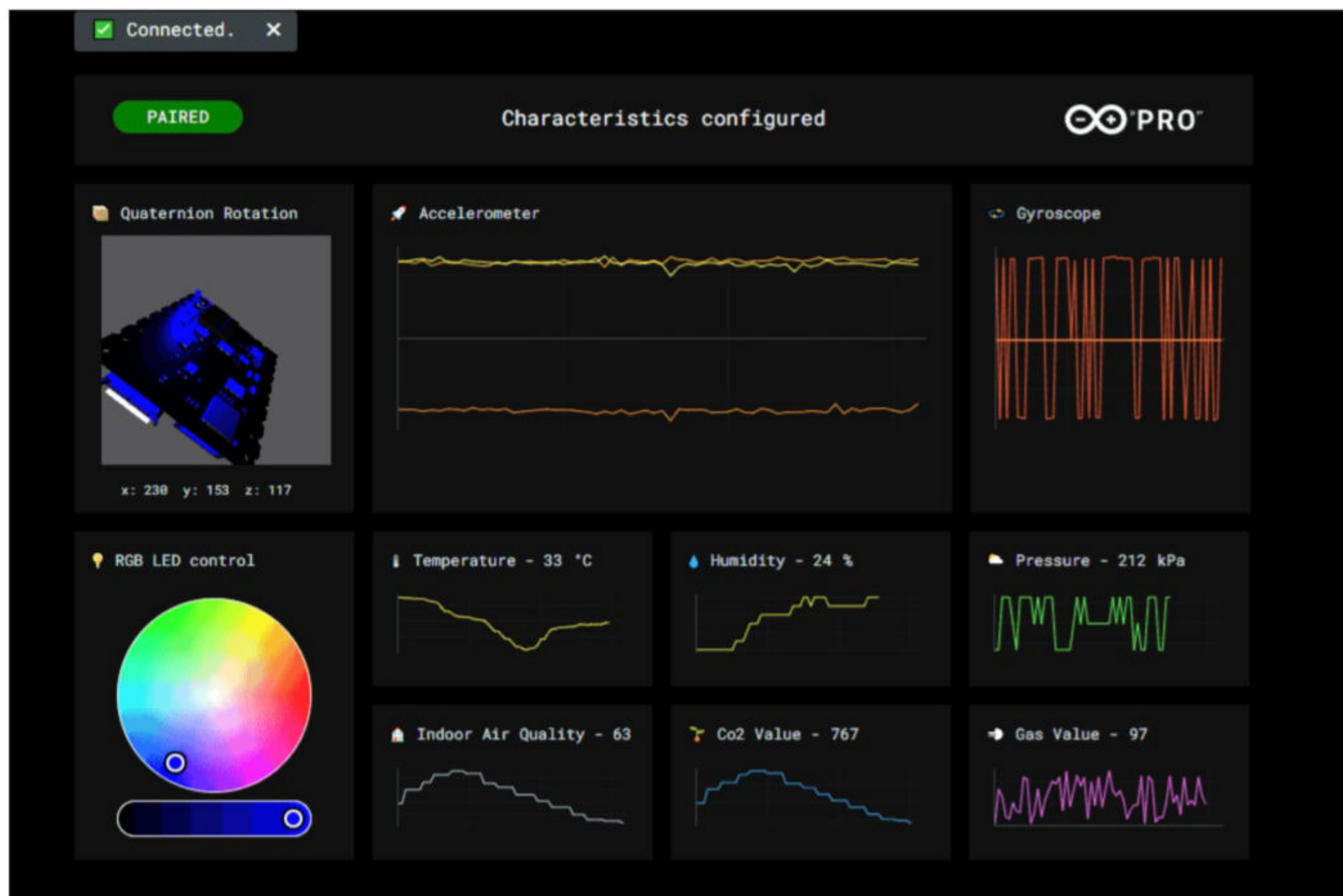
The Arduino Nicla dashboard shows in real time the state of all the sensors of the microcontroller connected through Bluetooth
