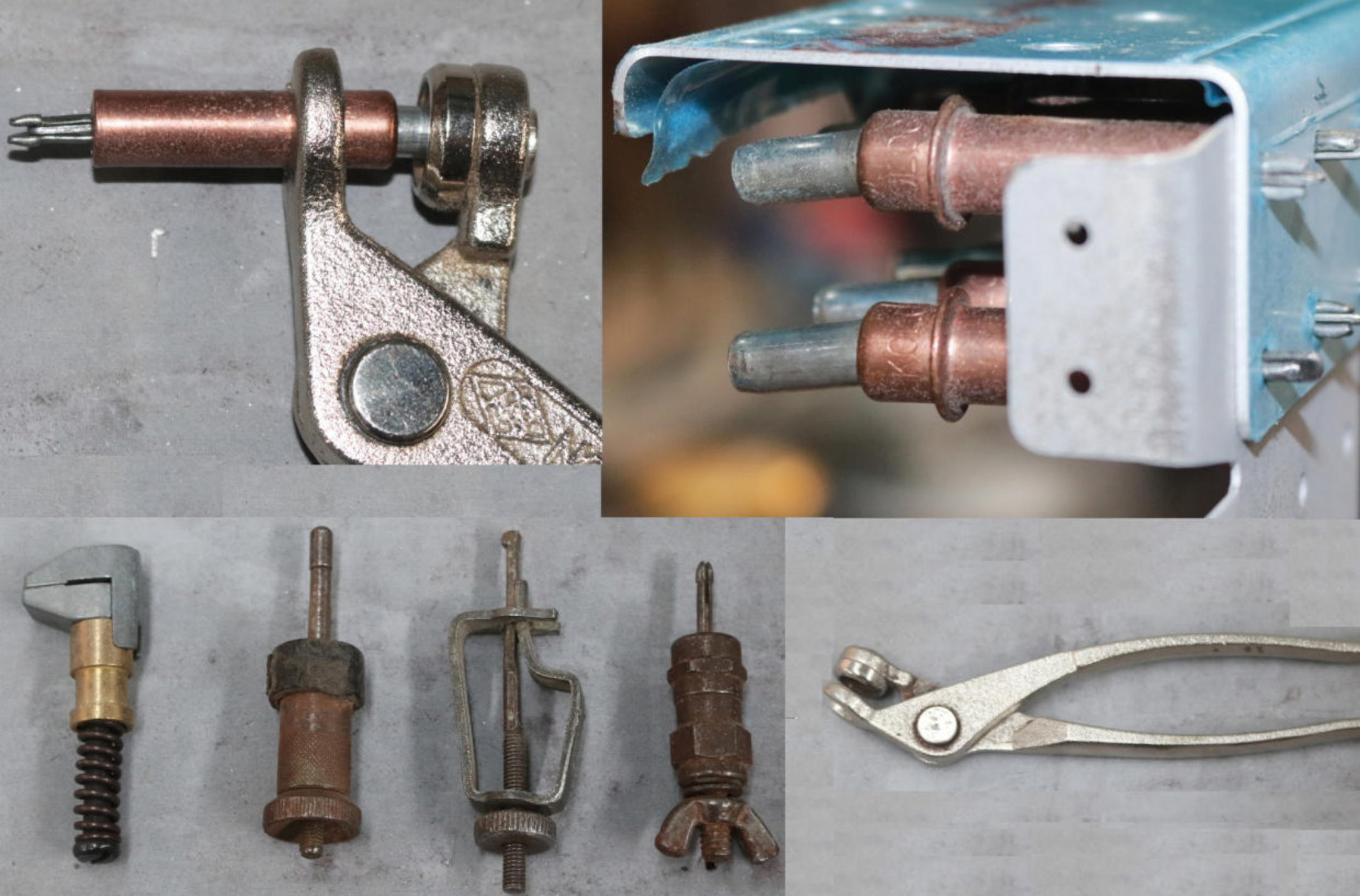
Above: The Cleco is a temporary skin fastener that holds parts you are about to rivet firmly. The top left shows it ready to insert — let go of the handle and the central pin moves forward and the jaws pull the parts tightly together. At the bottom you can see some vintage skin fasteners I found among my father's tools. The large diameter ones are 60-plus years old, but still work — it means I don't have to buy any big spring Clecos.
