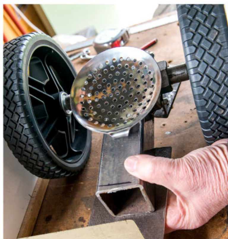
Plans, parts, and a ready-to-weld back end made from box section, a spoon seat and freewheeling plastic wheels on a drilled and tapped axle
