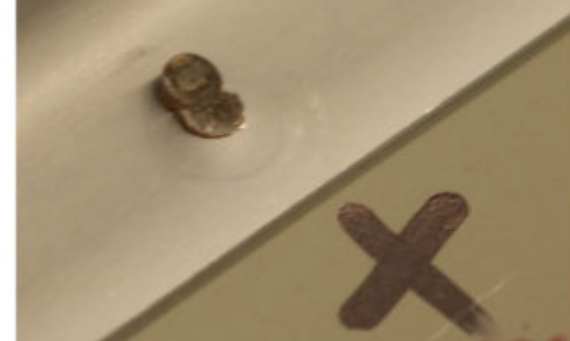
Bad rivets. Above is a close-up of a section of the tailplane; the rivets marked were not very flush and were marked, removed, and replaced. In the middle you see what looks like an extra rivet — it is. I ended up with a hole in the wrong place, so after getting advice, I put in some extra rivets, and once painted it won't show. Below you can see what happens when the bucking bar slips — instead of a nice round head it is mutilated, very weak, and needs to be replaced
