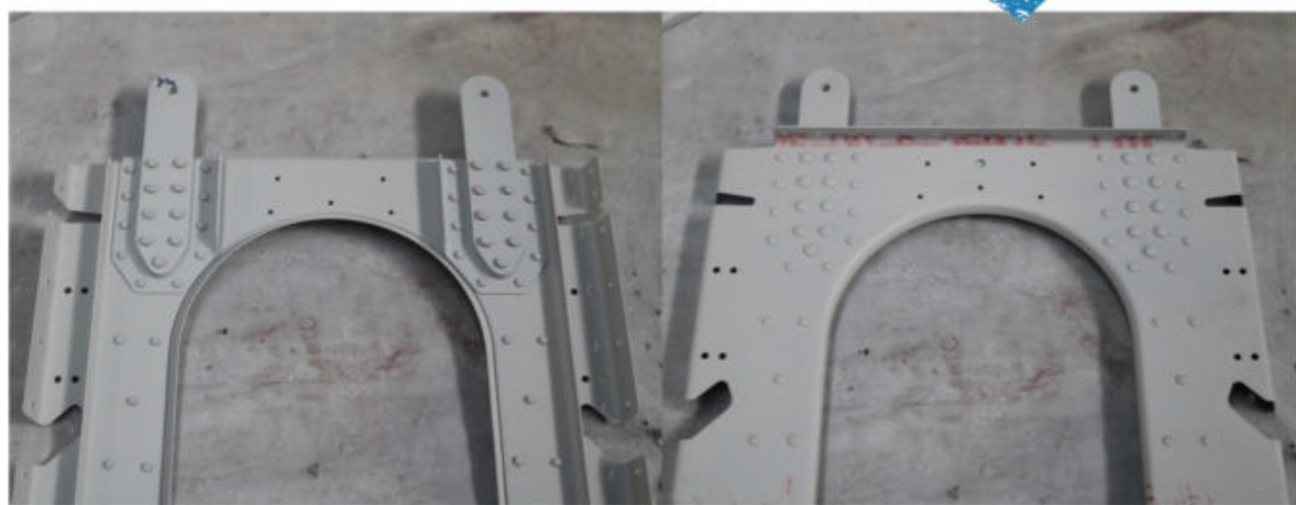
This is a good example of a riveted structure — one of the attachment points for the tail plane; the layers of metal and closely spaced rivets make it very strong but still light weight
