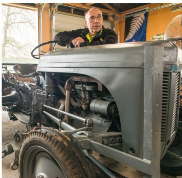
A singer sewing machine, with an electric sewing machine motor as the engine. This one has working steering, 3-point lift and a PTO (power take off)
