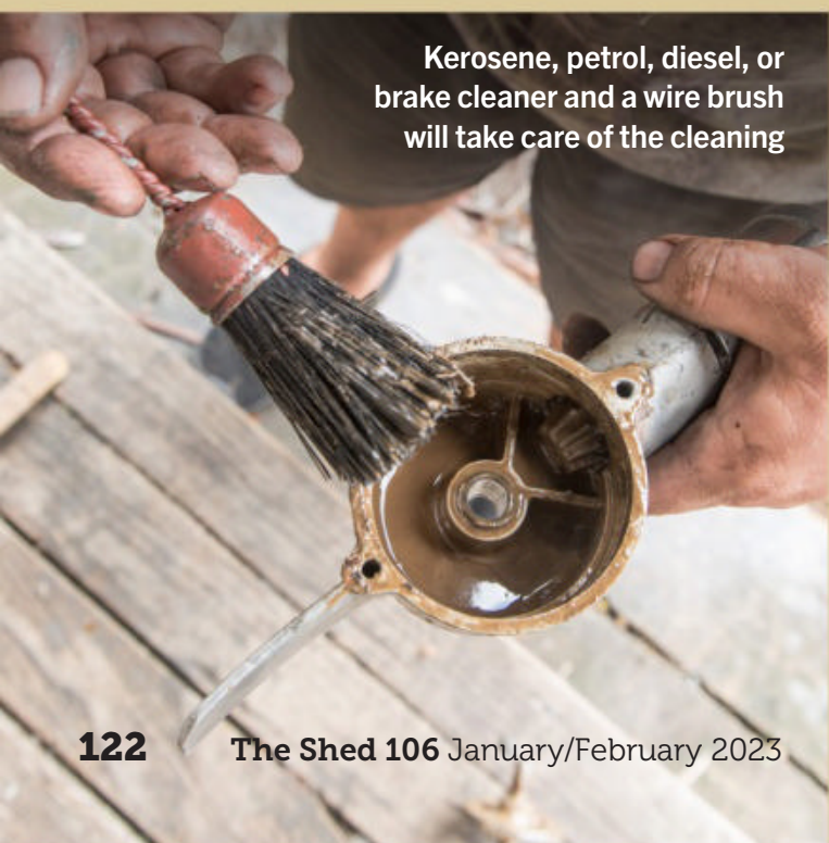
Gearbox clean — vice grips and screwdriver can be useful to gently budge stubborn bushes
