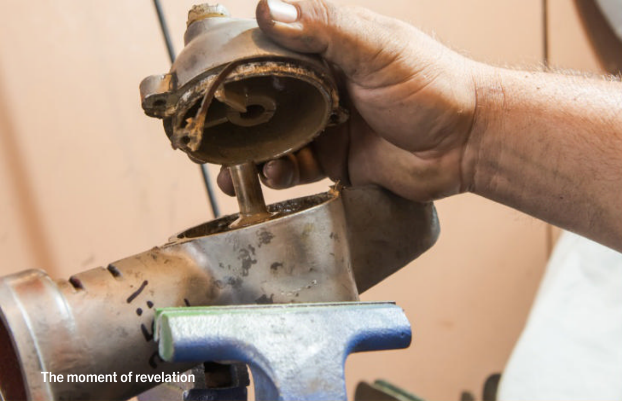
Once the bolts are extracted, use two screwdrivers in tandem and gradually pry off the gearbox cover
