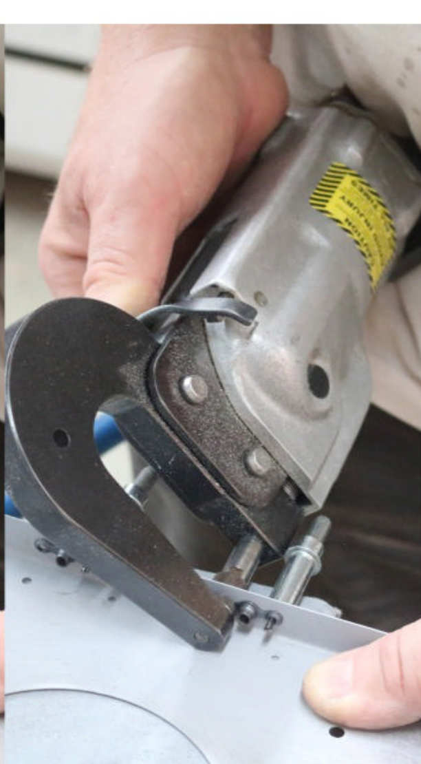
The pneumatic squeezer takes the RSI out of setting rivets — just don't get your finger trapped between those jaws when you press the trigger
