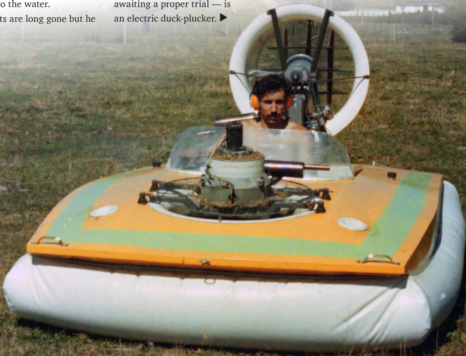
Plywood framed hovercraft with rotary Wankel motor and Hirth two-stroke for thrust
