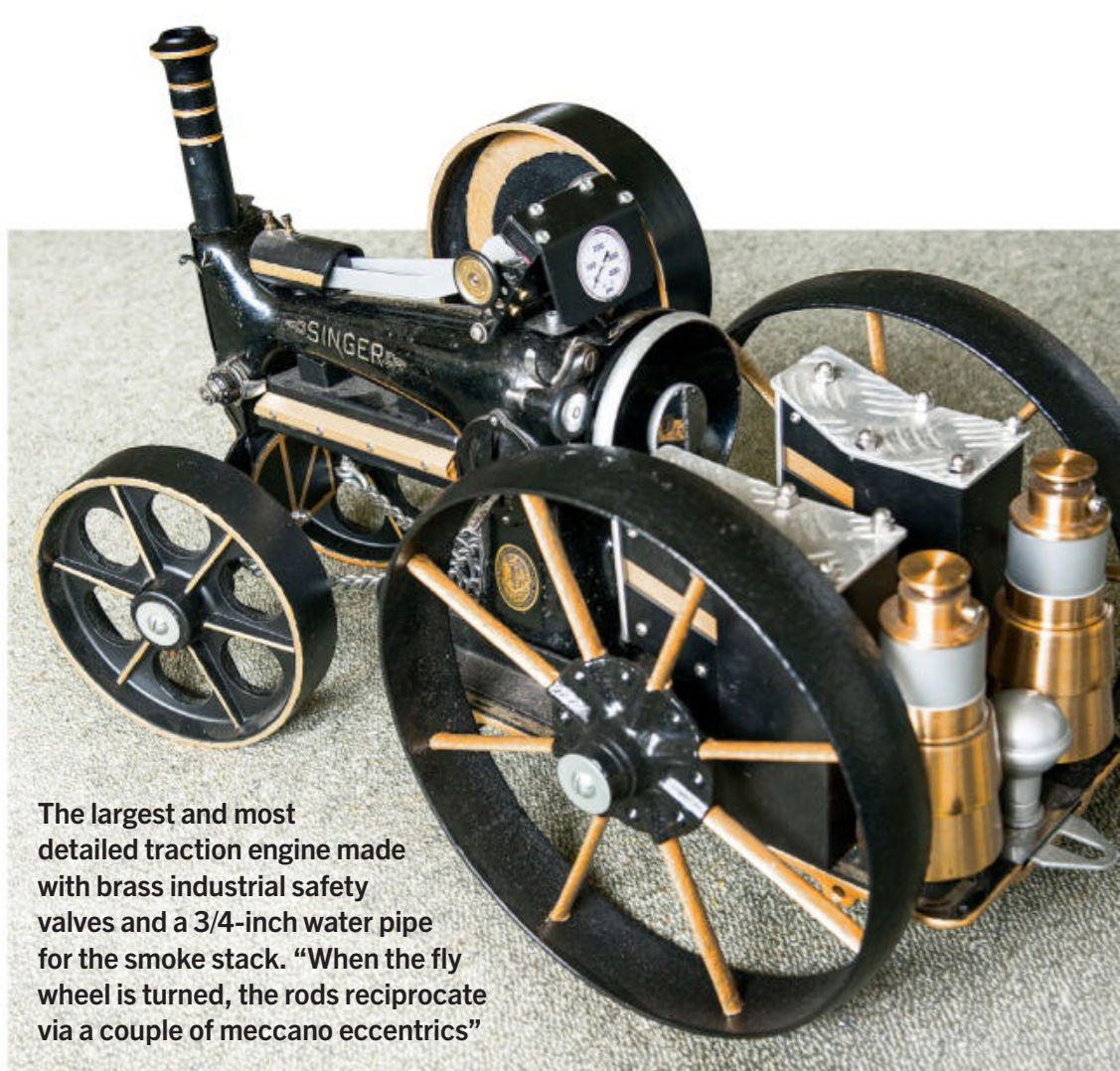
An 1800s hand cranked 'New Home' sewing machine; aluminium extrusion bits for the engine with four old porcelain fence insulators to simulate the cylinders
