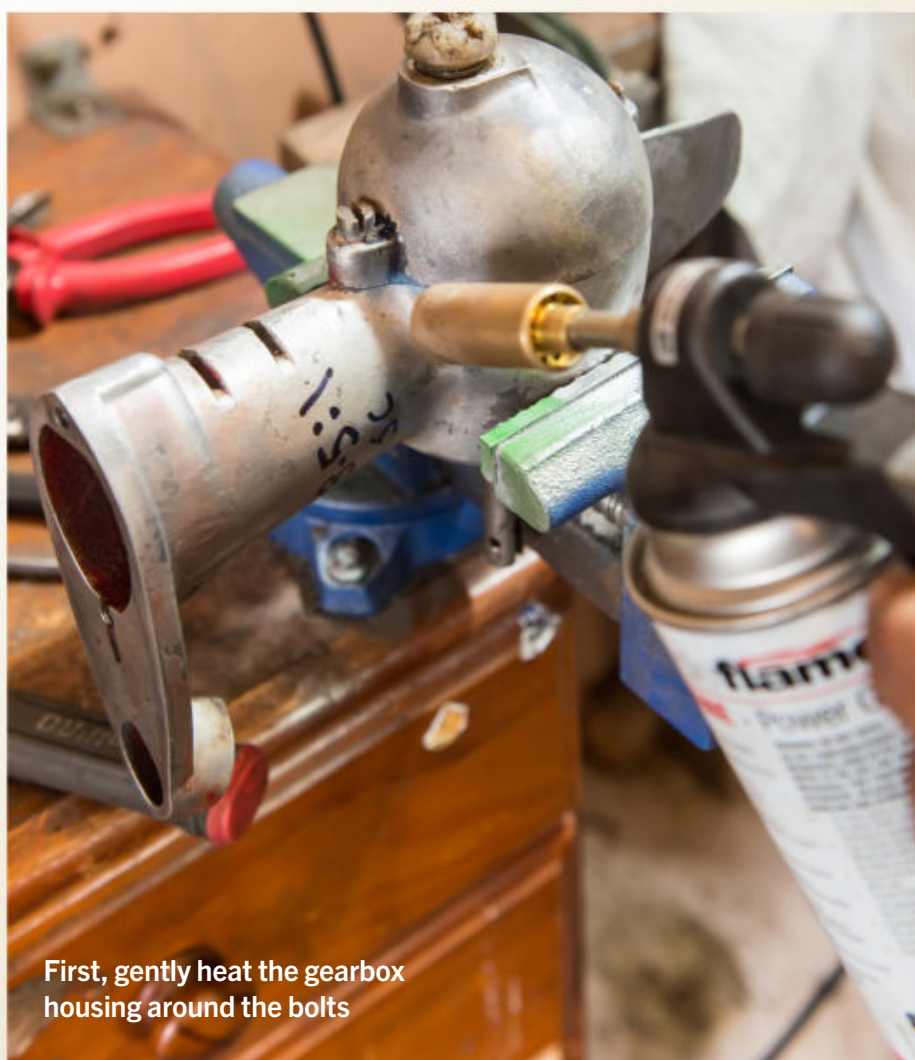
Use vice grips to help loosen the heads before employing a screwdriver — this will help minimise burring if the bolts are still too tight
