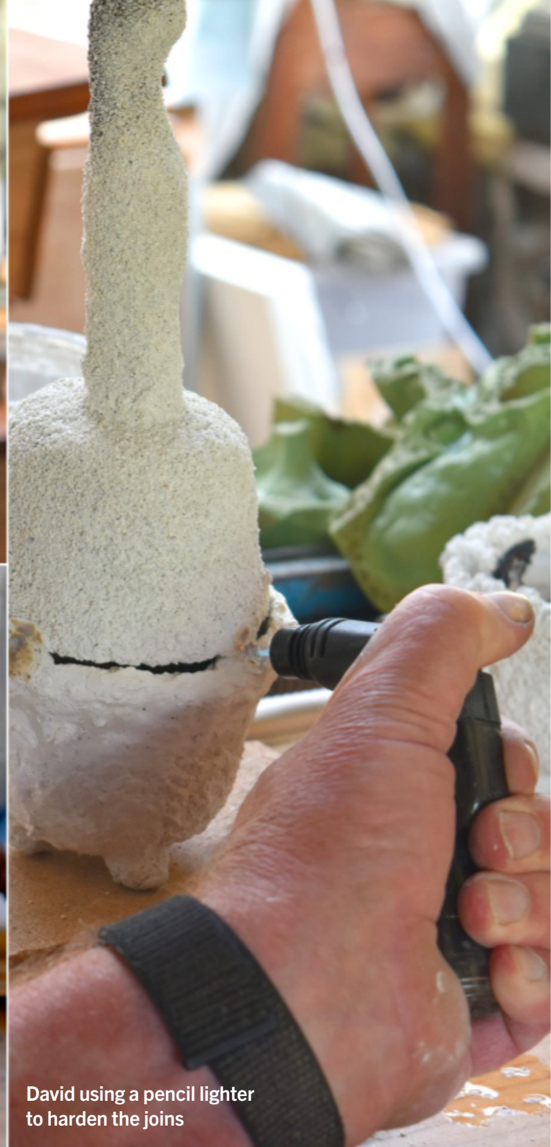
The crucible being joined to the sculpture ceramic shell
