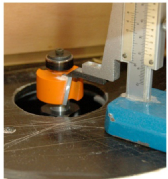
Setting height of bearing guided rebate cutter using Vernier height gauge
