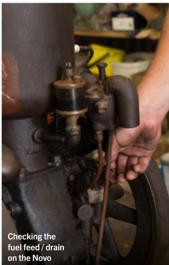
Pinching the oiler for lubrication of the cylinder before start up
