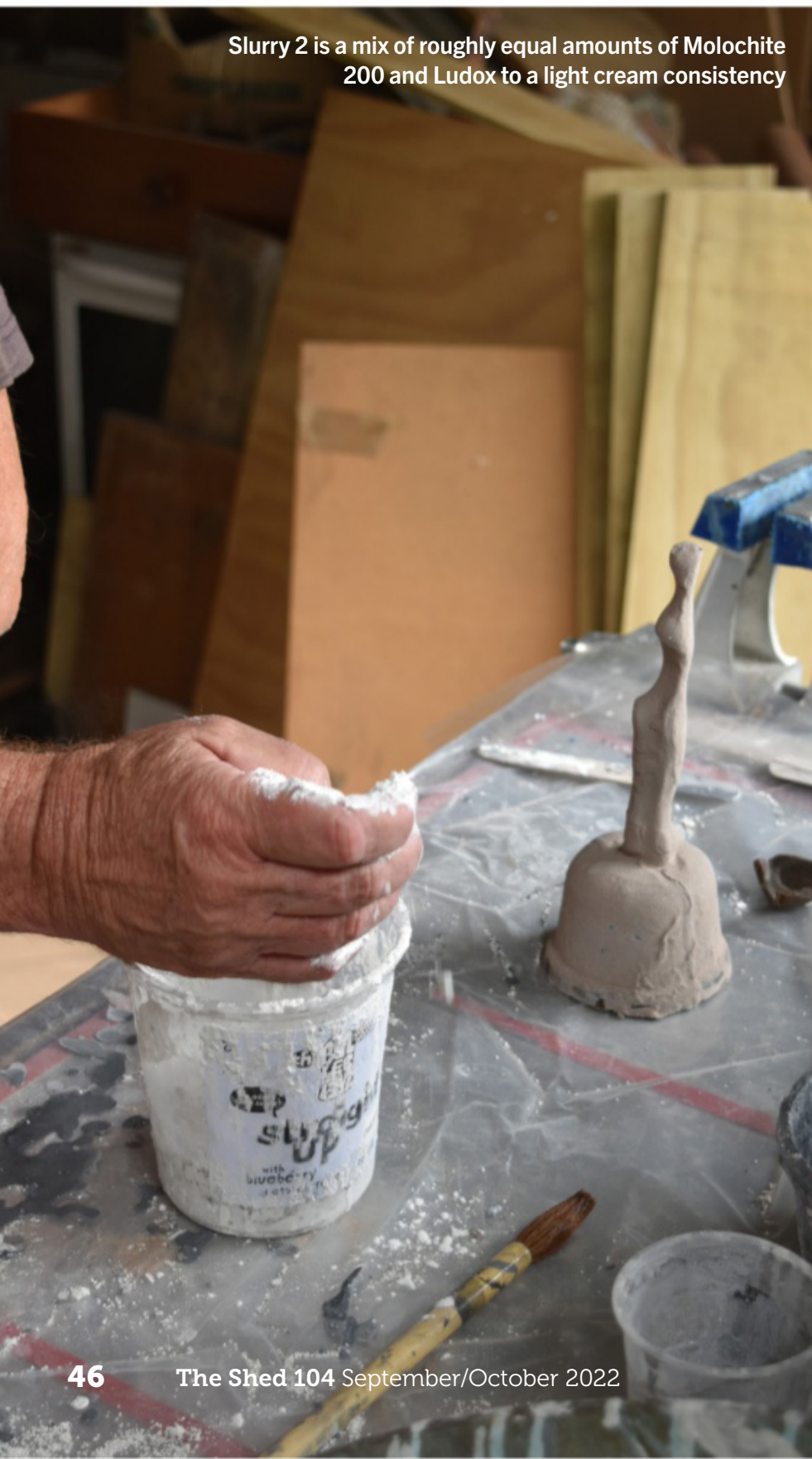
Doing a consistency and stickability test run of slurry 2
