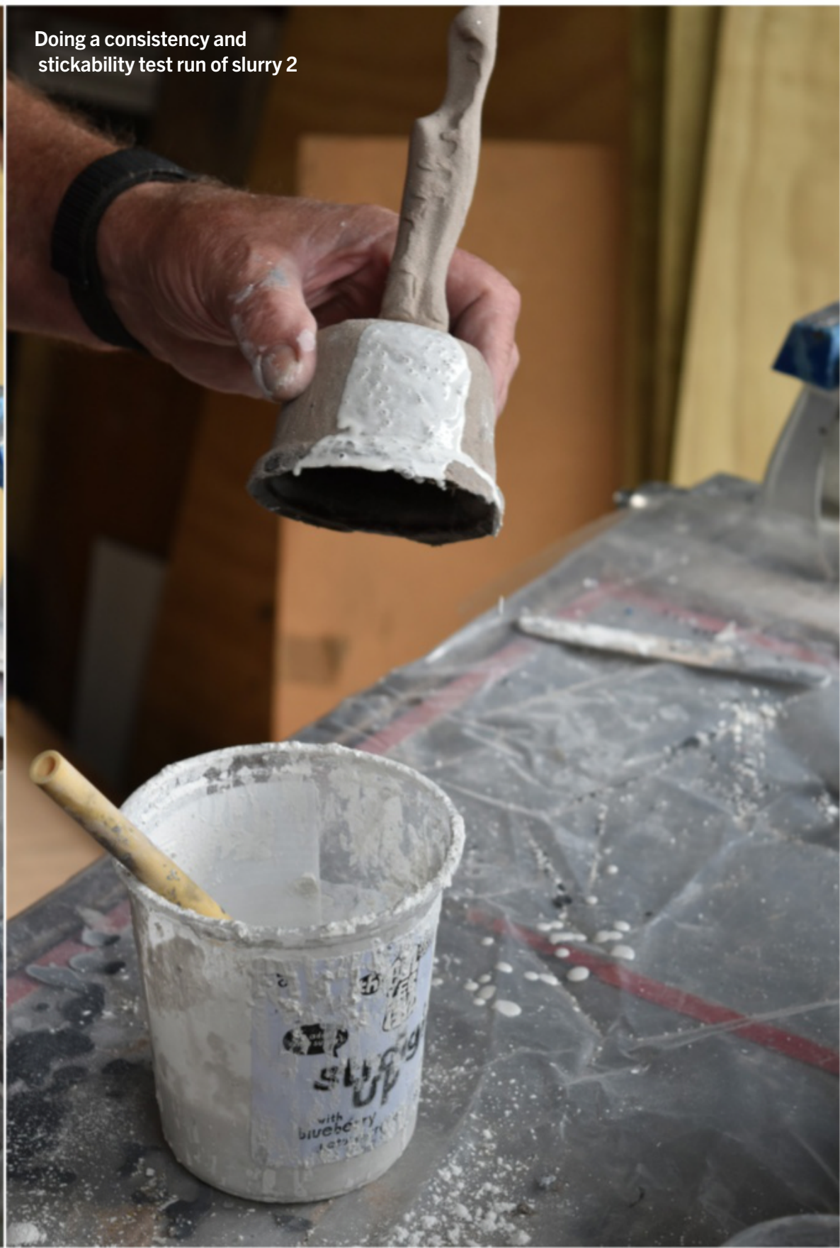
Slurry 2 is a mix of roughly equal amounts of Molochite 200 and Ludox to a light cream consistency
