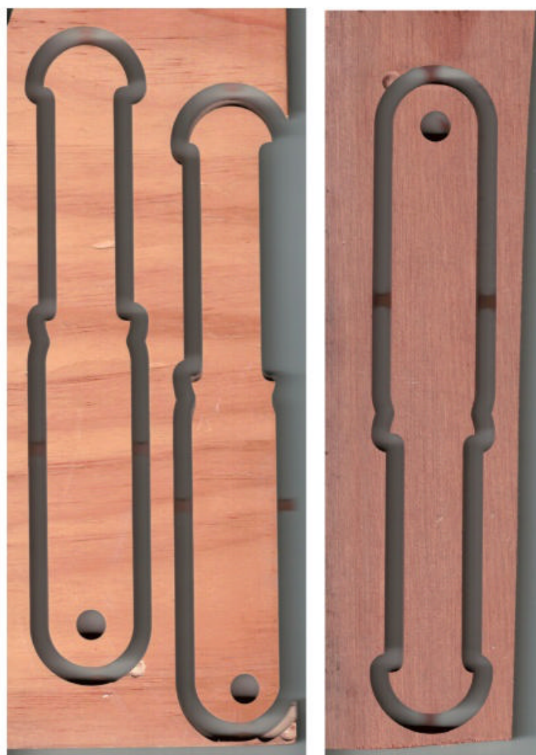
The cheese slicer cut from ply — note the movement at the top of the second one caused by the router being bumped due to the cam and box tensioners being too high
