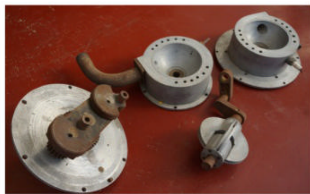
The split spherical chamber (top), linkage mechanism (left), and pistons (lower right) of the rotary motor. Not bad thinking for 1949
