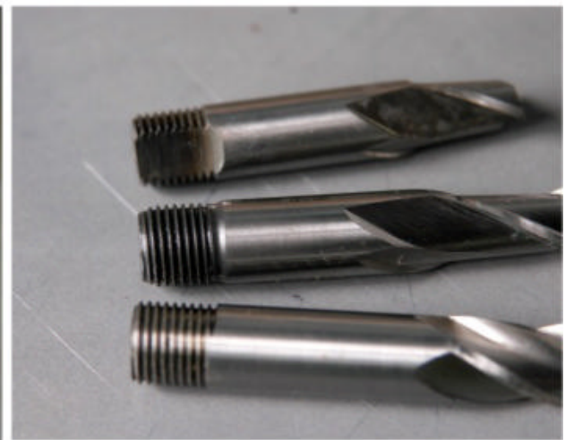
Cutters (from top), with threaded shank ground flat for grub screw, slot drill (two flutes), and end mill (three flutes)
