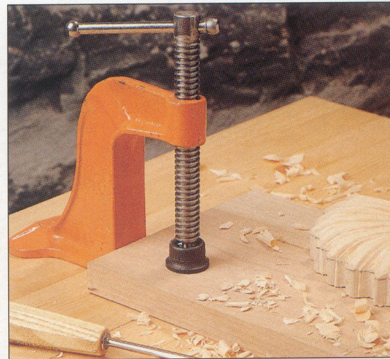
This hold-down clamp fits into a workbench recess originally intended for a bench dog.
