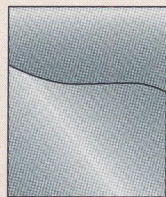
Uneven bevel Makes the chisel difficult to control and produces uneven cuts; caused by sharpening the bevel in some areas more than others
