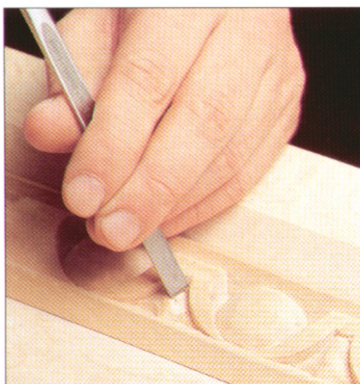
A gouge carves the sloping contours of the dart in a length of egg-and-dart molding. A narrow tool with a shallow sweep, or curvature, provides the most precise cut.
