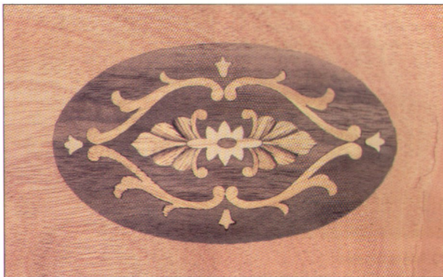
A marquetry inlay, formed from a pattern of dyed wood set in a veneer, adorns a mahogany tabletop. The recess into which the inlay is set was cut with a template-guided router.
