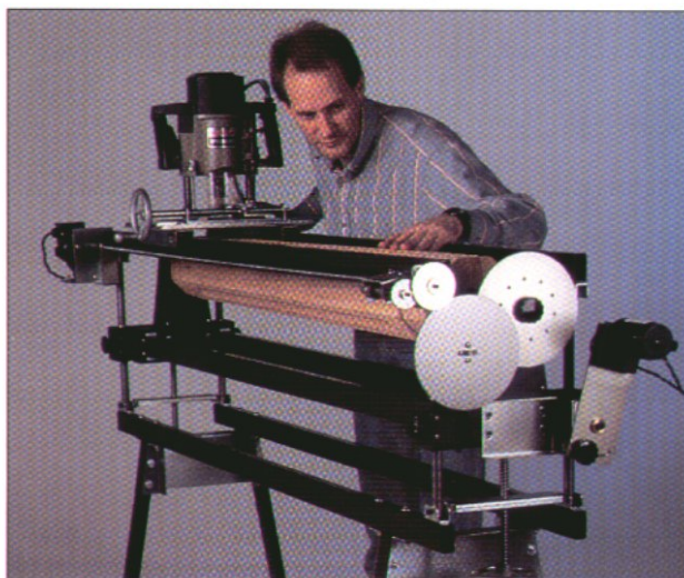
The commercial milling machine shown above transforms the router into a carving tool. Much like a lathe, the machine secures up to three workpieces between centers. Fixed to a metal plate, a router can then be fed along the bed of the machine by hand or with a motor drive. The router can also be left stationary while the crank is turned at the other end of the machine, rotating the workpiece into the bit.
