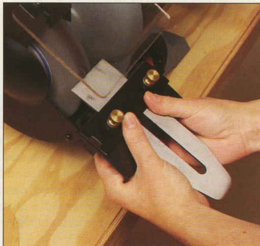
The nicked cutting edge of a plane blade is squared on a bench grinder. Clamping the blade in a commercial grinding jig keeps the end of the blade perpendicular to the grinder's abrasive wheel.
