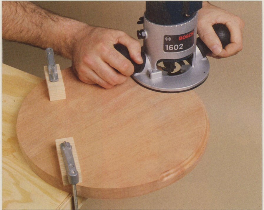
An edge-forming bit etches a decorative profile on the circumference of a table top. The cutter's ball-bearing pilot rides along the stock to keep the cut at a uniform depth.
