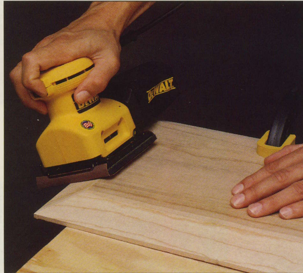
Combining the compactness of a sanding block with the efficiency of a power sander, the orbital palm sander quickly smooths the beveled edges of a raised panel.
