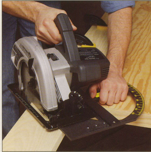
Riding along the edge of a commercial jig, a circular saw can make a miter cut at a precise angle. The jig ensures that the blade keeps to the intended cutting path.
