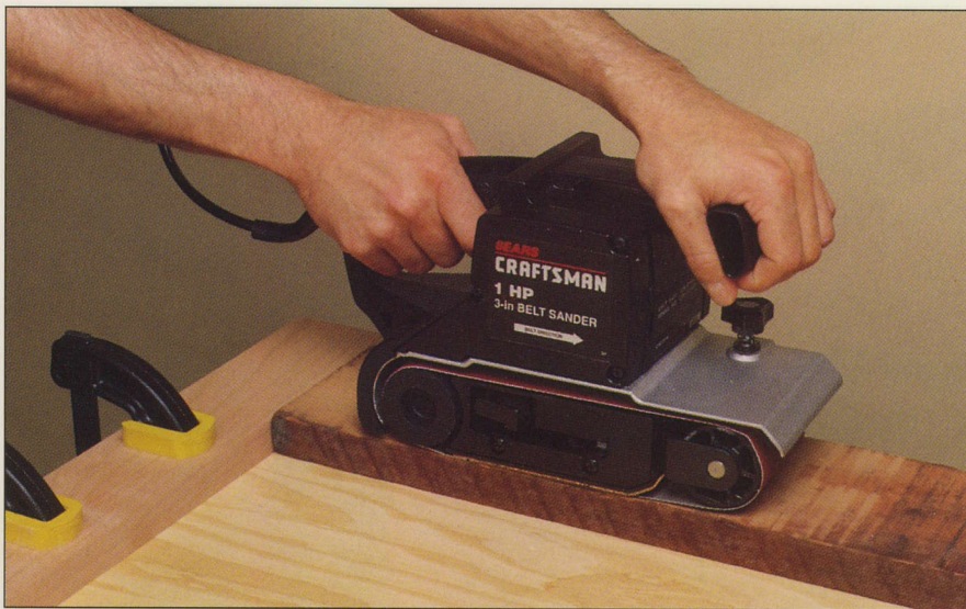
For removing stock, no tool is as effective as a belt sander. Here, it smooths the surface of a rough mahogany board.
