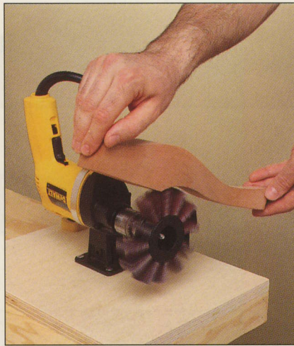
Mounted in a stand and fitted with a flap sander, an electric drill becomes a stationary sander, ideal for smoothing the contours of a cabriole leg.
