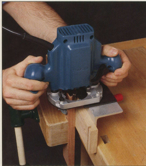
A router can fashion more joints than any other portable power tool. Here, one is used to shape a tenon at the end of a board, aided by a mortise-and-tenon jig.
