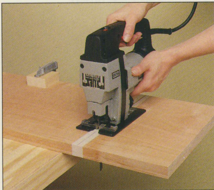
A piece of masking tape applied along the cutting line will reduce splintering while you are ripping or crosscutting.
