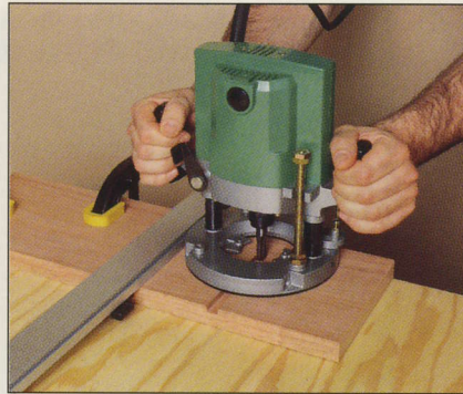
A grooving bit carves a dado in a board. Riding the router base plate along an edge guide produces a cut perpendicular to the board edges.
