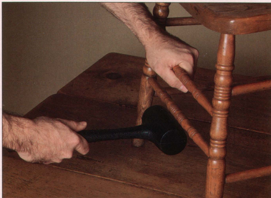
A dead-blow hammer strikes a chair leg to separate it from the leg rails. The metal shot in the head absorbs the blow, focusing the impact on the leg and preventing the hammer from rebounding.
