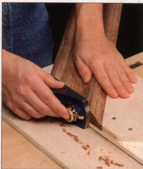
A shooting board holds the mitered end of a piece of molding square to the sole of a block plane. Such shop-made jigs extend the versatility of hand planes, letting them smooth end grain with little risk of tearout.
