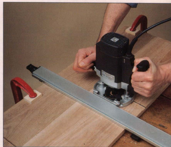
A combination bar clamp and edge guide helps a router cut a dado that is perpendicular to the panel edges.
