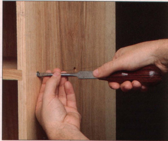
The non-tapered tip of a cabinetmaker's screwdriver enables it to drive a screw into a counterbore hole without marring the sides of the hole.
