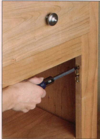
A ratchet screwdriver is ideal for turning screws where space is limited, such as inside the door opening of a cabinet.
