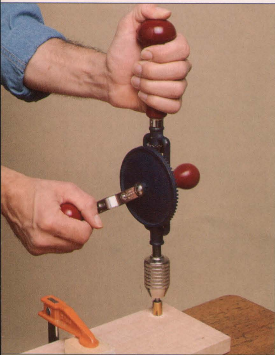
Fitted with a countersink bit, a hand drill widens the mouth of a pilot hole to allow the screw head to be set flush with the surface.
