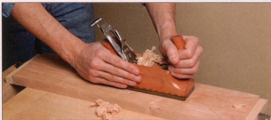
Its blade adjusted to slice off the thinnest of shavings, a wooden smoothing plane evens out the surface of a workpiece.
