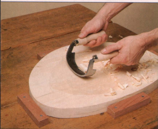
An inshave slices thin shavings from a flat, oval panel, transforming the surface into a chair seat.
