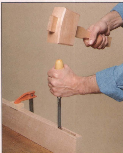
With its 90° angled cutting edge, a corner chisel squares the corners of a mortise cut by a router.
