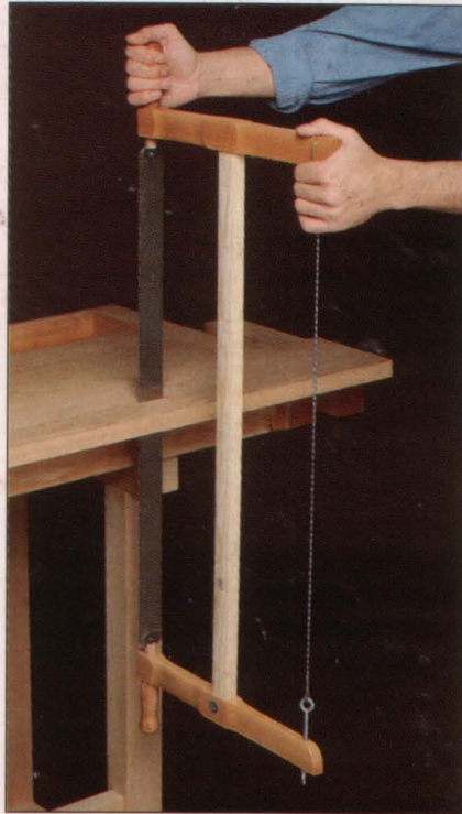
Its blade held taut by a tensioning wire, a frame saw slices through a hardwood board. Because frame saw blades are thinner than most other saw blades, they seldom bind—even in long rip cuts.
