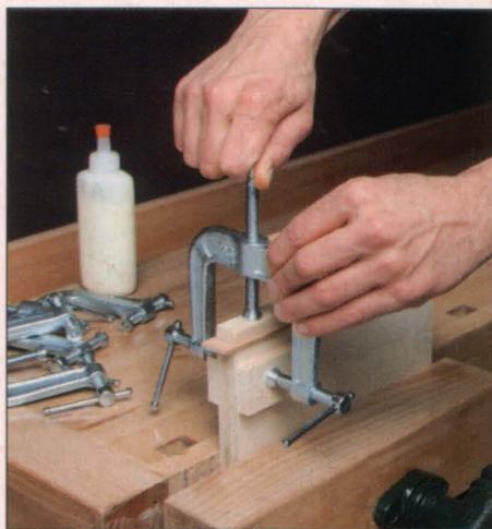
With its two outside screws gripping the opposite faces of a workpiece, the center screw of a three-way C clamp presses a length of edge banding in place during glue up.
