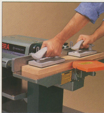
For surfacing a board face, push blocks help to keep stock flat and your hands safe. Lateral pressure keeps the edge against the fence.
