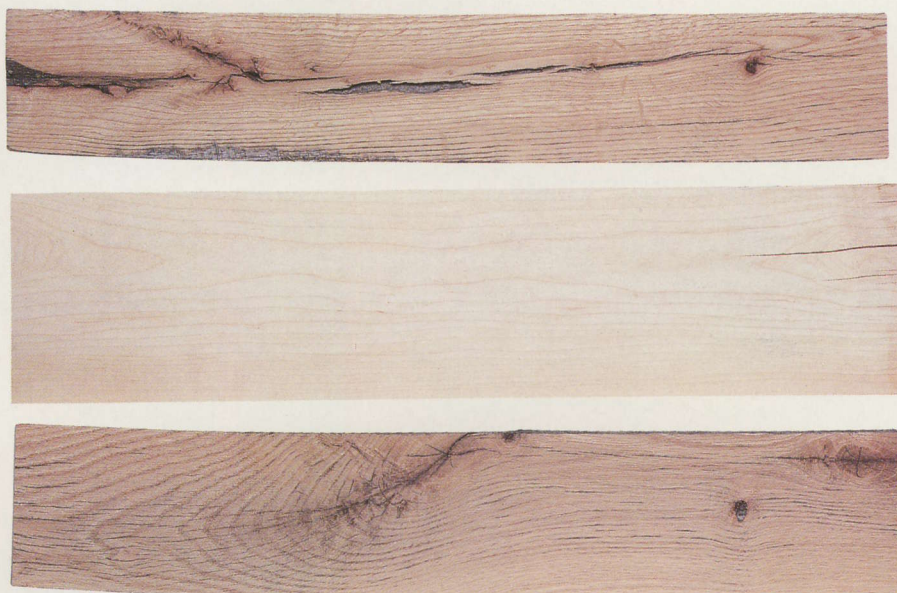
Three pieces of oak with defects: The top board shows splits, the middle piece reveals checks at one end, and the bottom board displays a crook, a loose knot and reaction wood.
