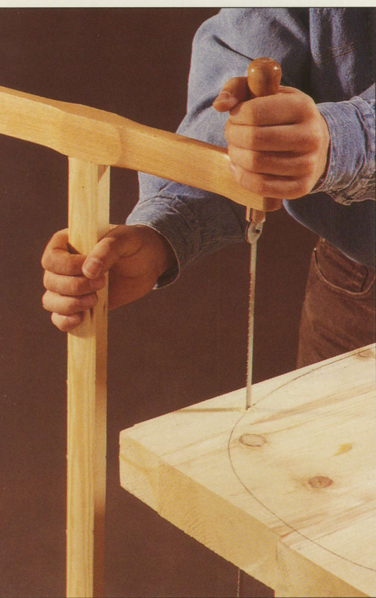
A frame saw cuts a Windsor chair seat blank from a pine plank. The blank will be shaped later with a variety of hand tools. It could also be cut on a band saw.
