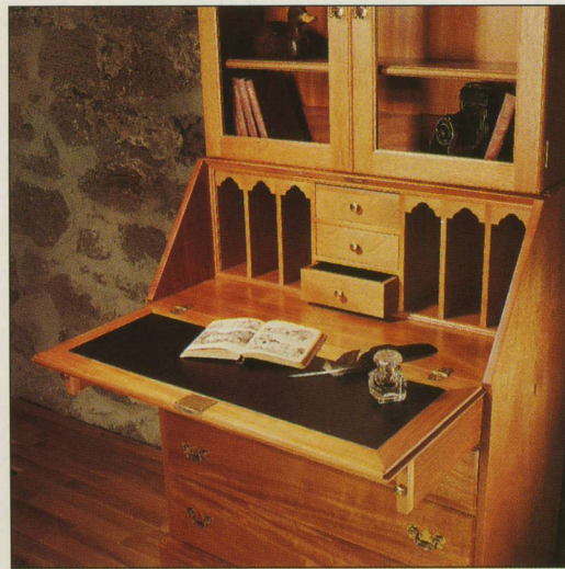
The weight of the fall-front in the secretary shown above is borne by a pair of supports called lopers. In the down position, the front becomes a leather-lined writing surface. The removable pigeonhole unit is set atop the desk unit.
