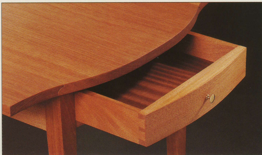
Supported by runners fastened to the side rails, the Pembroke table drawer shown above is assembled with through dovetails. The false front curves to match the profile of the end rail and drawer rails.
