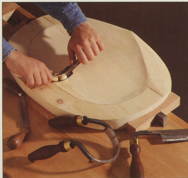
The top of a Windsor chair seat is traditionally sculpted by hand. With shaping tools like the spokeshave, inshave, and drawknife, it is possible to customize the seat for its user.
