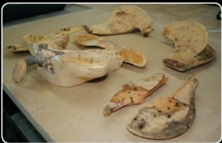
Broken tree as received in a box in seven pieces
