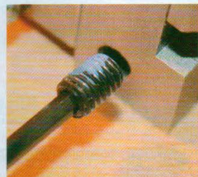
A small dab of Loctite Blue will seat the set screw securely.
