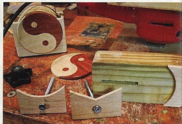
This shopmade jig holds a variety of shaped pieces for surface sanding.
