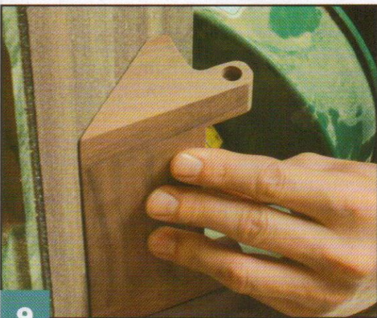
9 Glue and clamp the shovel sides onto the assembly. When dry, sand all sides flush with 220-grit sandpaper, creating bevels in the shovel bottom and back. Round the edges slightly. Use the belt sander.
