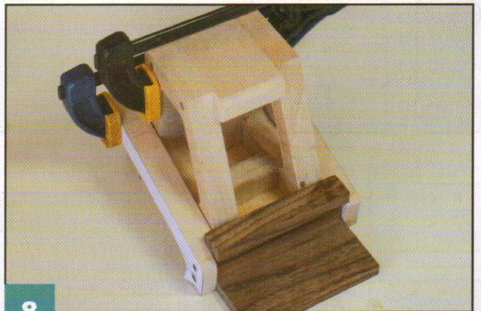
8 Dry fit the arms to the body. Then fit the shovel bottom and back assembly between the arms. Trim the assembly if needed.
