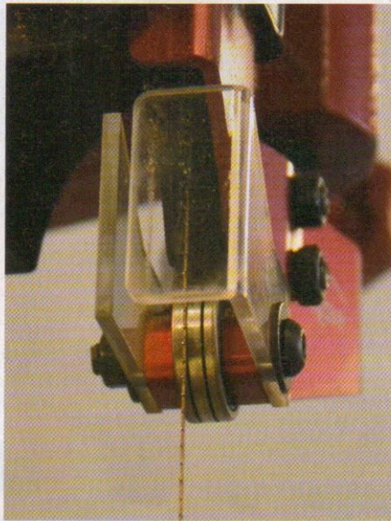
Dual precision-grooved bearings keep the blade aligned in tight turns.
