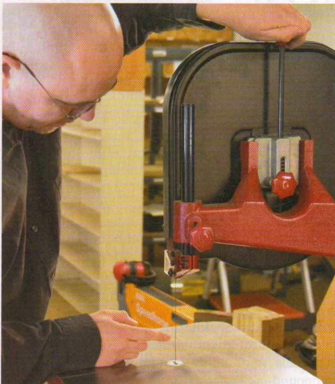
Proper tensioning is important. The blade tension should be set similar to that of a scroll saw—approximately \frac{1}{8} " (3mm) flexion.
