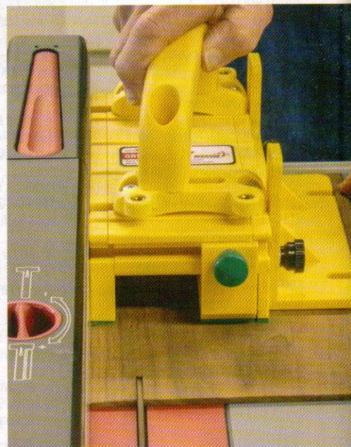
Although push-sticks do an adequate job, the GRR-Ripper tool keeps your hands safely away from the spinning blade.
