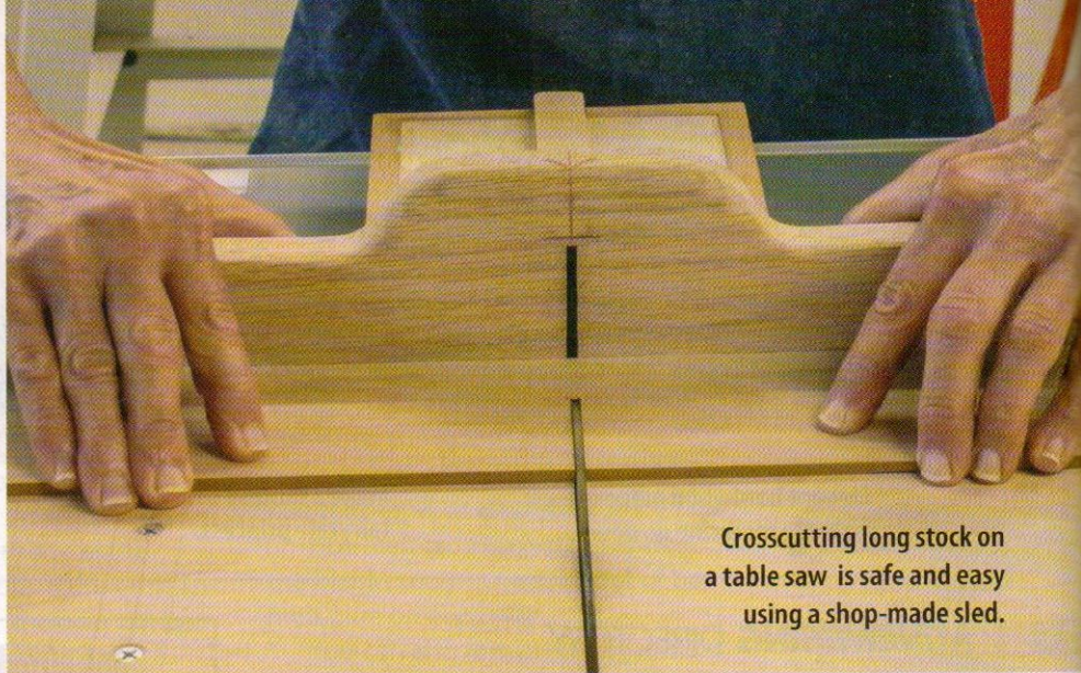
A table saw replaces the cumbersome and time-consuming process of preparing linear cuts on a scroll saw.
