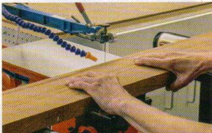
A table saw replaces the cumbersome and time-consuming process of preparing linear cuts on a scroll saw.
