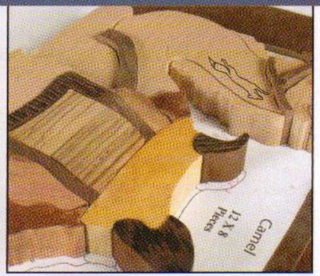
3 Taper the edges of the marked pieces. Use a 100-grit sanding drum. Use pliers to hold smaller pieces, and wear finger protection as you sand. In general, mark the level and sand down to the line, keeping the line side up and in sight whenever possible. Switch to a 220-grit drum to soften the edges and remove scratches from the coarser grit drum.
