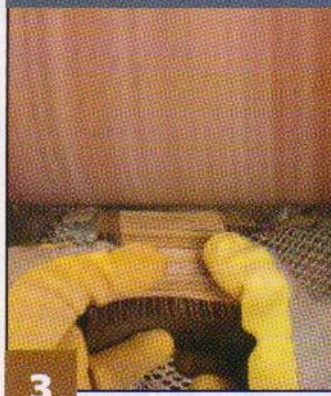
3 Taper the edges of the marked pieces. Use a 100-grit sanding drum. Use pliers to hold smaller pieces, and wear finger protection as you sand. In general, mark the level and sand down to the line, keeping the line side up and in sight whenever possible. Switch to a 220-grit drum to soften the edges and remove scratches from the coarser grit drum.
