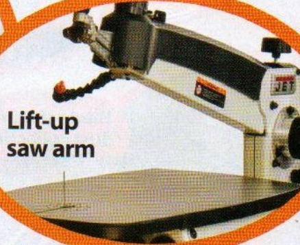
Controls at top front of saw arm
