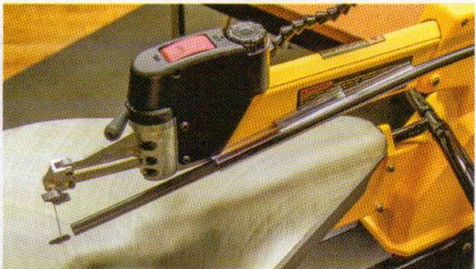
The flexible vacuum nozzle and magnetic mount let you position the dust collector where you need it.
