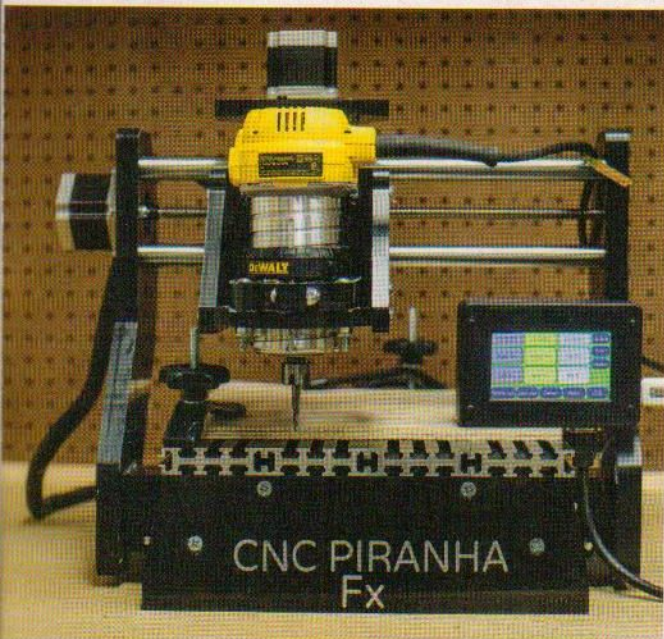
The Piranha FX combines a CNC router, a laser engraver, and a 3-D printer in one compact desktop unit.
