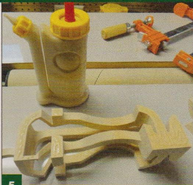
5 Glue the quarters to form halves. Glue and clamp two sets of quarters together to create two halves. Remove any glue squeeze-out with a damp rag. Cover the areas that will be glued together with tape and apply finish to the inside of the lantern. I use spray lacquer.
