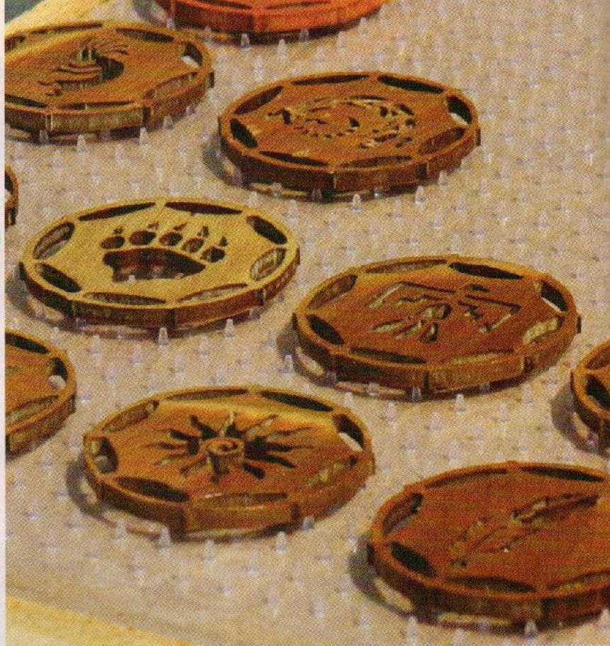
Carpet protectors provide a uniform raised surface for drying painted or finished projects.
