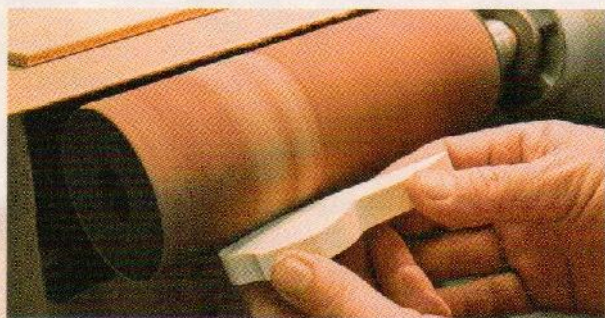
The Flex Drum sander is soft on the end, which allows you to carve rough detail using the sander.
