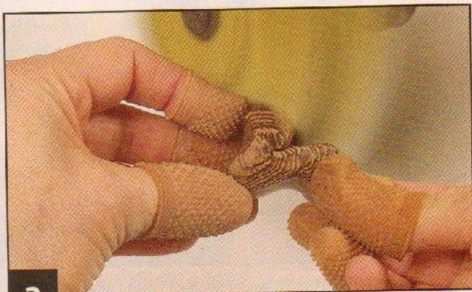
3 Buff the pieces. Smooth each of the pieces with a mop sander. The mop sander removes the scratches from the shaping process and produces a smooth surface.
