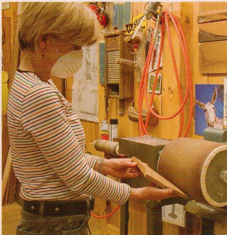
Judy uses an 8"-diameter drum with a 100-grit sanding sleeve to remove wood quickly.
