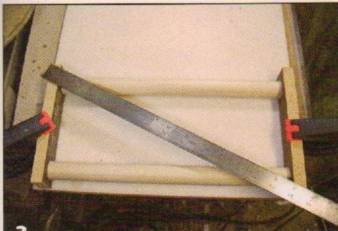
3 Glue the dowels in place. Apply glue to the ends of the dowels and insert them into the side supports. Measure the diagonals of the assembly to ensure it is square. Make any necessary adjustments and clamp the supports to the work surface until the glue dries.
