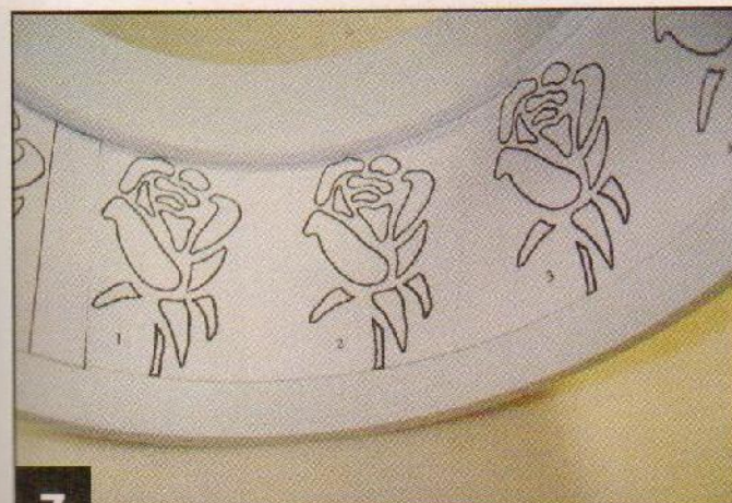
7 Attach the rose pattern to the PVC. Apply spray adhesive to the back of the pattern. Position the pattern inside the coupling with the feet aligned with the uncut edge.
