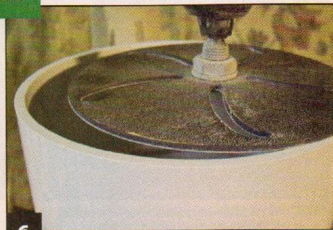
6 Sand the cut edge. We use a SeeSander, but you could use a belt sander or disc sander. Even up the cut edge leaving a smooth surface. The cut end of the coupling will become the top.
