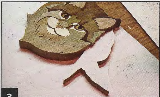
3 Cut the right side and right rear leg. The grain direction runs the same way for these two pieces, so you can cut both of them together and then cut the individual pieces apart.
