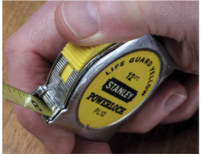
Stanley's iconic PowerLock in Life Guard Yellow with thumb-operated lock (above) and the patent drawing of William Bang's 1864 tape measure with 'compound spring-click stock' (below)
