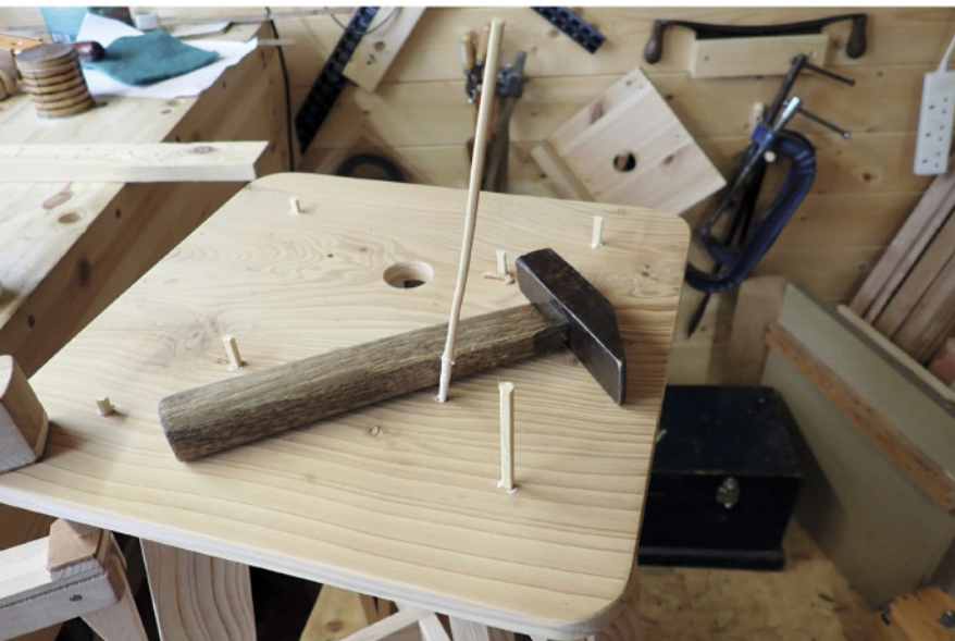
A vintage German fine saw (right) with an offset blade, does an excellent job of trimming back those stubs. Hold the seat tightly clamped down (above) when inserting nails to avoid a gap between the bearers and the seat. A square peg in a round hole (right). The wood fibres are visibly distorted by the corners of the bamboo nail, but there is no splitting, just a very tight fit. And there is still space for some glue to help keep all the parts together
