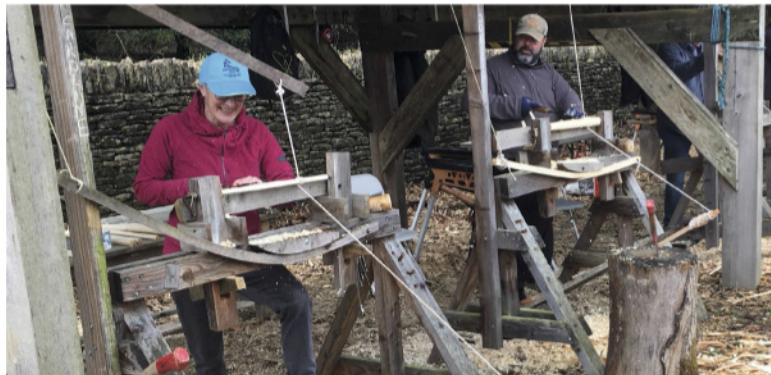
Caroline and Jon banter and smile at the pole-lathe. This is Day Three, with Caroline turning a spindle, with the wood about to wobble. She may have to run her hand round the spinning blank to keep it calm
