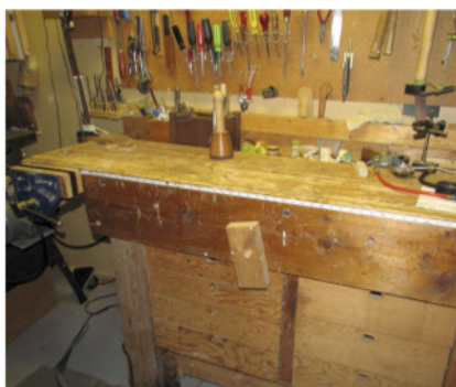
You need just a few holes on the apron to work with Bob's bench jack (Pic.4, above left). Rotate the 2x4 block to get to the desired support height for the board (Pic.5, above right)
