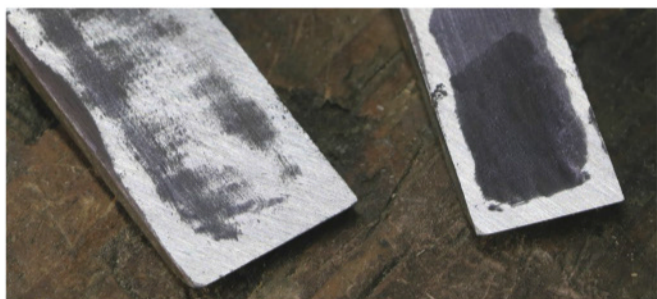
Two chisels first ground with a rotary tool (Fig.7, above). The back has been marked with a marker pen and honed with a flat 120 grit diamond stone. The hollow is shown by darker areas. The larger chisel needs more hollowing and flattening through honing. The smaller one needs more honing as the left-hand corner has no scratch marks
