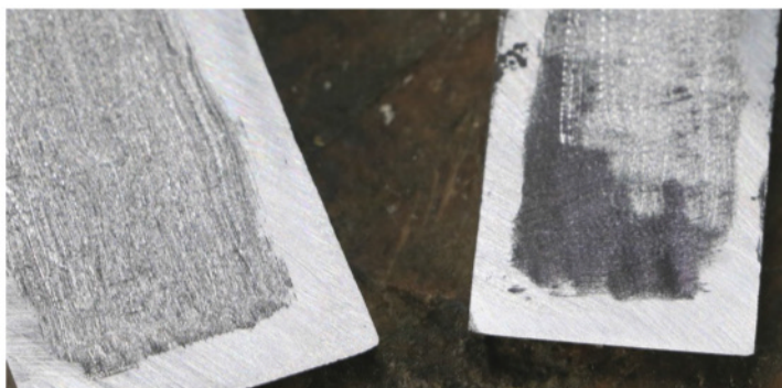
The finished hollowing and flattening on a 120 grit stone (Pic.8, above). They are now ready to be abraded on a 400, 1000 and finer polishing stone, 3000 and/or 6000 grit
