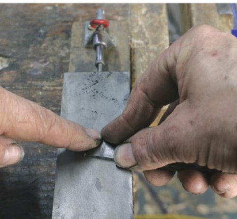
Holding the chisel with both hands near the cutting edge for accurate flattening (Pic.4, left). Bright areas on both chisels (Pic.5 above) are scratch marks from 120 grit diamond stone (Pic.6, right)
