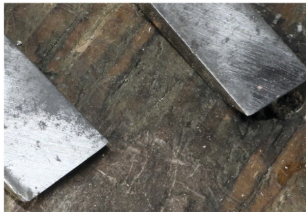
Holding the chisel with both hands near the cutting edge for accurate flattening (Pic.4, left). Bright areas on both chisels (Pic.5 above) are scratch marks from 120 grit diamond stone (Pic.6, right)
