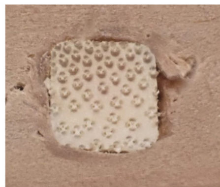
A vintage German fine saw (right) with an offset blade, does an excellent job of trimming back those stubs. Hold the seat tightly clamped down (above) when inserting nails to avoid a gap between the bearers and the seat. A square peg in a round hole (right). The wood fibres are visibly distorted by the corners of the bamboo nail, but there is no splitting, just a very tight fit. And there is still space for some glue to help keep all the parts together
