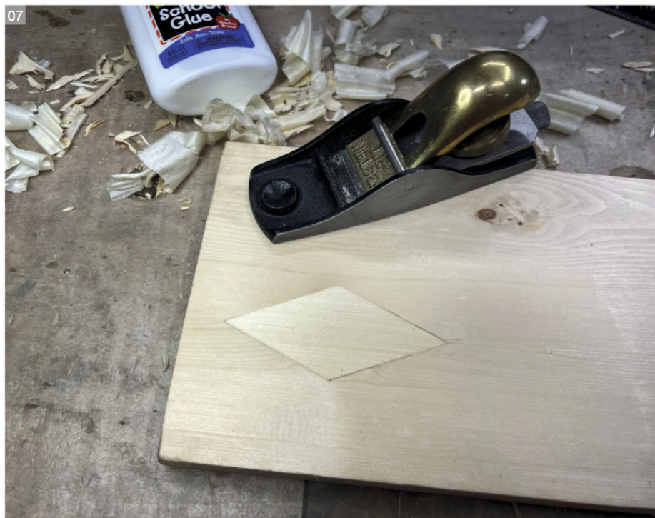
A block plane can be used to level the patch (above), so long as there's a fresh edge. Drawing the patch (left) to cover the damaged spot
