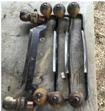
When Paul found an old French drawknife (left, above) he designed three of his own, with the distinctive round handles, and had them made as a set (on the right, above)
