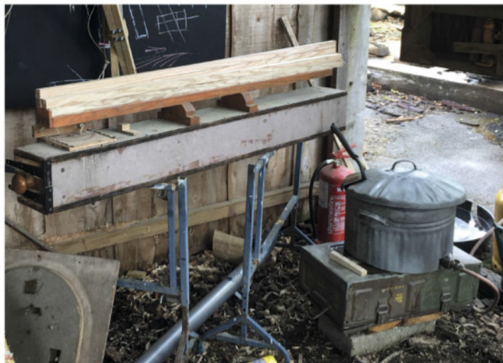
Bending the comb is done in a former, with a hand-powered piston jack
