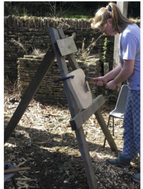
India (above) using an easel for removing waste with an adze. Then you will use a travisher or hollowing tool (right) or a scorp (below)
