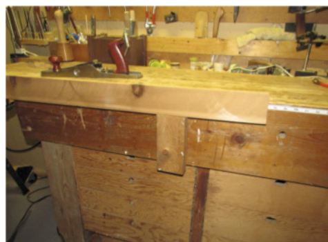
You need just a few holes on the apron to work with Bob's bench jack (Pic.4, above left). Rotate the 2x4 block to get to the desired support height for the board (Pic.5, above right)
