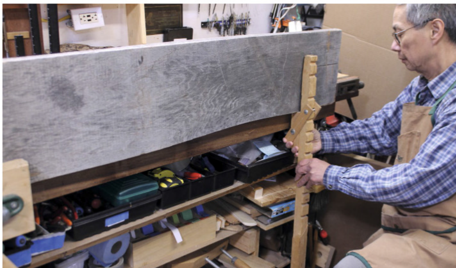
A board jack (Pic.1, above), aka a bench slave, is used to keep a board from sliding or dropping
