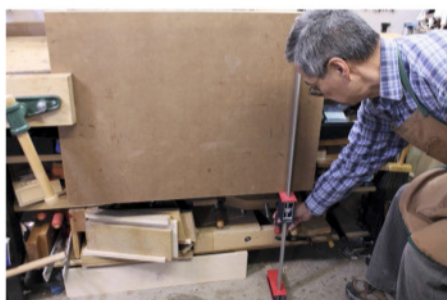
Any parallel clamp with a spreader function can work as a board jack (Pic.3, above)
