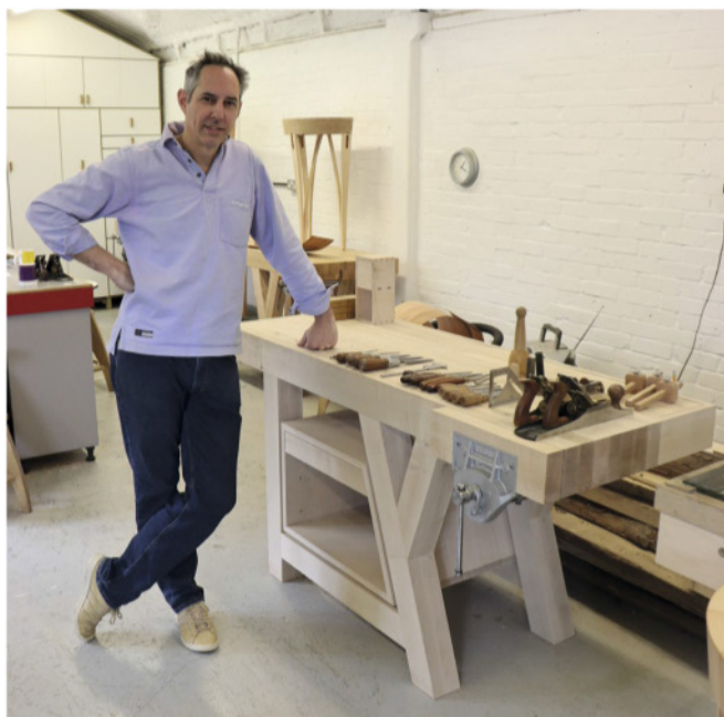
Ian Parker designed and made the unusual bench Quercus has purchased, attracted by the over-hanging end, Y-shaped underframe and right-handed bench vice (left). On that point we've tested where to drill our old bench to fit a pattern-makers vice (above), as debated in a blog by @lostartpress
