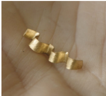
Macro photo (left) showing the ideal wedge-shaped cross section that results from the hammering. The finished rivet (above) ready to hammer into the bowl. Pliers being used (right) to bend the hammered strip into the wavy Cairns Bowl shape. The three stages of zig-zag rivet manufacture (below). The curved strip (right below), hammered and straightened (middle below) and bent (left below)
