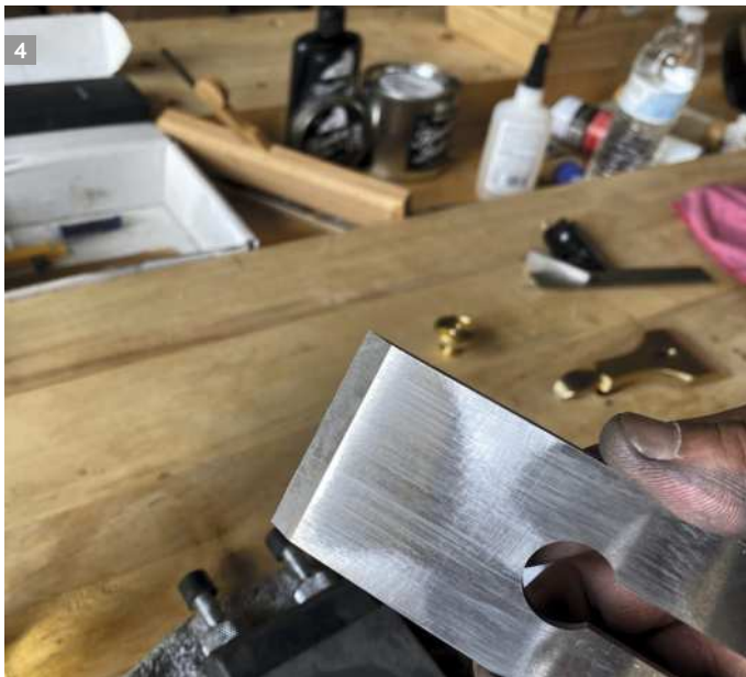
Curtiss goes through the grits of lapping compound (above) the same as going through grits on stones. He also laps the top of the blade (below)
