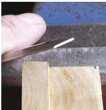
Bill Carter's iconic Blunt Chisel Tip, which starts with the bevel ground off the end of a paring chisel (left) to make it flat across the end (above) for working in any direction, into any tight spot, on any wood and along, across or against the grain (right)
