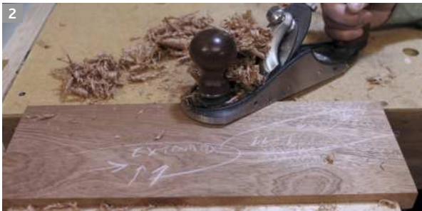
2 Broken shavings mean the board isn't flat (above). You can alter the shape of shavings by skewing a cut (right) or cupping the mouth to control how the shaving exits the plane
