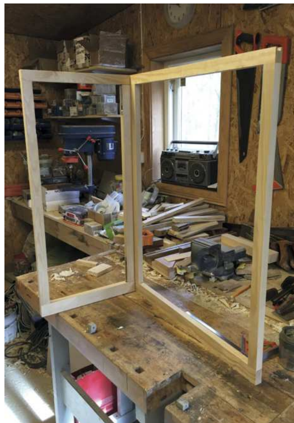
The face-frame assembly (above). There is a detachable upright on the right of the small cupboard face frame so that a gas bottle can be slid into the cabinet as it is a tight fit
