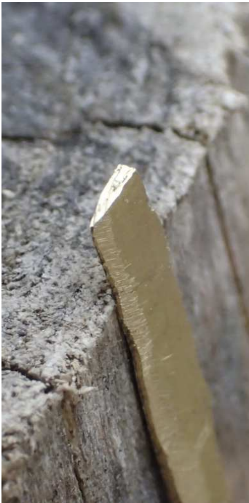
Macro photo (left) showing the ideal wedge-shaped cross section that results from the hammering. The finished rivet (above) ready to hammer into the bowl. Pliers being used (right) to bend the hammered strip into the wavy Cairns Bowl shape. The three stages of zig-zag rivet manufacture (below). The curved strip (right below), hammered and straightened (middle below) and bent (left below)
