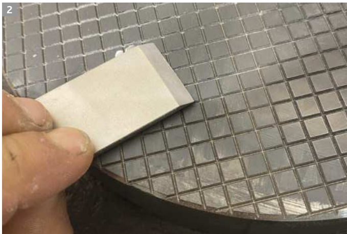
Curtiss goes through the grits of lapping compound (above) the same as going through grits on stones. He also laps the top of the blade (below)
