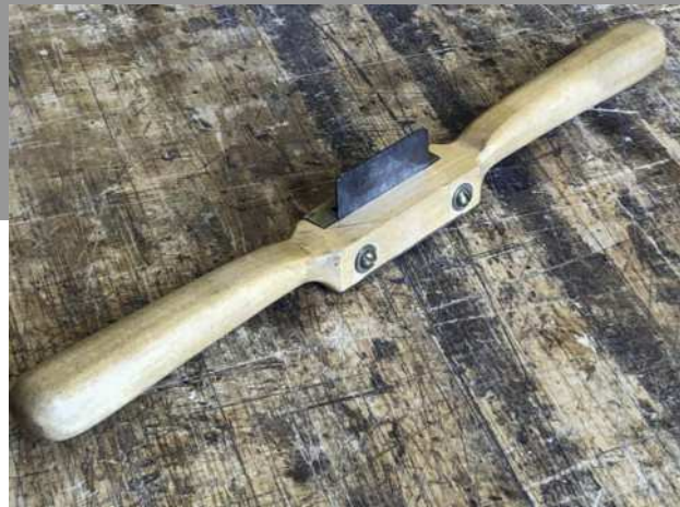
Ball-joint scrapers like Stanley's No.283 (left) were also made by other manufacturers. The chairmaker's scraper (above) is also known as a scraper shave or a chair devil
