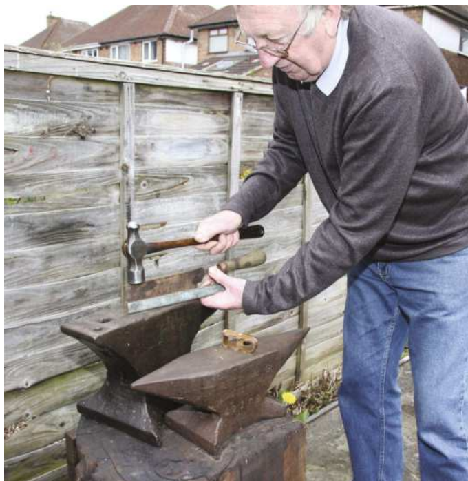
The bodies of Bill's planes are often made from the backs of old tenon saws, which he splits apart and then saws in half
