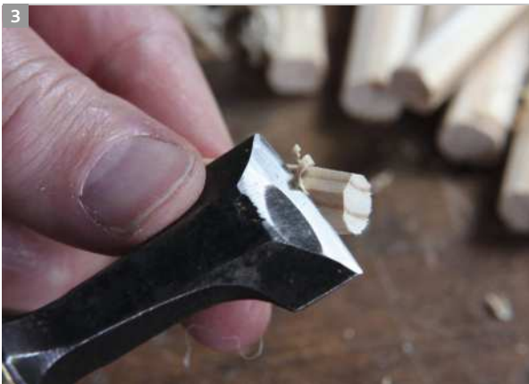
Pointing an end (above) to ease knocking the blank through the gate-hook dowel plate. A lump hammer knocks the blank through the hole (below)
