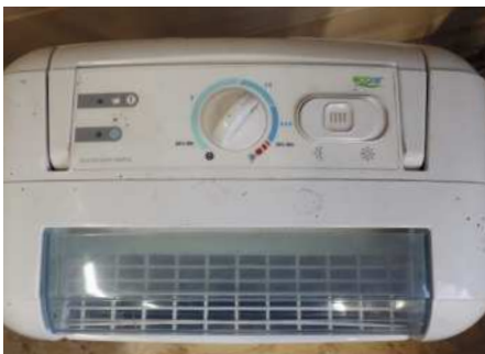
The dehumidifier close up (above). The power setting is about half way on the dial. The high or low power slider is to low. This was the initial guess, and Henrie never felt he should change these settings
