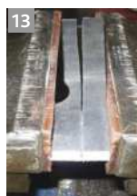
The little plane ready for lapping on the plate (left). The iron is an old one split into four (above left), then the wedge is cut and filed to shape (above right)
