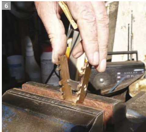
Fitting the bridge into the bent body (left), and the body is tightened with a washer spacer and again can be peined on an anvil (above)
