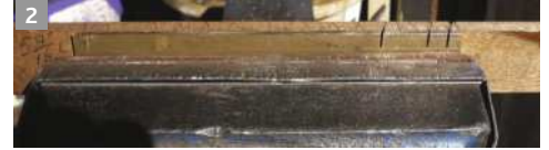
Using a wooden template (based on earlier planes), Bill guides a saw to cut the tails on the body (above). It takes a lot of hacksawing, knocking out of waste with a hammer, some filing and drilling for the body (below) to be ready for bending
