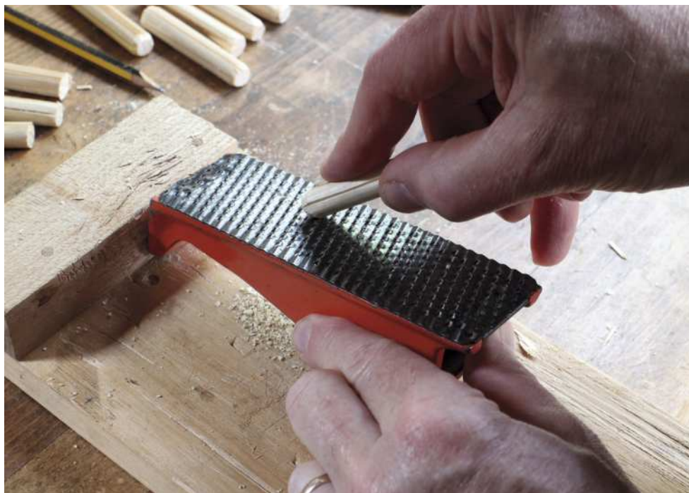
Bevelling ends of dowels on an inverted Surform block plane (above) and a blunted wood screw grips the dowel in the grooving jig (right)
