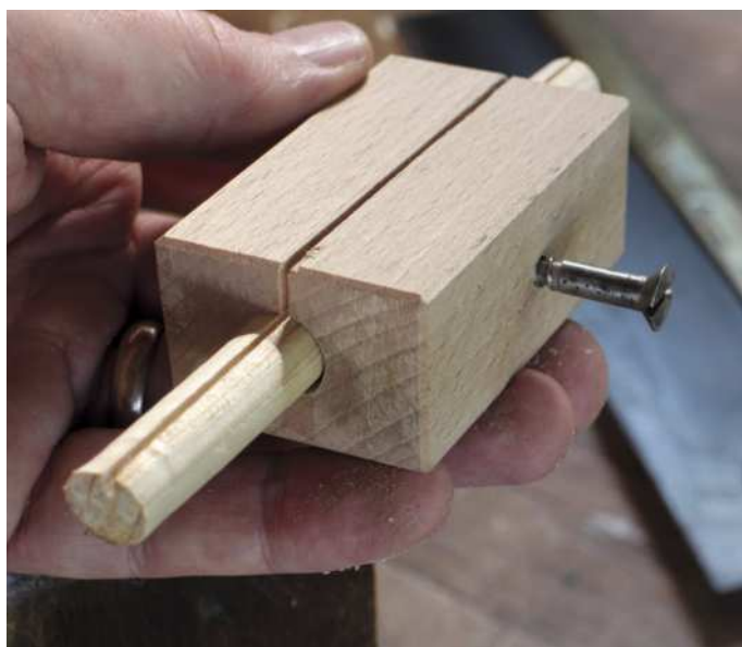
Bevelling ends of dowels on an inverted Surform block plane (above) and a blunted wood screw grips the dowel in the grooving jig (right)
