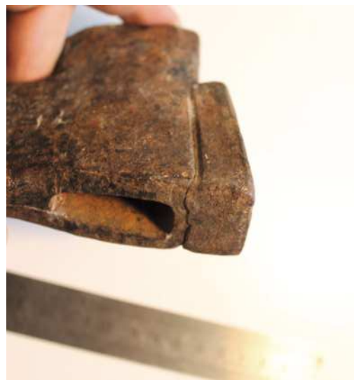
One of Per Nordlöv's earlier stamps (left): "P N L \ Garanti. In English Per Nordlöv, Warranty. The original handle (above) had an overall pleasant shape, but it had split and had been repaired with a nail. The forging line (right) shows where the poll has been added to the body
