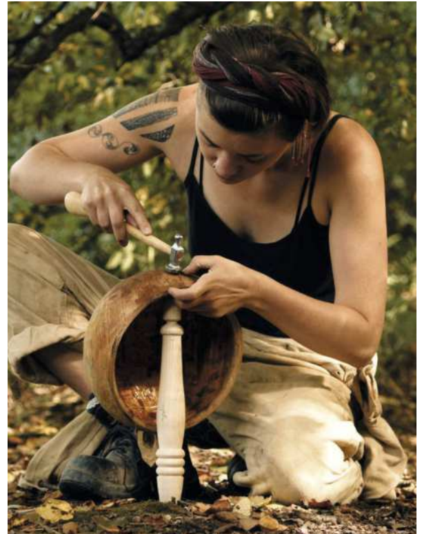
The wavy rivet (or corrugated fastener, above left) being hammered across a crack in the end-grain of the bowl. The wavy rivets (below left) on the full-size replica of the Cairns Bowl. Viv tapping home one of the rivets home (above) with the crack supported by a turned post
