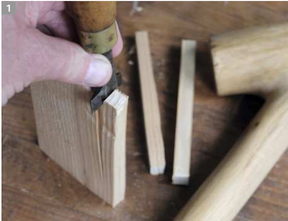
Using a butt chisel to rive squarish dowel blanks from a fir offcut
