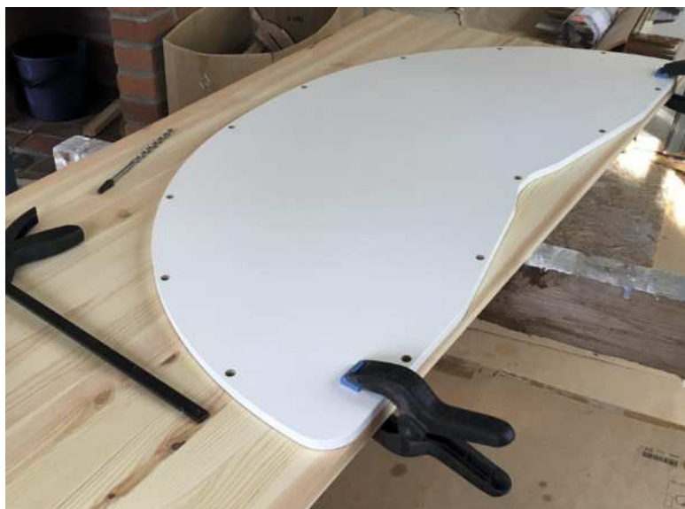
Copying the Ikea shelves onto the shelf material (above) One good thing with the Ikea kit is the the metal hardware also comes with two fibreboard shelves which can be used as templates for your own design.
