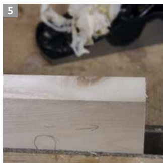
Press the shavings tight to the mouth (left) to control tear-out, and the trick works great for small sections of difficult grain (above). The last shaving is a record of the last blade setting
