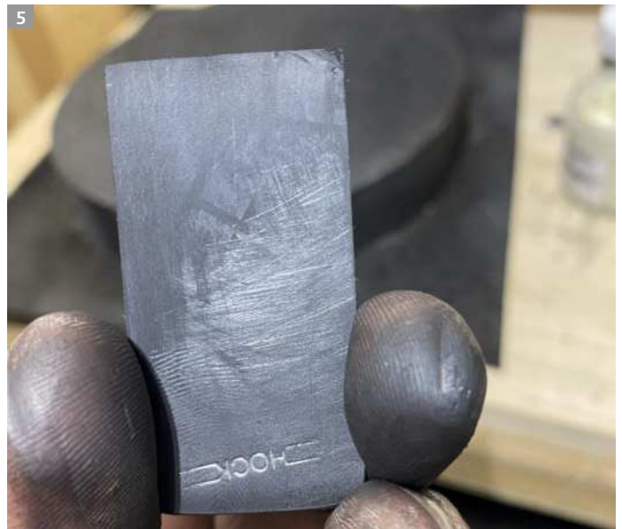
"There is," Curtiss promises, "curvature (above) to the blade." The lapping compound makes it easy to see your flattening process (below)
