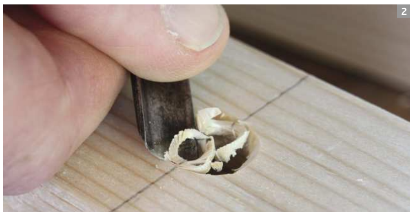
Chamfering a dowel hole (above) to accommodate the glue squeezed out. Dowels in place (below) and the joint ready for assembly
