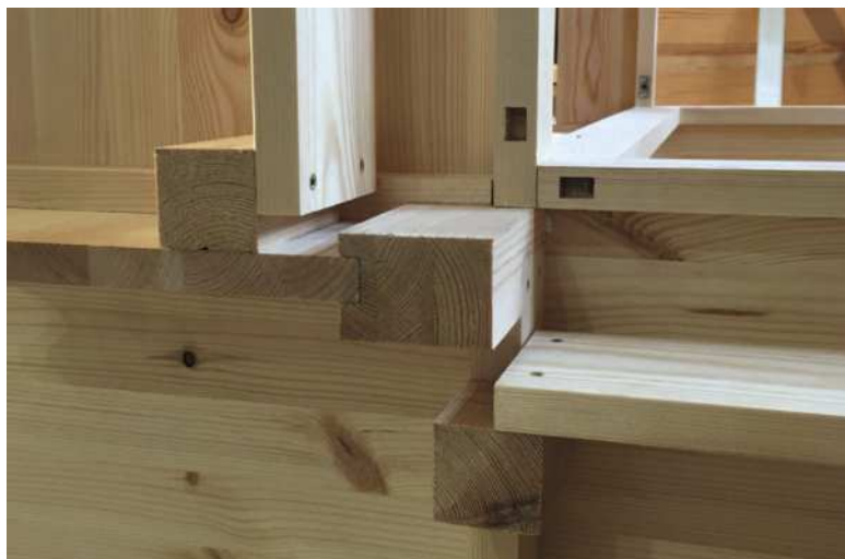
The finished carcass (above) and a view from underneath (below). The two mortise holes in the face-frame are where the legs will be attached
