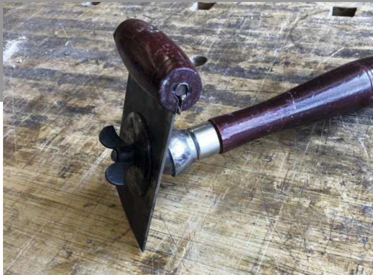
Ball-joint scrapers like Stanley's No.283 (left) were also made by other manufacturers. The chairmaker's scraper (above) is also known as a scraper shave or a chair devil
