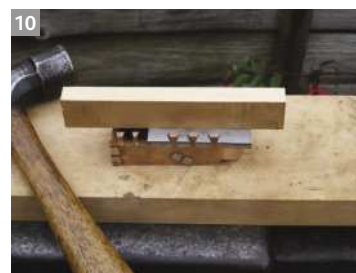
Marking out the joints on the sole (left) with the assembled body. Bill then cuts and files away the dovetails on the sole, and then fits one half of the sole (above left) ready for peining having made sure everything is flat. Then the joints on body and sole can be filed flat (above right)
