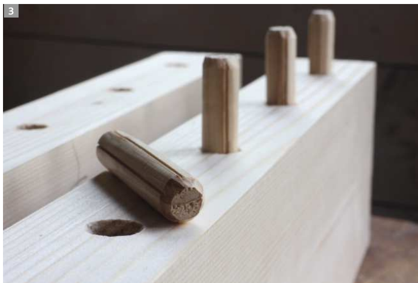
Chamfering a dowel hole (above) to accommodate the glue squeezed out. Dowels in place (below) and the joint ready for assembly
