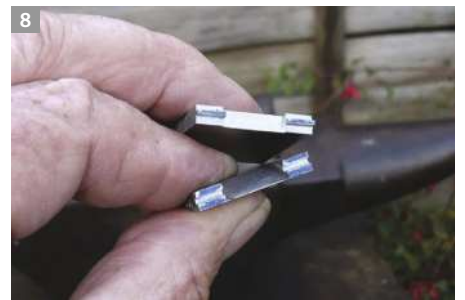
The halves of the sole must be carefully joined by filing, otherwise they might buckle or twist (above)
