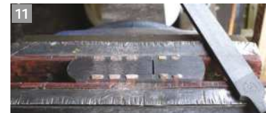
Marking out the joints on the sole (left) with the assembled body. Bill then cuts and files away the dovetails on the sole, and then fits one half of the sole (above left) ready for peining having made sure everything is flat. Then the joints on body and sole can be filed flat (above right)
