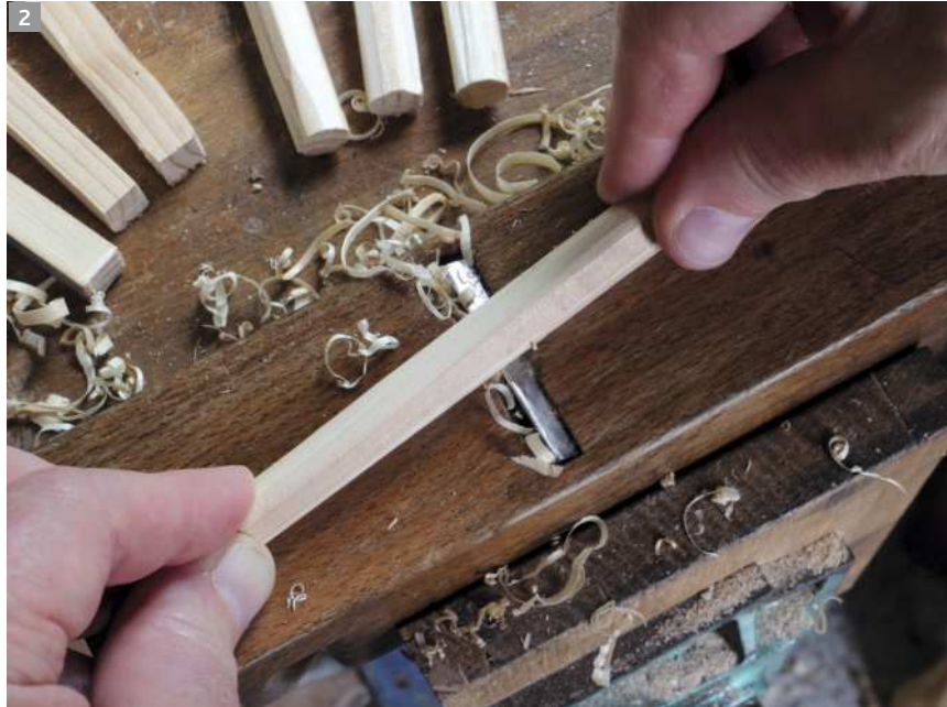
Roughly rounding blanks on an inverted plane gripped in the vice (above). Filing a countersink on the dowel plate with a rat-tail file (below)
