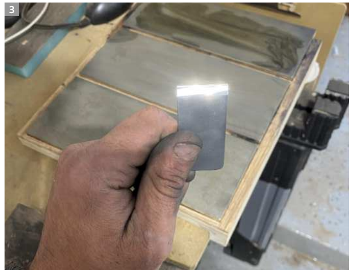
"There is," Curtiss promises, "curvature (above) to the blade." The lapping compound makes it easy to see your flattening process (below)
