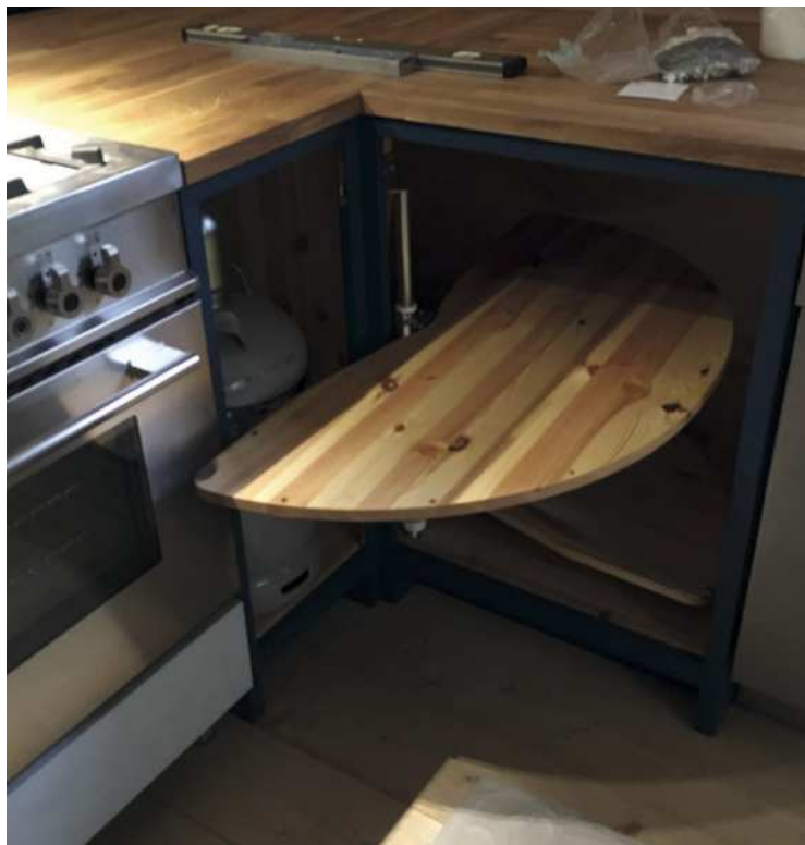
The carousel and shelves in place in the finished cupboard (above). The first stage of prototyping (Pic.1, below left) and midway through assembly (below). Note the sturdy central post to which the carousel hardware will be screwed
