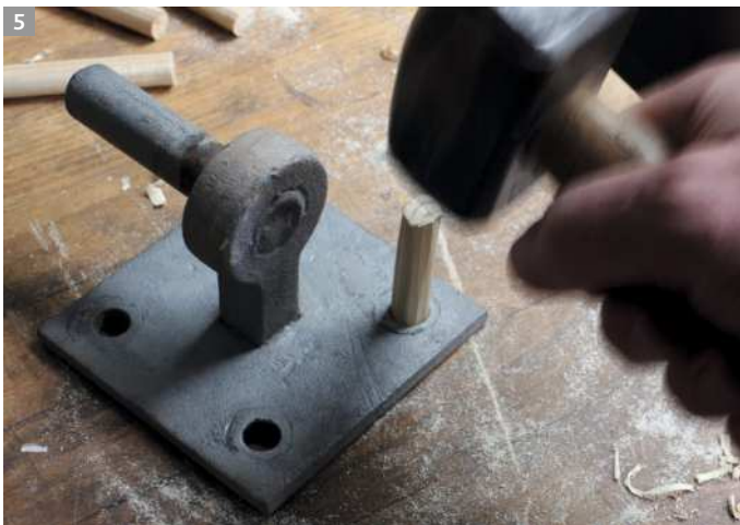
Pointing an end (above) to ease knocking the blank through the gate-hook dowel plate. A lump hammer knocks the blank through the hole (below)
