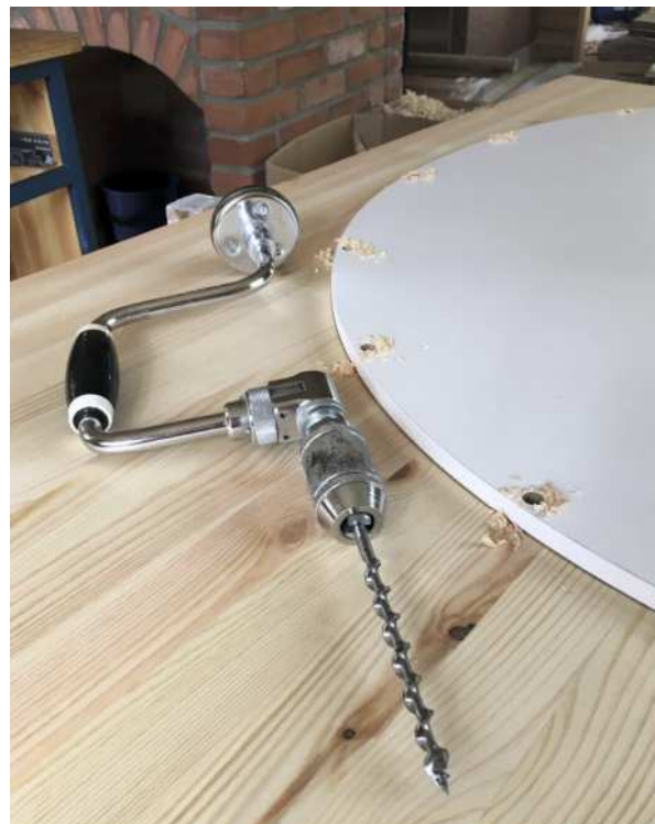
Using a brace and bit (above) to transfer the holes from the Ikea shelf onto the solid wooden one
