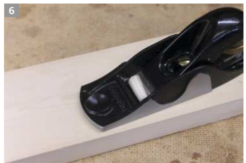
Press the shavings tight to the mouth (left) to control tear-out, and the trick works great for small sections of difficult grain (above). The last shaving is a record of the last blade setting
