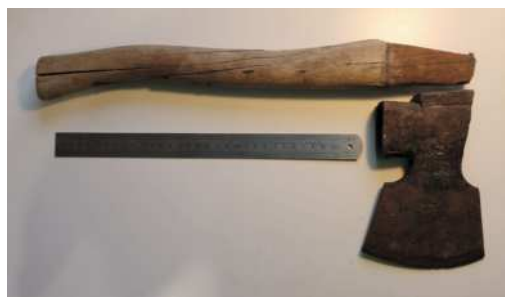
One of Per Nordlöv's earlier stamps (left): "P N L \ Garanti. In English Per Nordlöv, Warranty. The original handle (above) had an overall pleasant shape, but it had split and had been repaired with a nail. The forging line (right) shows where the poll has been added to the body
