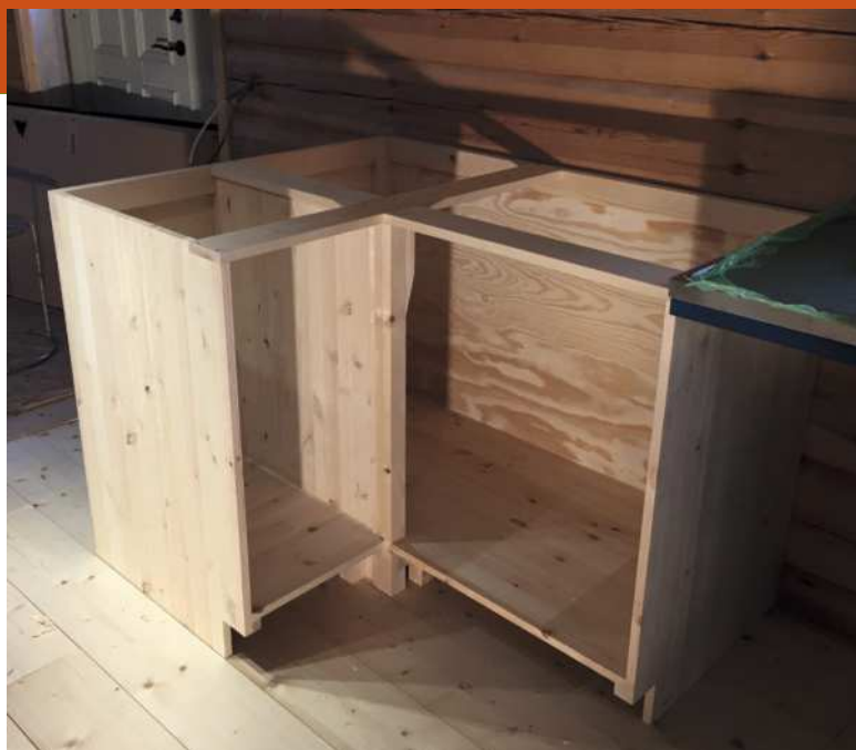
The finished carcass (above) and a view from underneath (below). The two mortise holes in the face-frame are where the legs will be attached
