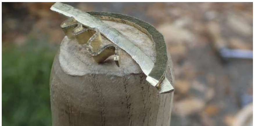
Macro photo (left) showing the ideal wedge-shaped cross section that results from the hammering. The finished rivet (above) ready to hammer into the bowl. Pliers being used (right) to bend the hammered strip into the wavy Cairns Bowl shape. The three stages of zig-zag rivet manufacture (below). The curved strip (right below), hammered and straightened (middle below) and bent (left below)
