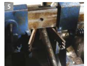
Inserting the bridge with a wide washer as a spacer (left), then the body is bent around the end of a metal rod using sash cramps (right)
