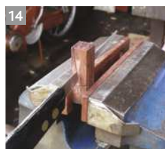
The little plane ready for lapping on the plate (left). The iron is an old one split into four (above left), then the wedge is cut and filed to shape (above right)
