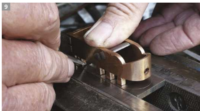
Fitting the bridge into the bent body (left), and the body is tightened with a washer spacer and again can be peined on an anvil (above)
