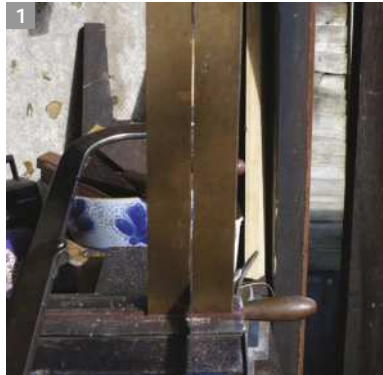
Bill halves the brass back of a tenon saw to make the body of a small mitre plane
