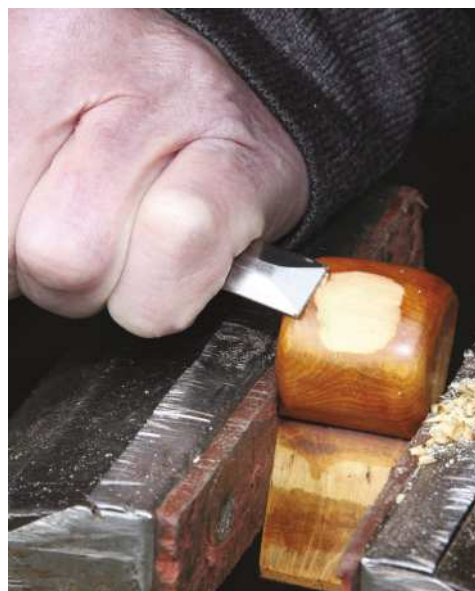
Bill Carter's iconic Blunt Chisel Tip, which starts with the bevel ground off the end of a paring chisel (left) to make it flat across the end (above) for working in any direction, into any tight spot, on any wood and along, across or against the grain (right)
