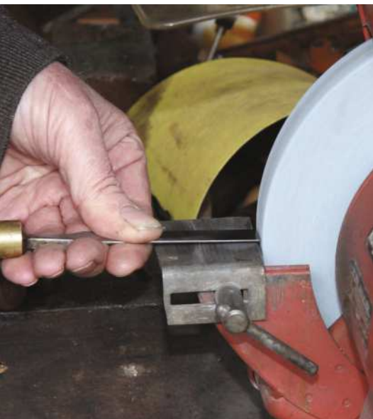
Bill Carter's iconic Blunt Chisel Tip, which starts with the bevel ground off the end of a paring chisel (left) to make it flat across the end (above) for working in any direction, into any tight spot, on any wood and along, across or against the grain (right)
