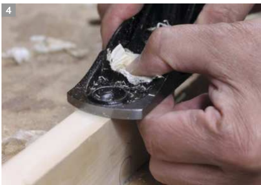
2 Broken shavings mean the board isn't flat (above). You can alter the shape of shavings by skewing a cut (right) or cupping the mouth to control how the shaving exits the plane
