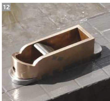
The little plane ready for lapping on the plate (left). The iron is an old one split into four (above left), then the wedge is cut and filed to shape (above right)
