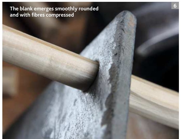
Pointing an end (above) to ease knocking the blank through the gate-hook dowel plate. A lump hammer knocks the blank through the hole (below)
