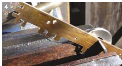
Bill halves the brass back of a tenon saw to make the body of a small mitre plane
