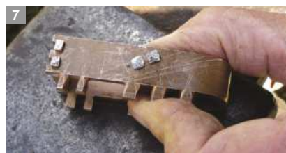
Fitting the bridge into the bent body (left), and the body is tightened with a washer spacer and again can be peined on an anvil (above)
