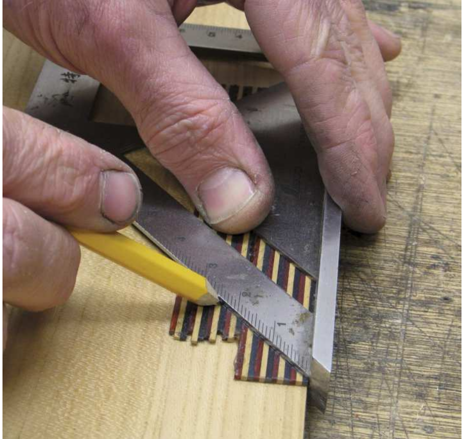
Mark up the stringing with a mitre square at 45° as the first step in making herringbone band (above). Cut at 45° with a fine saw (below)
