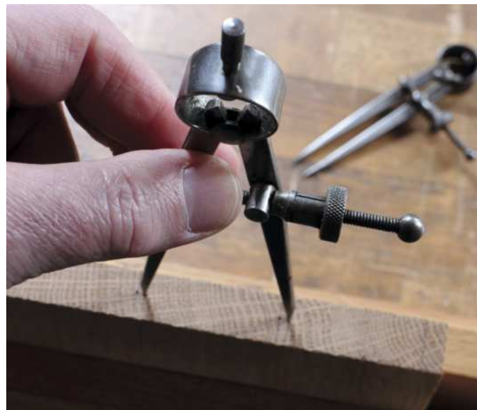
Contemplating the good points of Best Lancashire spring dividers (left). The locking mechanism (above) of M&W dividers loosened to show the split 'Quick Nut'. Spacing dovetails (below) using M&W toolmakers' Sheffield spring dividers
