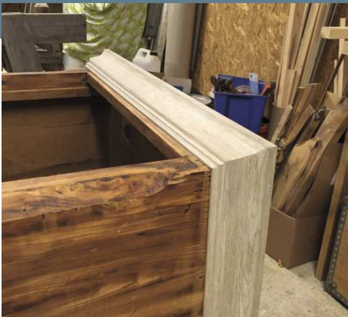
Dry-fitting the newly assembled cornice (above), stained and oiled (right)
