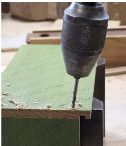
Leaning the drill over a bit, so that the wooden nail can enter deeper into wood without splitting the top edge (above)
