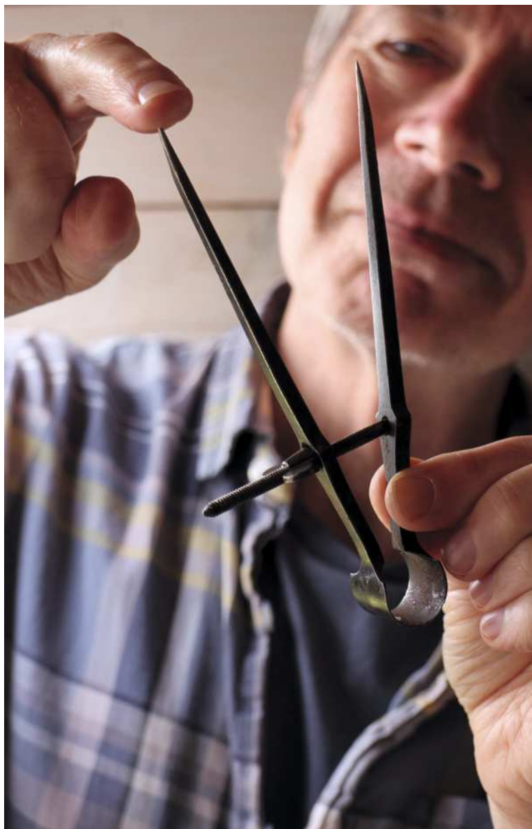
Contemplating the good points of Best Lancashire spring dividers (left). The locking mechanism (above) of M&W dividers loosened to show the split 'Quick Nut'. Spacing dovetails (below) using M&W toolmakers' Sheffield spring dividers
