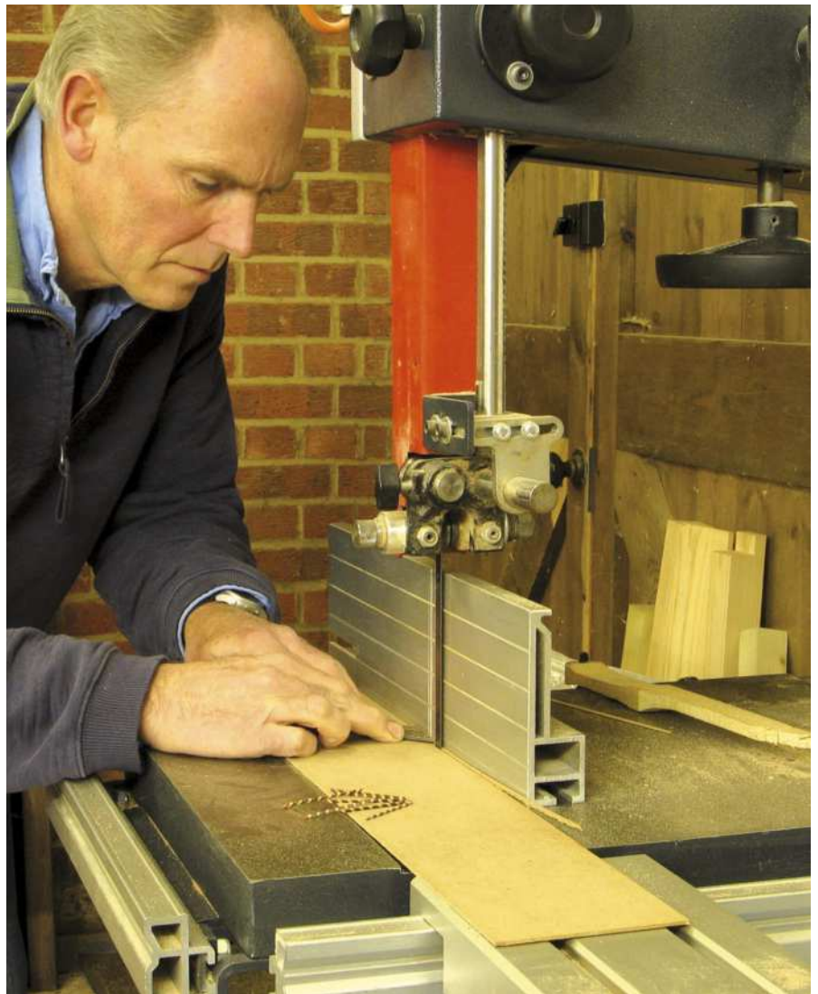
Using a false table on the bandsaw (above and right) to produce short lengths of 'rope', as on p.41. Take great care with this cut, perhaps using a much lower, false fence to keep fingers from the blade
