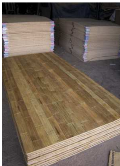
Processed and woven bamboo 4x8ft sheet materials ready for export (left). Some of the bamboo species found in Vietnam are amongst the most solid and thick-walled bamboos on our planet (above)
