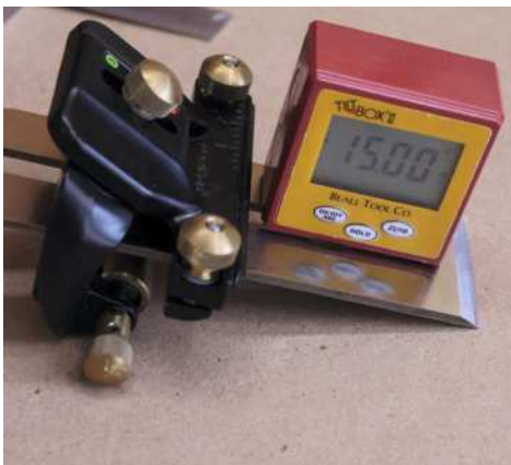
Charles Mak sits an inclinometer on plane a blade to adjust angles with a honing guide p62
