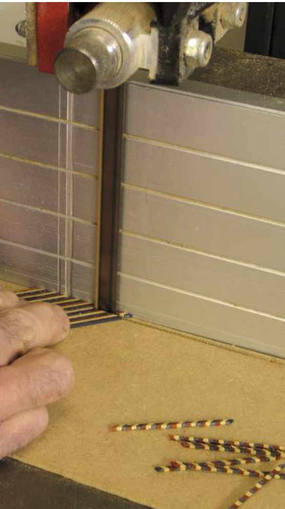
Using a false table on the bandsaw (above and right) to produce short lengths of 'rope', as on p.41. Take great care with this cut, perhaps using a much lower, false fence to keep fingers from the blade
