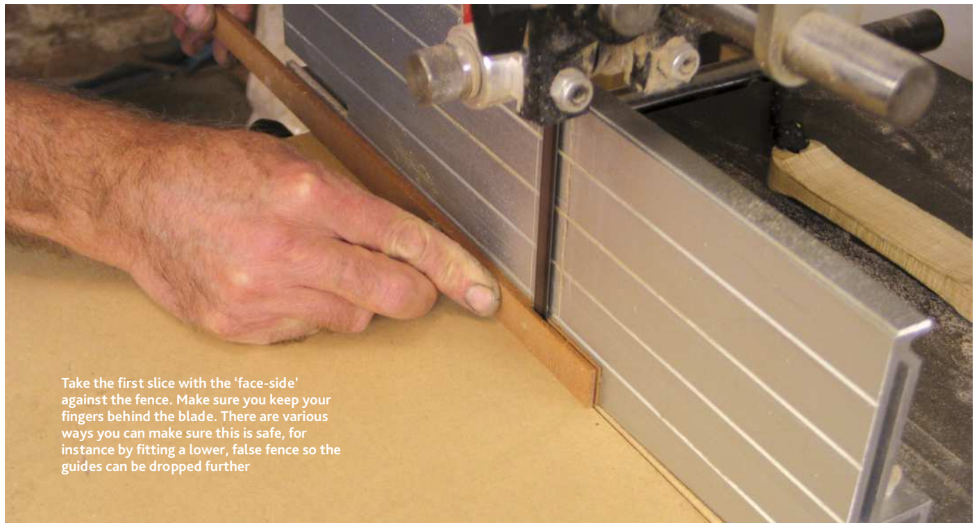
Using a false table on the bandsaw (above and right) to produce short lengths of 'rope', as on p.41. Take great care with this cut, perhaps using a much lower, false fence to keep fingers from the blade
