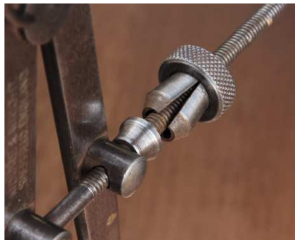
Contemplating the good points of Best Lancashire spring dividers (left). The locking mechanism (above) of M&W dividers loosened to show the split 'Quick Nut'. Spacing dovetails (below) using M&W toolmakers' Sheffield spring dividers
