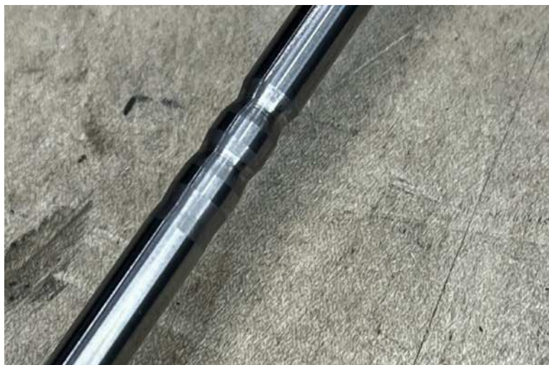
The first Blackburn Tools carbide burnishers (above) with spalted handles. The three grooves that make up the Accu-Burr (right), for a finest hook on the left and coarsest on the right
