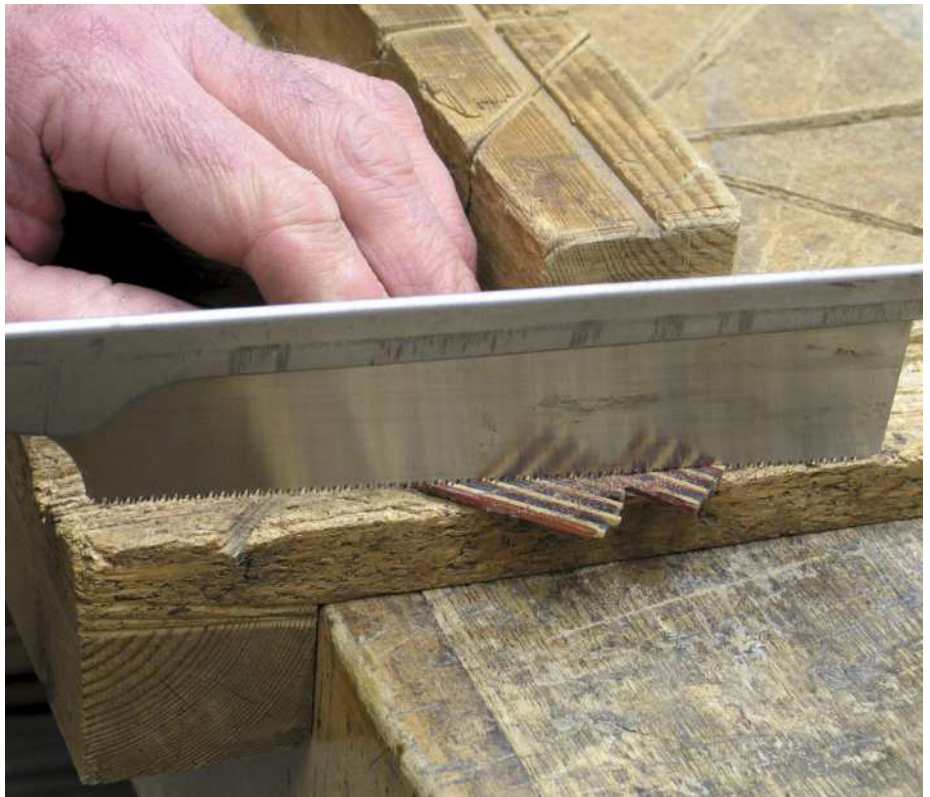
Mark up the stringing with a mitre square at 45° as the first step in making herringbone band (above). Cut at 45° with a fine saw (below)
