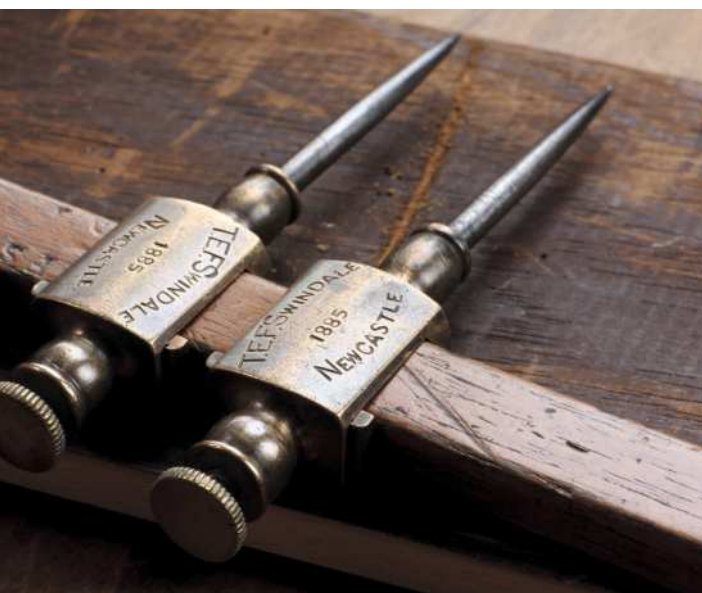
TEF Swindale's 1885 brass trammel heads (above left) on the original mahogany beam. Old tools marked with an owner's name and date establish a personal connection (left). M&W's 'Points of Superiority' illustrated in the company's 1952 catalogue (above)
