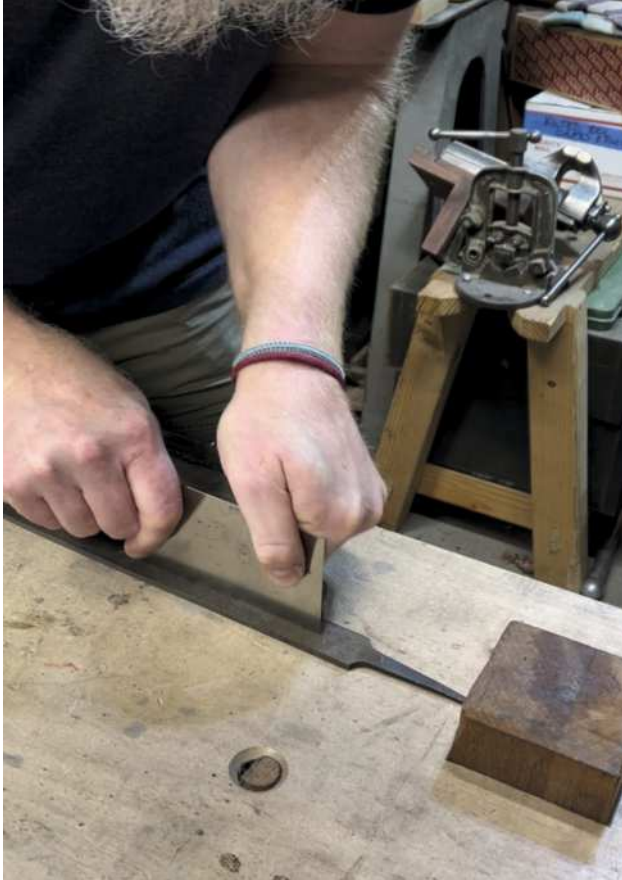
Pushing a scraper over a mill file (above). Burnishing the face of a scraper (above right). Turning the hook with the Accu-Burr (below) and one fitted with a London pattern bog oak handle (right)
