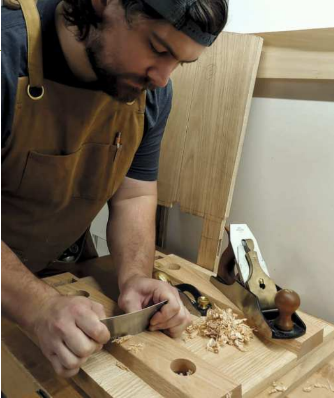
Using a card scraper to clean up the bottom of a chair (above) and using sliding dovetail plane to shape a joint (right)
