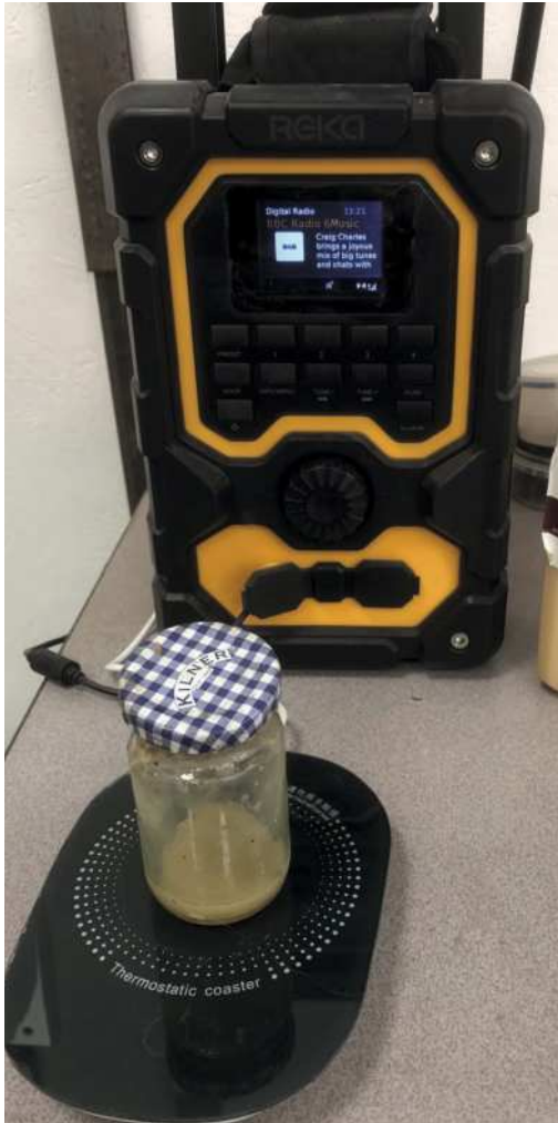
Bill also uses a Thermostatic Drink Coaster (above), powered via USB from the back of a DAB radio. The weight of the bottle switches on a gentle heat just hot enough to warm a pot of fish glue on a cold day
