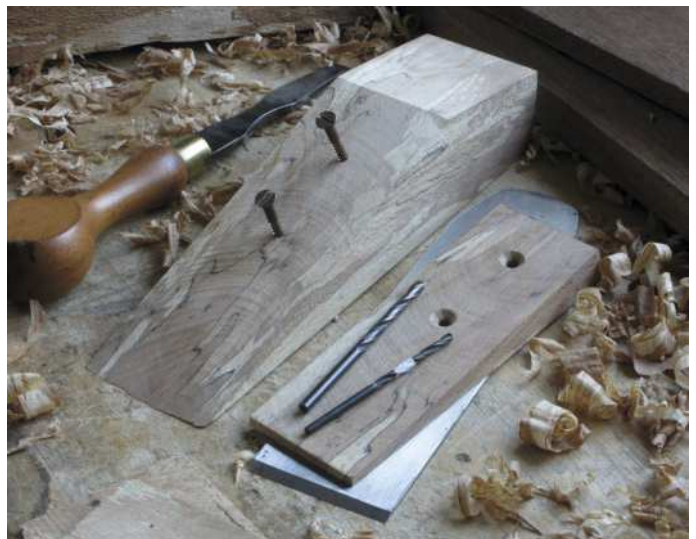
Two bronze wood screws hold the cap and blade to the bed (above). The chisel plane in spalted beech from a special tree has a 2in blade (below)
