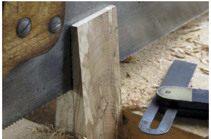
Sawing a 17^\circ bed for the blade (above) and cutting a slice of beech to clamp the blade (below)
