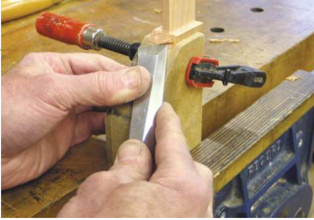
Using a chisel to trim a mitre calls for a slicing cut (above). Using your body and legs to drive the chisel (right). A long-bladed paring chisel making a stopped cut (below)
