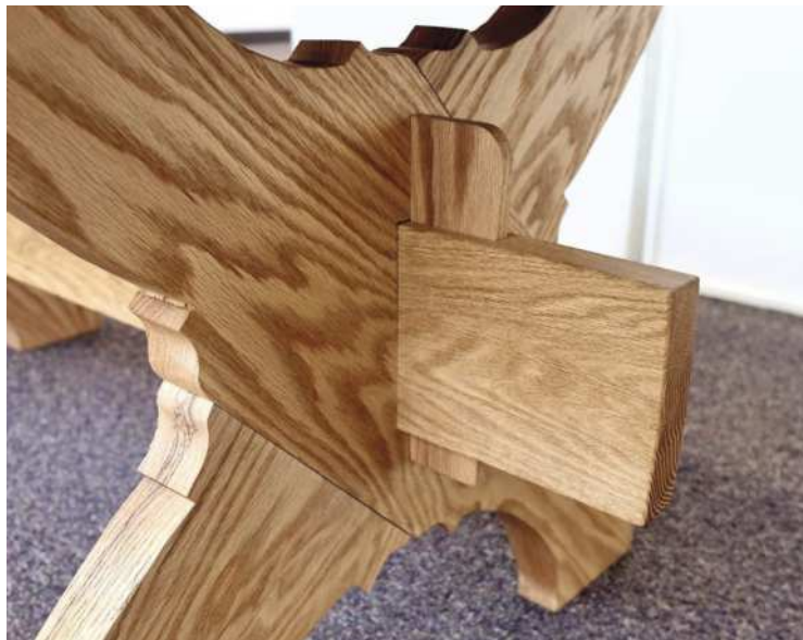
Sawbuck mortise and tusk tenon joinery (above) on a dining table frame. Spiral shavings spilling from the sliding dovetail plane (left), cutting with the grain
