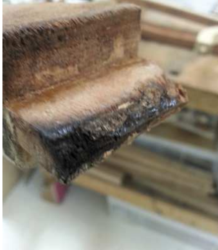
Using a steamer to reverse protein glue (above) and a charred tenon (left) on a 19th Century chair rail. All the tenons on this chair were burnt like this
