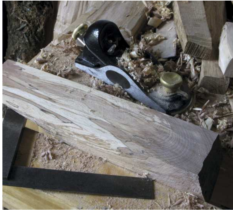
Two faces of the souvenir chunk of beech roughly squared with the axe (right) and flattening the sole with the Stanley 9½ block plane (above)
