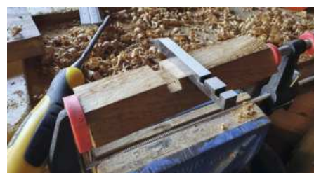
Cutting the recess (above) for the iron
