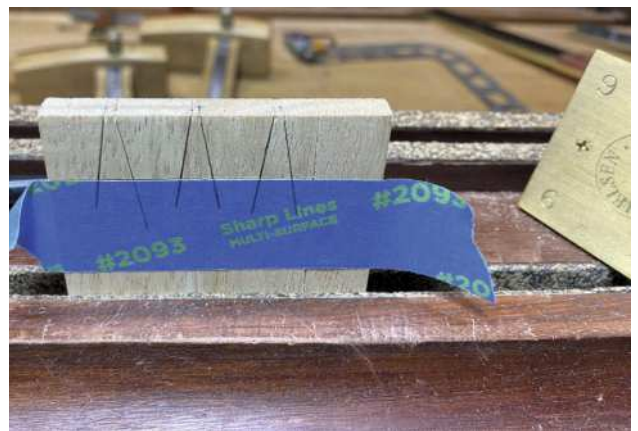
Marking up the tails with blue tape for visibility (above, Pic.3), with the tail positions transferred onto blue tape (left, Pic.2). Slope the chisel away from the opposite side when 'tenting' the sockets (Pic.4, below)
