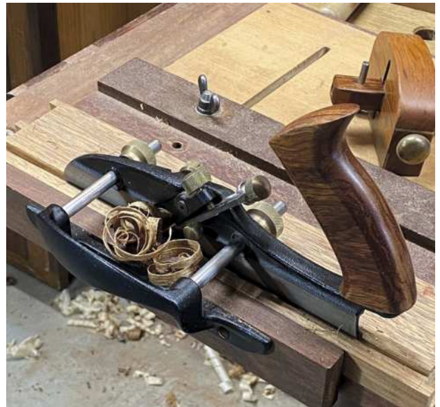
While the drawer front is held in a sticking board, the groove for the drawer bottom is ploughed (above, Pic.1)
