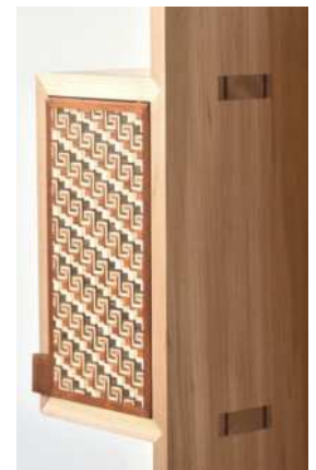
Zigzag (above left) is made with mitre joints for the triangle, with reinforcements, with 45° mitre to the base. It is made from lenga and American walnut. Cadena (above right) is made from lenga for the body, MDF for the door, padouk for the wedges, dowels and handle
