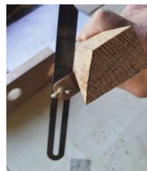
Cutting the mango wood from Surrey Timbers. Two pieces (above) prepped. The 50° angle for the rest (right)
