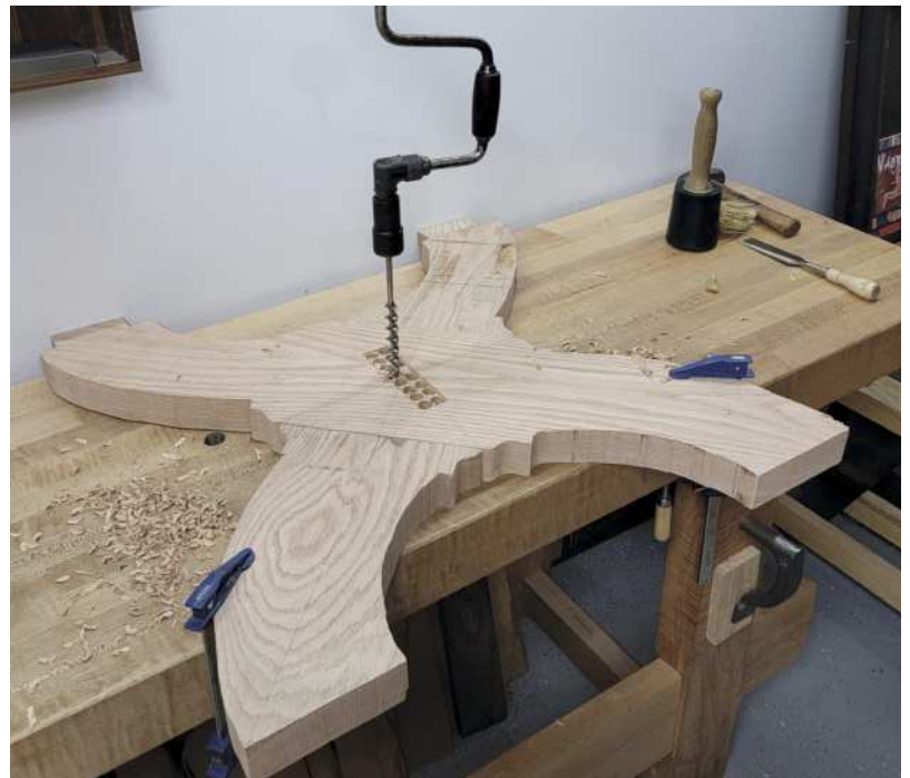
Using the frame of a dial indicator (above) to hold a pencil for marking cut lines for levelling chair legs. Using an auger bit and brace (right) to remove waste for the sawbuck table leg
