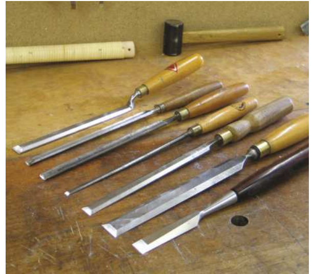
Horizontal chiselling of a tenon shoulder (left) is where the traditional long-bladed paring chisel excels. A selection (above) of old and new paring chisels, and Lie-Nielsen chisels with standard and paring handles (below)
