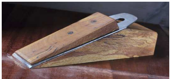
Two bronze wood screws hold the cap and blade to the bed (above). The chisel plane in spalted beech from a special tree has a 2in blade (below)
