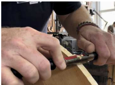
The 5/8in Wood Owl Tri-Cut auger bit (left) was borrowed from another student. This is one of the tools Ethan will be getting for his own shop soon. Refining the edge of the top (above) with Ethan's Millers Fall N.1 circular spokeshave. Breaking the edges on a rung (right) with a bronze No.101 block plane. Drilling by hand (below) and students showing the cricket tables (below right)
