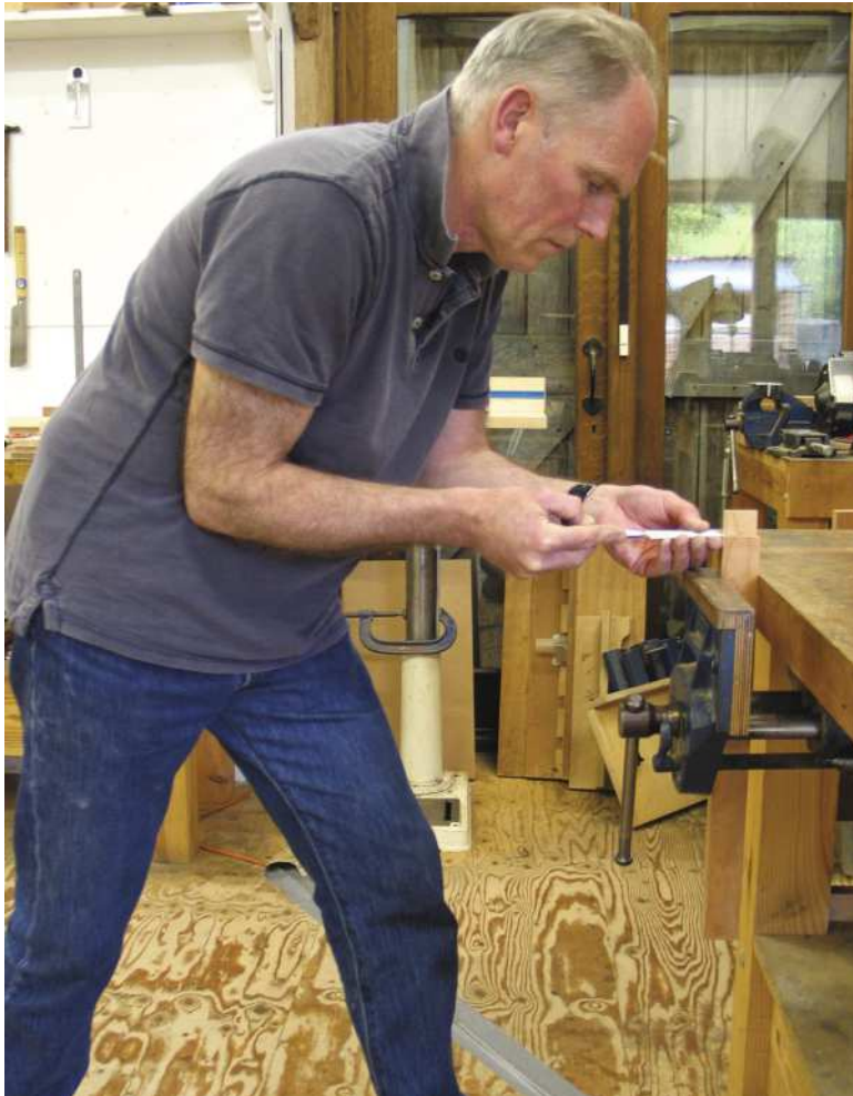
Horizontal chiselling of a tenon shoulder (left) is where the traditional long-bladed paring chisel excels. A selection (above) of old and new paring chisels, and Lie-Nielsen chisels with standard and paring handles (below)
