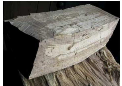
Two faces of the souvenir chunk of beech roughly squared with the axe (right) and flattening the sole with the Stanley 9½ block plane (above)
