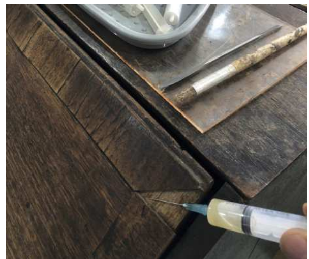
David Cracknell (left) using fish glue for the first time on Bill's chairmaking course. David (@cinque.ports.woodworks) is vice-chairman of Woodland Heritage and a director of Whitney Sawmills. Using a syringe (above) to fix a loose piece of veneer
