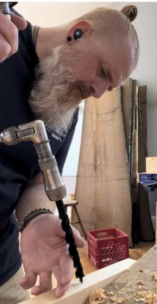
The 5/8in Wood Owl Tri-Cut auger bit (left) was borrowed from another student. This is one of the tools Ethan will be getting for his own shop soon. Refining the edge of the top (above) with Ethan's Millers Fall N.1 circular spokeshave. Breaking the edges on a rung (right) with a bronze No.101 block plane. Drilling by hand (below) and students showing the cricket tables (below right)
