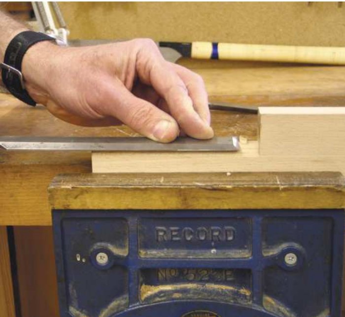
Using a chisel to trim a mitre calls for a slicing cut (above). Using your body and legs to drive the chisel (right). A long-bladed paring chisel making a stopped cut (below)
