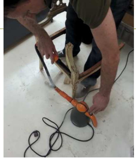
Using a steamer to reverse protein glue (above) and a charred tenon (left) on a 19th Century chair rail. All the tenons on this chair were burnt like this
