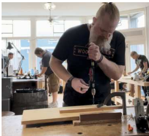
The 5/8in Wood Owl Tri-Cut auger bit (left) was borrowed from another student. This is one of the tools Ethan will be getting for his own shop soon. Refining the edge of the top (above) with Ethan's Millers Fall N.1 circular spokeshave. Breaking the edges on a rung (right) with a bronze No.101 block plane. Drilling by hand (below) and students showing the cricket tables (below right)
