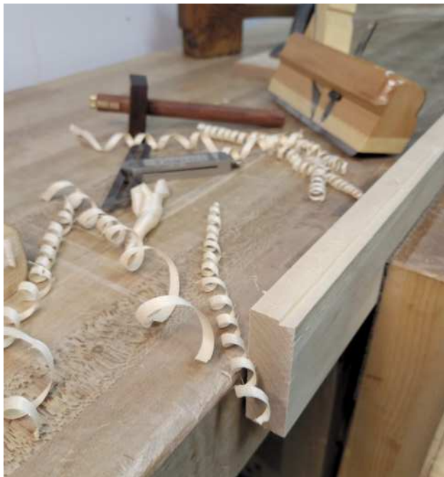
Sawbuck mortise and tusk tenon joinery (above) on a dining table frame. Spiral shavings spilling from the sliding dovetail plane (left), cutting with the grain
