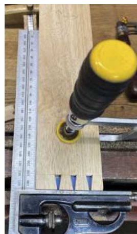
Marking up the tails with blue tape for visibility (above, Pic.3), with the tail positions transferred onto blue tape (left, Pic.2). Slope the chisel away from the opposite side when 'tenting' the sockets (Pic.4, below)
