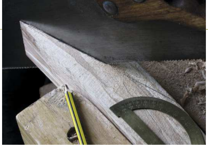
Sawing a 17^\circ bed for the blade (above) and cutting a slice of beech to clamp the blade (below)
