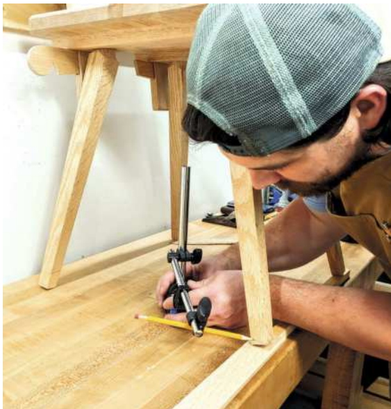
Using the frame of a dial indicator (above) to hold a pencil for marking cut lines for levelling chair legs. Using an auger bit and brace (right) to remove waste for the sawbuck table leg
