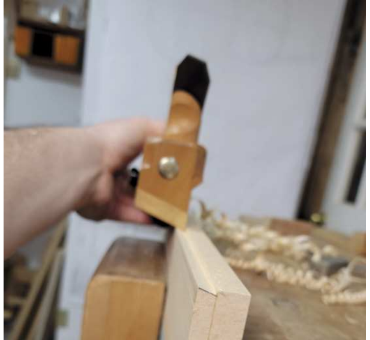
Using a card scraper to clean up the bottom of a chair (above) and using sliding dovetail plane to shape a joint (right)
