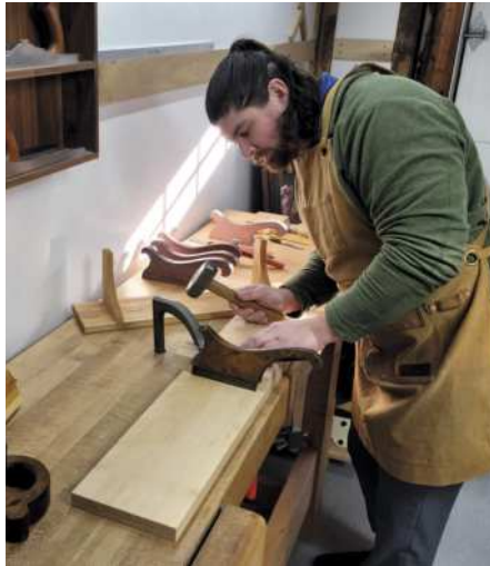
Aligning the fence to cut sliding dovetails
