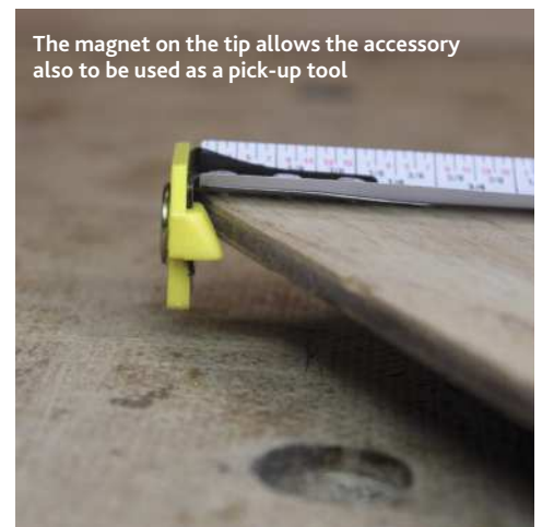
The square check prevents the tape measure from sliding off the corner
