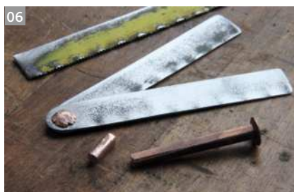
Peening the nail without a rove (left) makes a low-profile rivet. The mini-bevel with remains of the hacksaw blade (above). A practical rove punch (right) can be made from a stretcher
