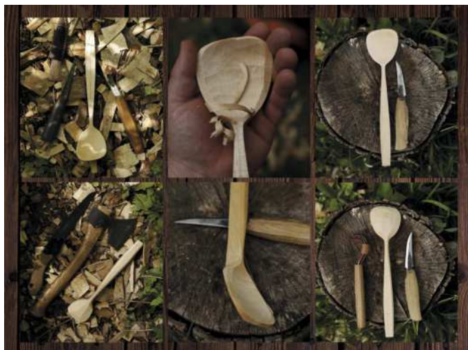
Top left to right: 'Circumference' carved and initial hollow done; 'Crank' carved in; and top profile 'Cleaning' done. Bottom left to right: tools for the axing stages; carved 'Crank' transition; bottom profile 'Cleaned' and showing the basic tools for the knife stages
