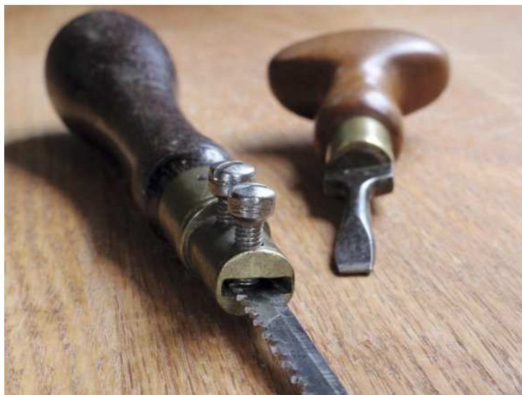
Cheese-head machine screws clamp the padesaw's adjustable blade (above). Extravagant and simple handle shapes (above right) of the compass saw and padesaw. The 19th Century compass saw makes a tidy exit from the kerf (below left). Touching up the teeth of the compass saw with a Stubs file (below). The narrow blade of the padesaw follows a curve in moulded plywood (right)
