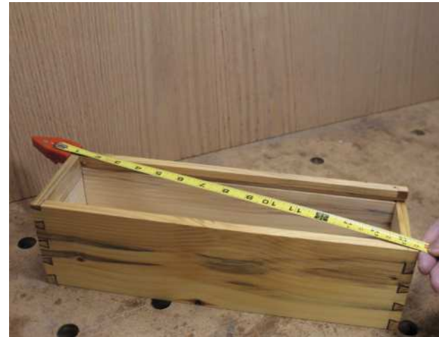
The magnet on the tip allows the accessory also to be used as a pick-up tool
