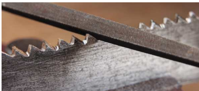
Cheese-head machine screws clamp the padesaw's adjustable blade (above). Extravagant and simple handle shapes (above right) of the compass saw and padesaw. The 19th Century compass saw makes a tidy exit from the kerf (below left). Touching up the teeth of the compass saw with a Stubs file (below). The narrow blade of the padesaw follows a curve in moulded plywood (right)
