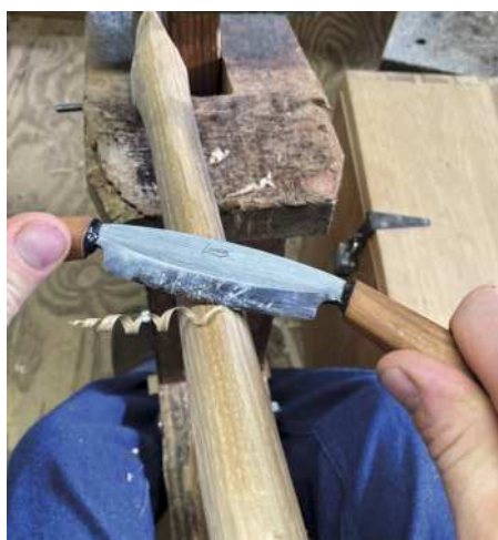
Pulling to shape an axe handle (left and above). Jason Lonon (right) at his shop in North Carolina, USA, holding a hand-forged hatchet
