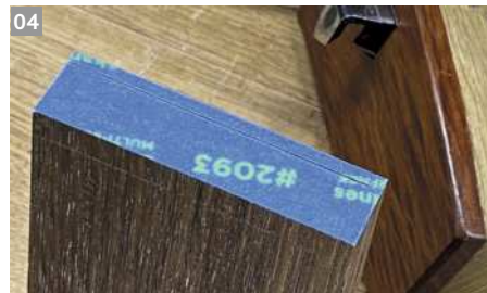
Derek's blue tape method (introduced by him in 2011), is good for end-grain (above) and for transferring lines held on the Moxon vice (left). Peel away the tape inside the sockets (below) and you are left with crisp lines for the saw
