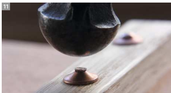
The bored and countersunk punch slips over the nail (above) and the rove. Elliott-Lucas end-cutters nipping the nail to length (above right). Well-targeted tapping of the ball-peen hammer (below) spreads the nail over the rove. The glittering prize (right) is a secure and neatly-finished rivet
