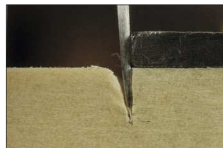
One photo in the Layout Tools section shows options when it comes to choosing a marking knife, and the importance of the bevel (above)
