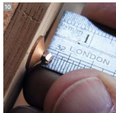
About 3/32in (2mm) is left standing above the rove (above). 4oz, 8oz and 24oz ball-peen hammers (below)
