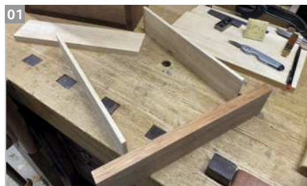
The 18mm drawer front is merbau; a very hard and tough timber. The 7mm sides and 14mm back were part of a Tasmanian oak (which is a Eucalyptus) panel. I seek out Tassie oak for drawer sides as it is sold locally in quartersawn form. This is ideal for minimising wood movement
