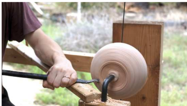
Turning the foot of the bowl (left) with the tip-hook down. Rough turning the hollow (above)
