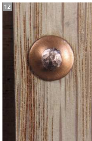
The bored and countersunk punch slips over the nail (above) and the rove. Elliott-Lucas end-cutters nipping the nail to length (above right). Well-targeted tapping of the ball-peen hammer (below) spreads the nail over the rove. The glittering prize (right) is a secure and neatly-finished rivet
