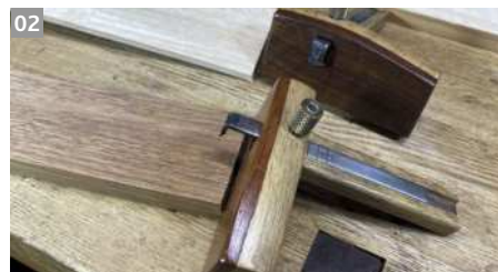
A Japanese-style cutting gauge was made by Derek, based on a Japanese mortice gauge (Kinshiro), which uses two knives. The metal is laminated steel from a Japanese blade. David Charlesworth used knife gauges he converted from Marples pin gauges
