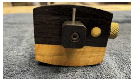
The Superior Marking Gauge kit includes a hardened pin, a cutting gauge, and a pencil, all secured with set screws and an allen wrench (above). Is there anything better than bog oak and boxwood (right)
