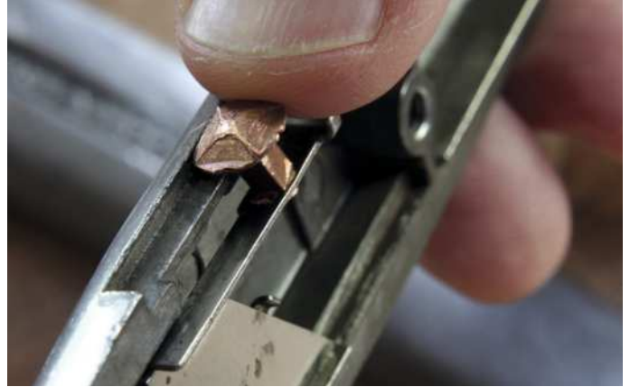
A clenched copper nail replaced the lost button on the Stanley 99 utility knife (above), in action (below) with a curved blade
