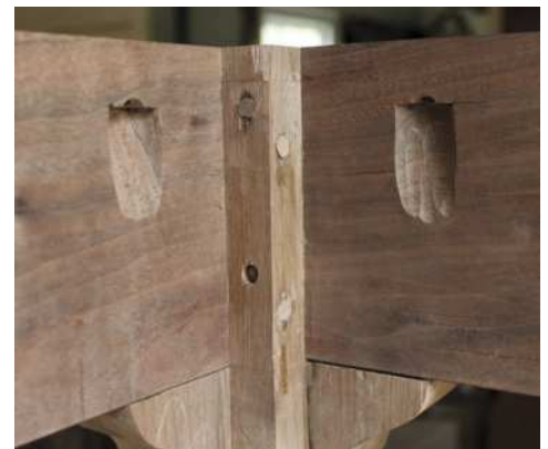
A screw well (above) on an 18th Century Virginian table. Note the maker dug the well too deep and pierced the outside face of the table apron. Two finished screw wells (right) on adjoining aprons of the sideboard table, ready for screws and top attachment
