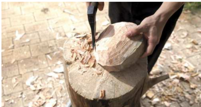
Axing the rough shape of the bowl (above) and the first out pass at the bottom (right)
