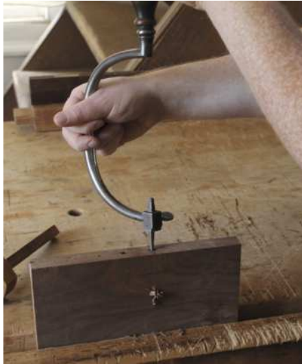
A bit and brace, held at an angle, is used to drill the hole for the screw well
