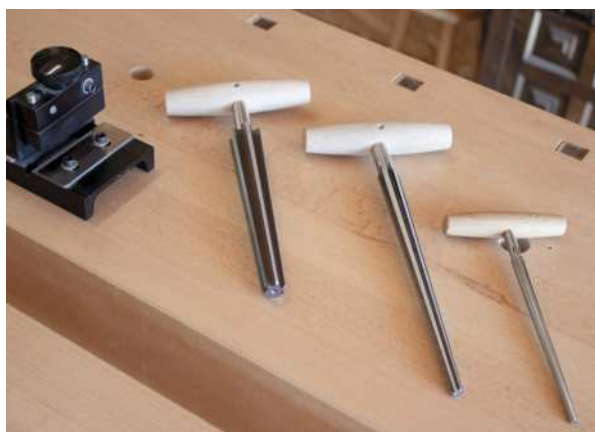
Different peg models (above) in ebony, boxwood and Indian rosewood (above). Luthier's reamers (below) and peg shaper
