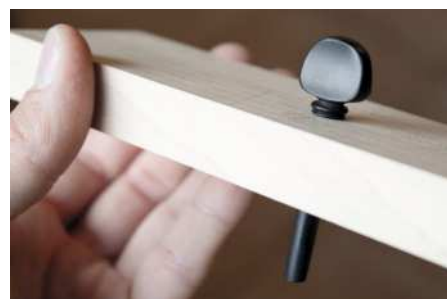
Detail of a wedged peg protruding through a door (above). Choosing the location of any pull (left) may greatly affect the appearance of a piece. Over-long peg (below) fitted to a drawer front
