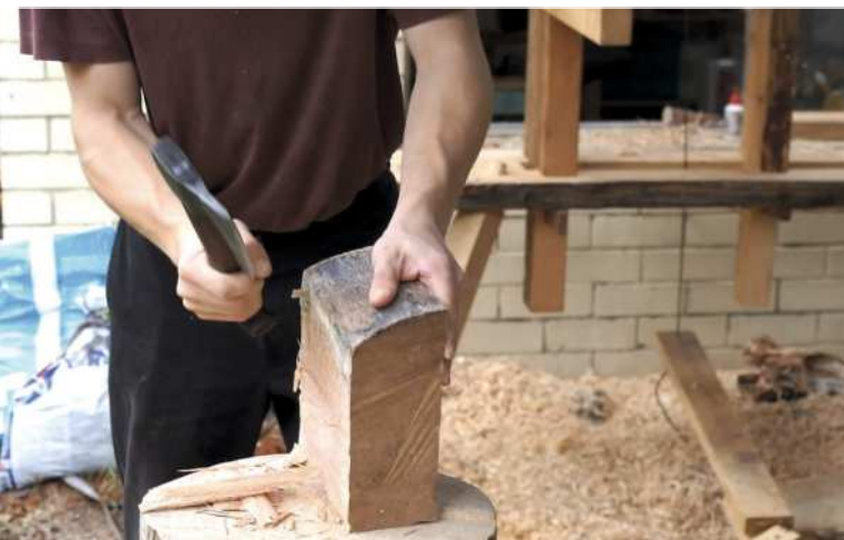
The first step after splitting the blank is flattening the top face (left). Julian uses dividers to scribe a circle and then bore a small hole (above) for an interference fit tenon mandrel
