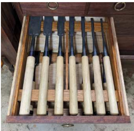
Six Umeki-Oire-Nomi sized chisels (above, from top) 1in, ¾in, ½in, ¼in, ⅜in, and ⅛in. The lowest chisel is a fishtail chisel, which is used to clear the corners of pin sockets. The chisel to the right is a Sokozari, which is used for clearing chips from a mortise. A set of Kiyohisa slicks (right)
