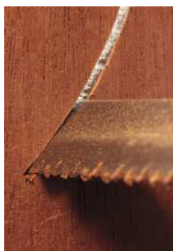
Cheese-head machine screws clamp the padesaw's adjustable blade (above). Extravagant and simple handle shapes (above right) of the compass saw and padesaw. The 19th Century compass saw makes a tidy exit from the kerf (below left). Touching up the teeth of the compass saw with a Stubs file (below). The narrow blade of the padesaw follows a curve in moulded plywood (right)
