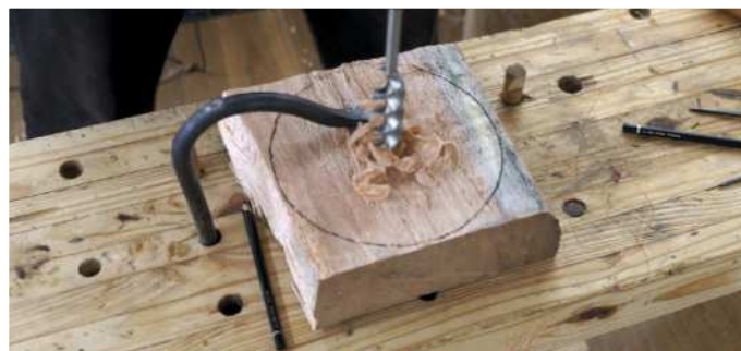
The first step after splitting the blank is flattening the top face (left). Julian uses dividers to scribe a circle and then bore a small hole (above) for an interference fit tenon mandrel
