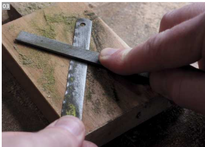
Old paint and high points are filed away along the 'wave-set' edge (left). Clamp the blade and use tin snips (above) to cut the required ends
