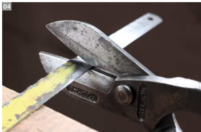
Old paint and high points are filed away along the 'wave-set' edge (left). Clamp the blade and use tin snips (above) to cut the required ends
