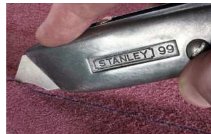
A clenched copper nail replaced the lost button on the Stanley 99 utility knife (above), in action (below) with a curved blade
