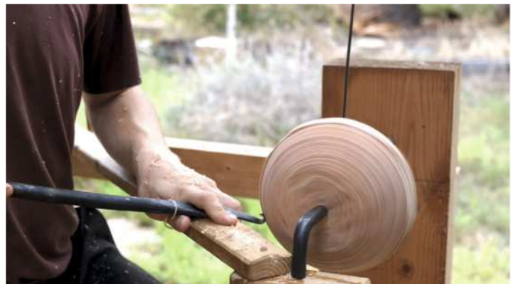
Axing the rough shape of the bowl (above) and the first out pass at the bottom (right)
