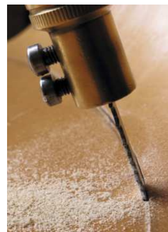
Cheese-head machine screws clamp the padesaw's adjustable blade (above). Extravagant and simple handle shapes (above right) of the compass saw and padesaw. The 19th Century compass saw makes a tidy exit from the kerf (below left). Touching up the teeth of the compass saw with a Stubs file (below). The narrow blade of the padesaw follows a curve in moulded plywood (right)
