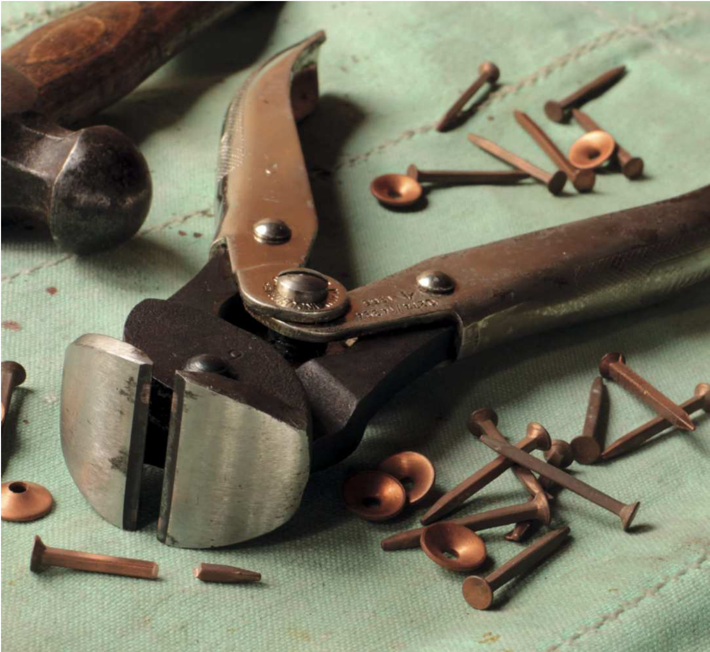
When it comes to snipping the rivets, compound lever nippers by Maun Industries (above) are easiest on the hands. Oak and mahogany riveted using square copper nails and roves (below). Angles are recorded on straight-edged card for future reference (right)
