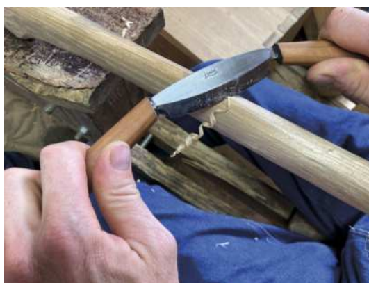
Pulling to shape an axe handle (left and above). Jason Lonon (right) at his shop in North Carolina, USA, holding a hand-forged hatchet
