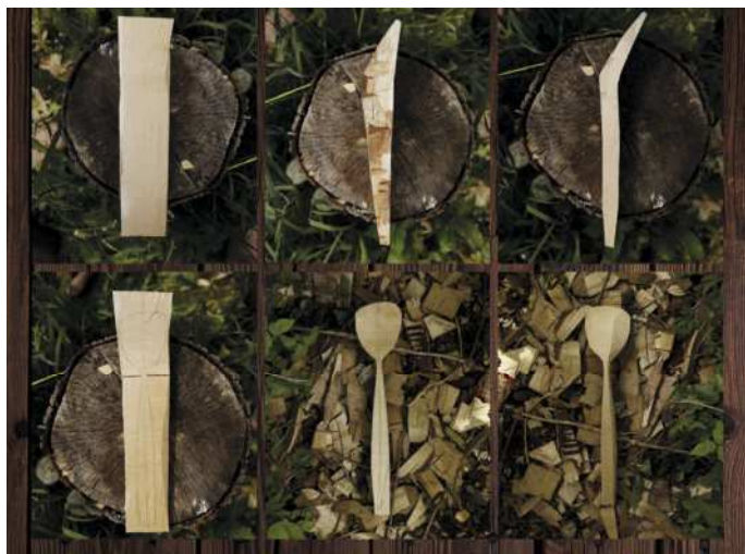
Top left to right: birch billet in radial grain orientation; bottom 'Crank' axed in; and 'Crank' matched. Bottom left from right: design drawn and stop cuts sawn in; 'Circumference' axed out; 'Cleaning' done
