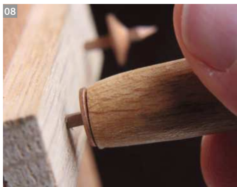
The bored and countersunk punch slips over the nail (above) and the rove. Elliott-Lucas end-cutters nipping the nail to length (above right). Well-targeted tapping of the ball-peen hammer (below) spreads the nail over the rove. The glittering prize (right) is a secure and neatly-finished rivet
