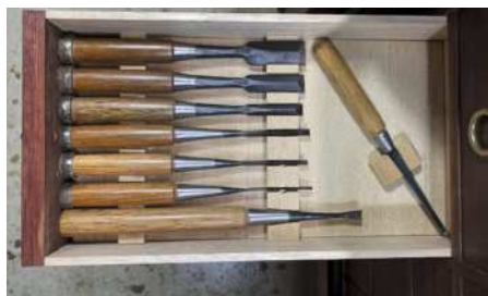
Six Umeki-Oire-Nomi sized chisels (above, from top) 1in, ¾in, ½in, ¼in, ⅜in, and ⅛in. The lowest chisel is a fishtail chisel, which is used to clear the corners of pin sockets. The chisel to the right is a Sokozari, which is used for clearing chips from a mortise. A set of Kiyohisa slicks (right)
