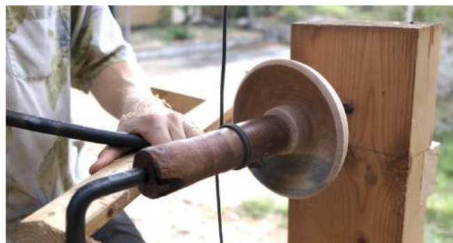
Turning the foot of the bowl (left) with the tip-hook down. Rough turning the hollow (above)
