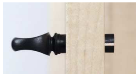
Detail of a wedged peg protruding through a door (above). Choosing the location of any pull (left) may greatly affect the appearance of a piece. Over-long peg (below) fitted to a drawer front
