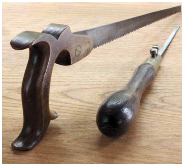
Cheese-head machine screws clamp the padesaw's adjustable blade (above). Extravagant and simple handle shapes (above right) of the compass saw and padesaw. The 19th Century compass saw makes a tidy exit from the kerf (below left). Touching up the teeth of the compass saw with a Stubs file (below). The narrow blade of the padesaw follows a curve in moulded plywood (right)
