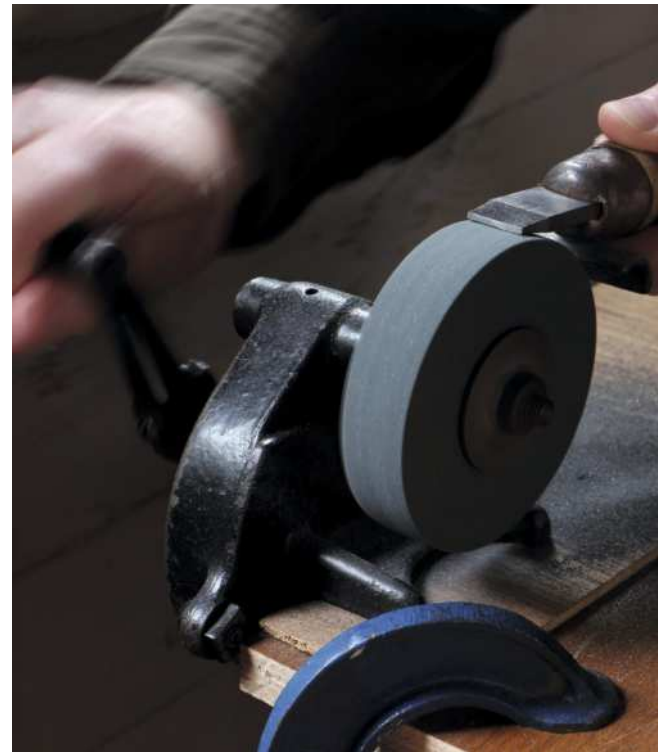
Sawing the shank with the Eclipse No.670 Junior hacksaw (left), then hollow grinding the tip on the hand-cranked Black Knight grinder (above) to produce a dedicated broad-tipped screwdriver for plane iron screws (right)
