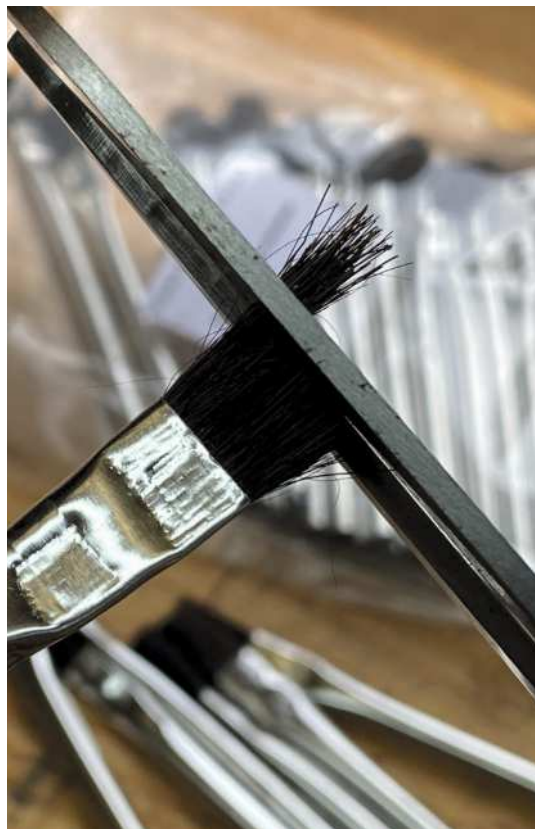
Clinching down the body of a cheap glue brush (above) helps holding the bristles in place. The bristles on these brushes are far too long (right) and need a good haircut before they're any good
