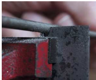
Shaping the side bead profile with a round file (above) having snipped a rusty Stanley Fatmax with Gilbow metal shears (right) and gloved hands. The cutter is sandwiched with cut-away L-shaped cheeks (below)
