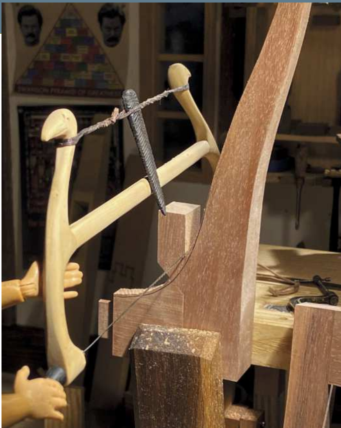
The bowsaw is made from a bandsaw blade with a feather-shaped toggle
