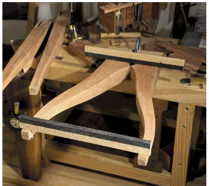
The curves on the legs are so shallow that it is hard to hide a glue line if you choose to make them from two pieces
