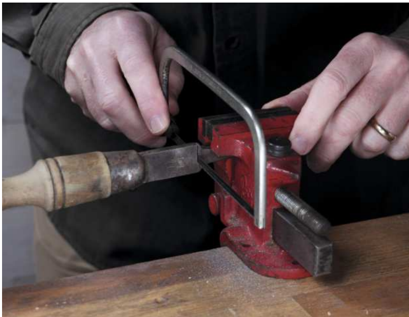
Sawing the shank with the Eclipse No.670 Junior hacksaw (left), then hollow grinding the tip on the hand-cranked Black Knight grinder (above) to produce a dedicated broad-tipped screwdriver for plane iron screws (right)
