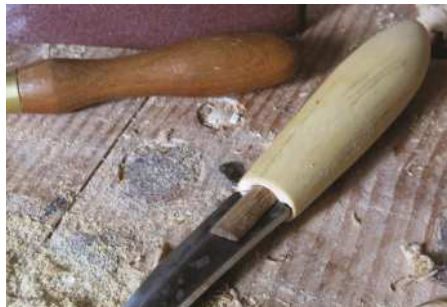
Sean uses a simple technique for fitting a handle to a new or old knife, drilling a blank and fitting a split piece of dowel to hold the tang
