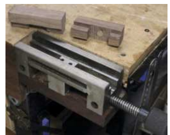
One of the jaws is made low-profile to handle thinner materials against a bench dog (above). You can now enjoy the use of a tail vice without breaking the bank (left)
