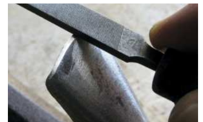
The broken-down beast (above) dug from the garden. Hacksawing the initial bevel was slow work (left), and filing a back bevel (below) to ease the blade's exit
