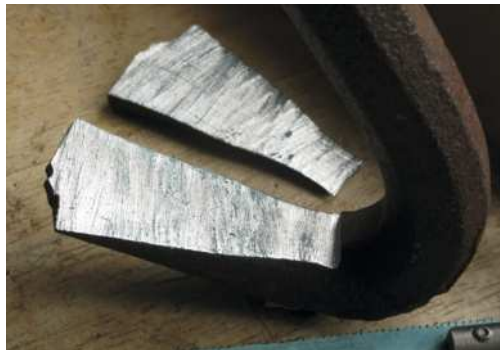
The broken-down beast (above) dug from the garden. Hacksawing the initial bevel was slow work (left), and filing a back bevel (below) to ease the blade's exit
