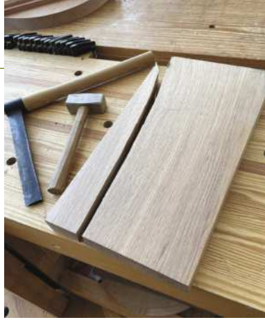
Riving follows the grain (above). The grain on the board's edge is straight, but angled on its face. Wood for arms might be salvaged. But you can split kiln-dried stock to produce ideal chair parts (right)
