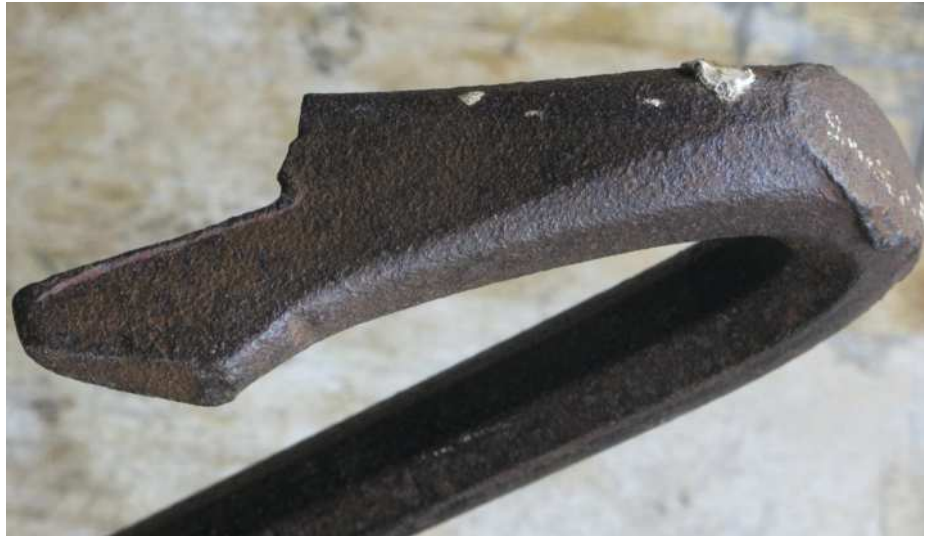
The broken-down beast (above) dug from the garden. Hacksawing the initial bevel was slow work (left), and filing a back bevel (below) to ease the blade's exit
