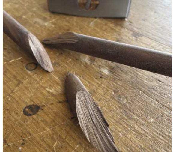
Two victims of the sledge test. Short-grain walnut (above) and brash cherry (below)
