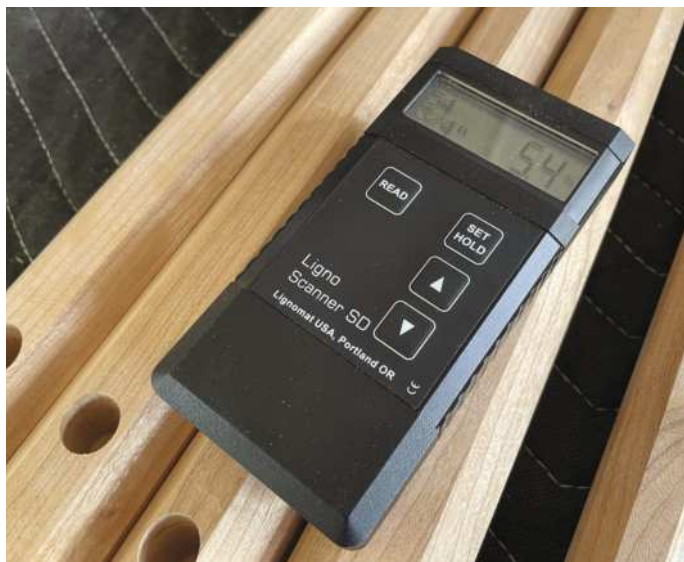
Chris resisted owning a moisture meter for years. It pays for itself the first time you find a problem using this tool
