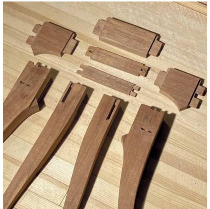
The curves on the legs are so shallow that it is hard to hide a glue line if you choose to make them from two pieces
