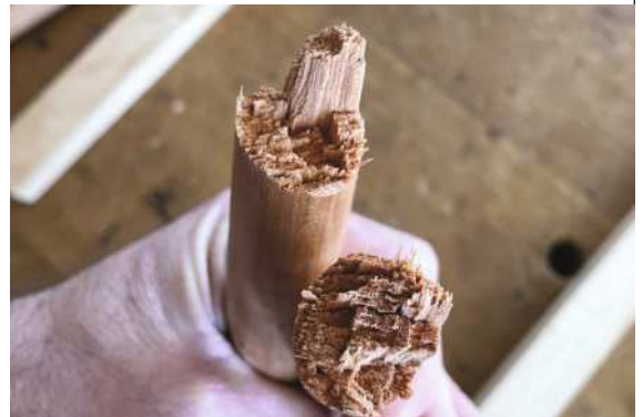
Two victims of the sledge test. Short-grain walnut (above) and brash cherry (below)
