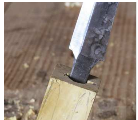
Drill a hole the length and width of the tang (top), using squares to guide the bit. If the tang flares towards the blade file to widen the top of the hole (left). Check the fit of the tang (above) before shaping the handle
