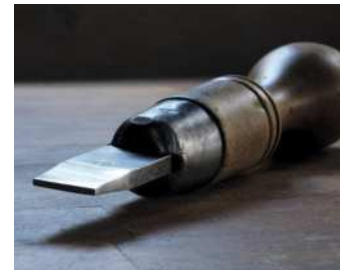
Sawing the shank with the Eclipse No.670 Junior hacksaw (left), then hollow grinding the tip on the hand-cranked Black Knight grinder (above) to produce a dedicated broad-tipped screwdriver for plane iron screws (right)
