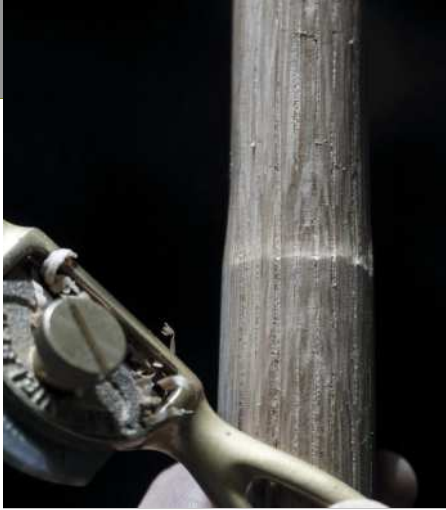
With a concave-sole spokeshave you can taper the tenon shoulder (Pic.4). A leg joint on a stick chair can loosen (below, Pic.1)
