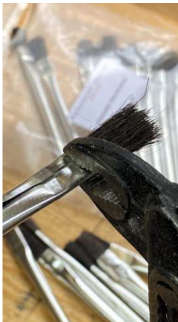
Clinching down the body of a cheap glue brush (above) helps holding the bristles in place. The bristles on these brushes are far too long (right) and need a good haircut before they're any good
