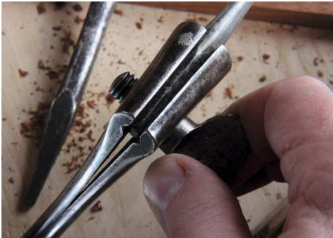
Spofford's 'clamshell' socket (above) excels with square-shanked bits. Using the ratcheting Millers Falls No.422 in a tight spot (right)
