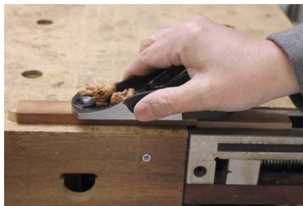
One of the jaws is made low-profile to handle thinner materials against a bench dog (above). You can now enjoy the use of a tail vice without breaking the bank (left)
