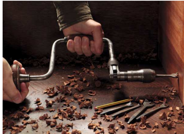
Spofford's 'clamshell' socket (above) excels with square-shanked bits. Using the ratcheting Millers Falls No.422 in a tight spot (right)
