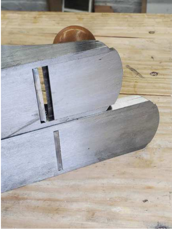
The Sweetheart No.4 (right) is well built, but the tote is big and clumsy. The planes each have an adjustable mouth that can be closed to a hair's breadth (above) or opened like a barn door.
