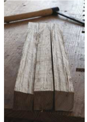
Riving follows the grain (above). The grain on the board's edge is straight, but angled on its face. Wood for arms might be salvaged. But you can split kiln-dried stock to produce ideal chair parts (right)
