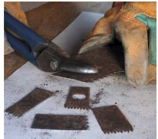
Shaping the side bead profile with a round file (above) having snipped a rusty Stanley Fatmax with Gilbow metal shears (right) and gloved hands. The cutter is sandwiched with cut-away L-shaped cheeks (below)
