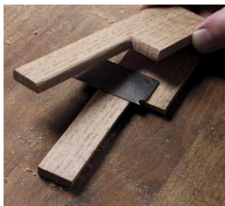
Shaping the side bead profile with a round file (above) having snipped a rusty Stanley Fatmax with Gilbow metal shears (right) and gloved hands. The cutter is sandwiched with cut-away L-shaped cheeks (below)
