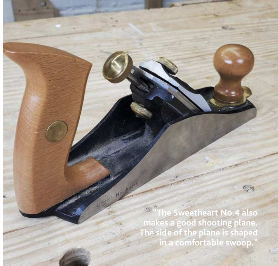
The Sweetheart No.4 (right) is well built, but the tote is big and clumsy. The planes each have an adjustable mouth that can be closed to a hair's breadth (above) or opened like a barn door.
