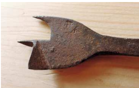
An unsharpened and fettled bit makes a very jagged hole (above). Sharpened, fettled and minimal clean-up (above right) The 7/8in bit after a scrub with a softish wire brush (left) before sharpening and cleaning
