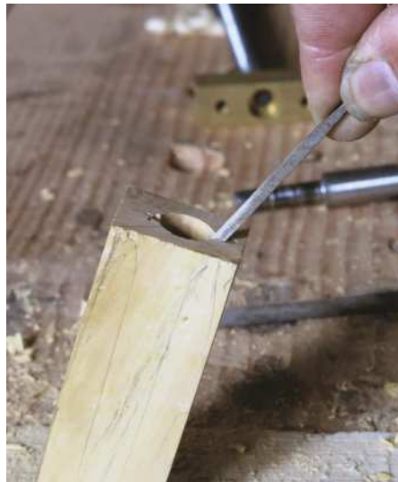
Drill a hole the length and width of the tang (top), using squares to guide the bit. If the tang flares towards the blade file to widen the top of the hole (left). Check the fit of the tang (above) before shaping the handle
