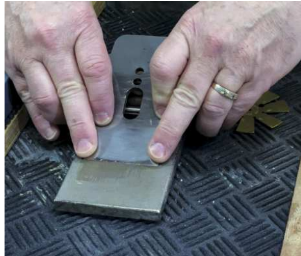
Look for monocrystalline diamond stones for the longest life. With diamond bench stones available in a full range of grits, they cover the gamut of sharpening needs
