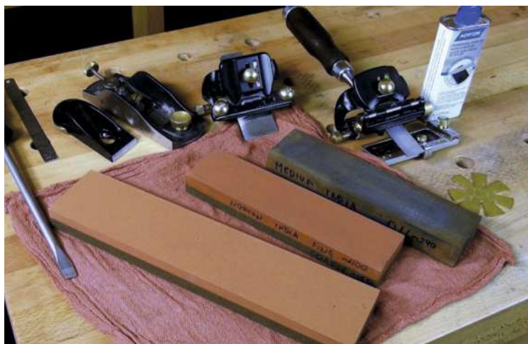
Man-made stones (above) are available in a small range of grits, from coarse, medium to fine. A coarse/fine combination stone is an excellent choice. Natural stones (right) are graded by the hardness of the particles, the harder the particles, the finer the grit
