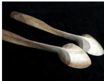
Carving the back of a blackwood ( Acacia melanoxylon ) kitchen spoon (left) and a pair of hickory wattle ( Acacia faciformis ) eating spoons, tangential cut, bark down (above)
