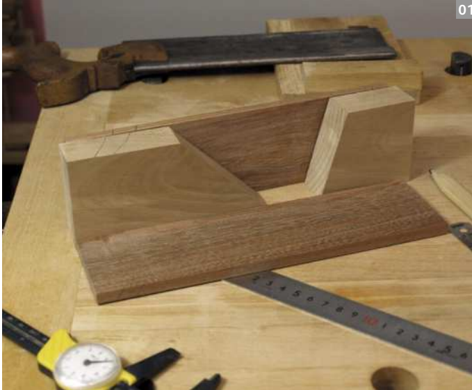
Laminating the body, bed, throat and mouth (Pic.3, above) means there is less chopping to be done. The blade was made from an old Dunlop tyre iron, hardened with Mitch's micro forge (Pic. 4, right)
