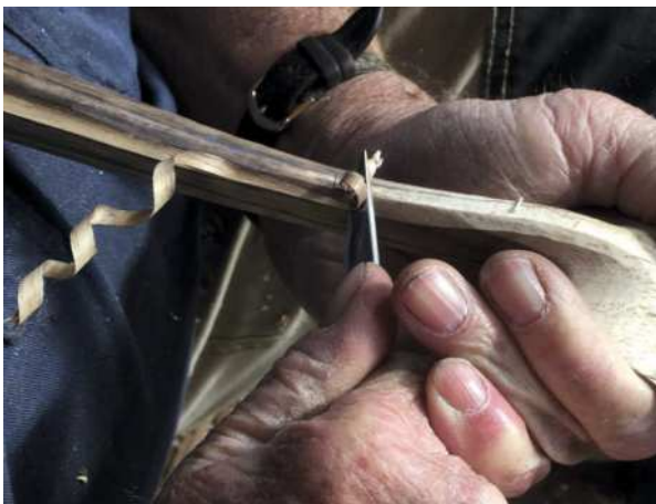
Carving the back of a blackwood ( Acacia melanoxylon ) kitchen spoon (left) and a pair of hickory wattle ( Acacia faciformis ) eating spoons, tangential cut, bark down (above)
