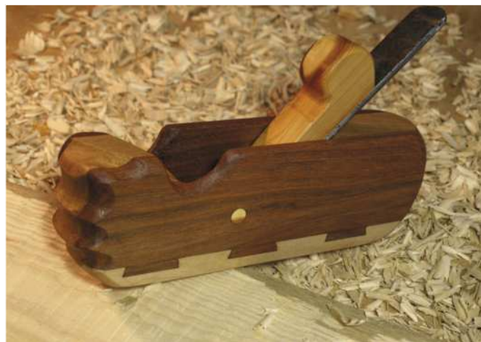
Pic.1 Mitch Peacock's scrub plane has a dovetailed sole
