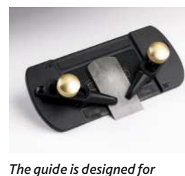
The new Veritas guide comes with a registration plate for setting 30° or 25° bevels, with a shim for honing a micro-bevel
