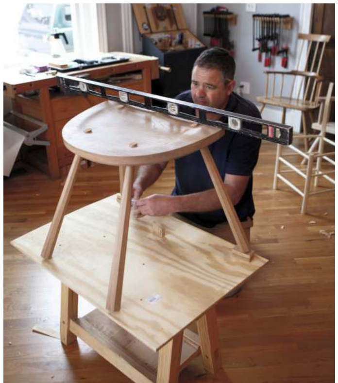
From Good Work , Chris using small wedges and blocks of wood to level the chair side to side
