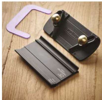
The new Veritas guide comes with a registration plate for setting 30° or 25° bevels, with a shim for honing a micro-bevel
