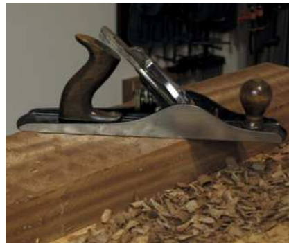
Pic.2 Shaving thickness has been limited by the Stanley No.5's mouth
