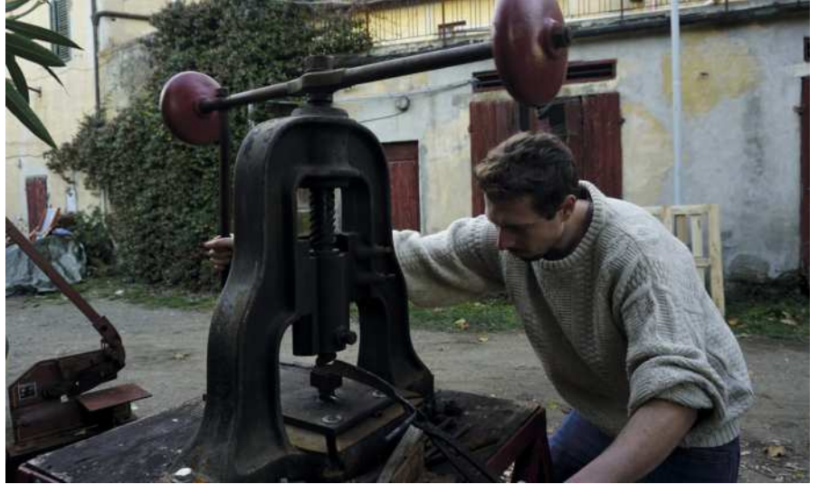
Forging a drawknife on the flypress (right). Sheaths are important working with sharp tools!
