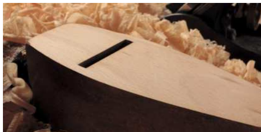
Freshly exposed quarter-sawn beech has a pinkish hue from the boat-shaped Preston smoother (above). Torchlight shows between the Preston wood's sole and the try-square
