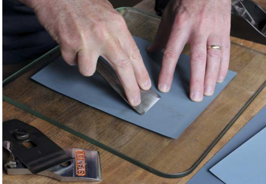
Removing the gubbins from the glass plate of the bathroom scales (above), being used as a flat surface for sharpening a Stanley No. 4 iron using fine abrasive
