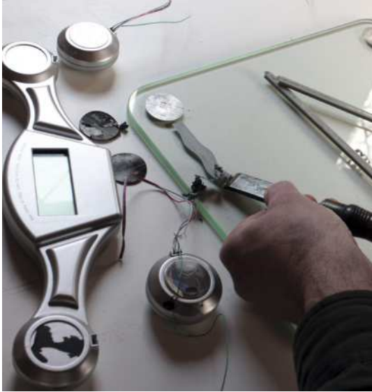
Removing the gubbins from the glass plate of the bathroom scales (above), being used as a flat surface for sharpening a Stanley No. 4 iron using fine abrasive
