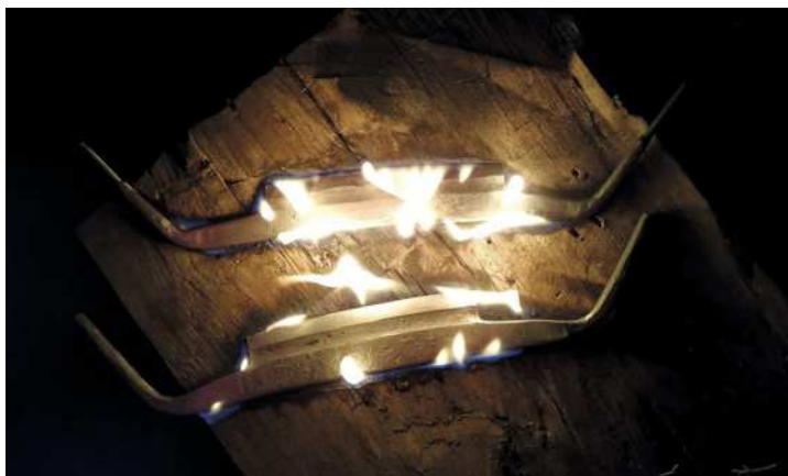
The peened tang holds the handle in place (left) over a coin washer. A forged surface texture (above), and the completed knife over a hand-stitched sheath (right). Drawknives normalizing after forging (below)
