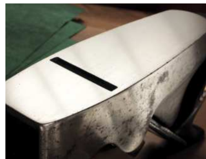
Flattening in progress with emery cloth (left). The Spiers infill sole (above) scored by a hard life, and restored to factory flatness (right)
