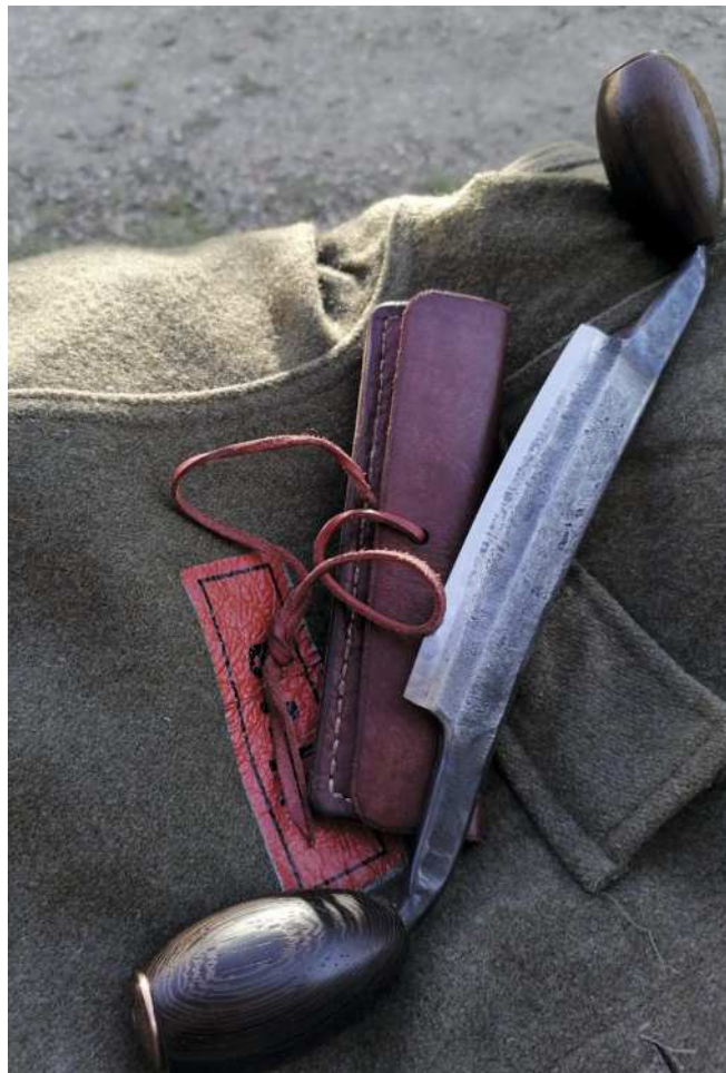
The peened tang holds the handle in place (left) over a coin washer. A forged surface texture (above), and the completed knife over a hand-stitched sheath (right). Drawknives normalizing after forging (below)
