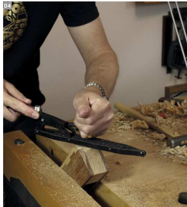
As an added detail Mitch decided to add a dovetailed sole, with the dovetailed grooves (Pic.5, above) set at an angle. The dovetails were sawn by hand, the waste was chiselled out, the bottoms cleaned with a router plane and the sides finished with a side-rebate plane. They didn't need to be angled across the sole, but it does mean the dovetails appear on both sides and ends, which initially looks impossible. After assembly the plane was rasped (Pic.6, right)
