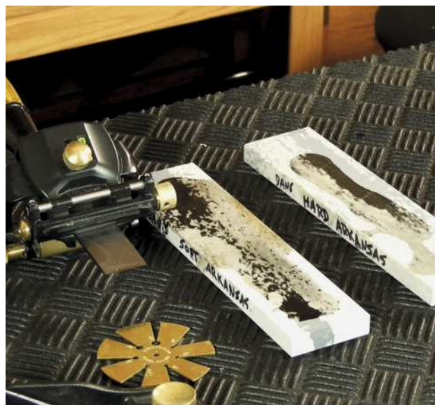
Man-made stones (above) are available in a small range of grits, from coarse, medium to fine. A coarse/fine combination stone is an excellent choice. Natural stones (right) are graded by the hardness of the particles, the harder the particles, the finer the grit
