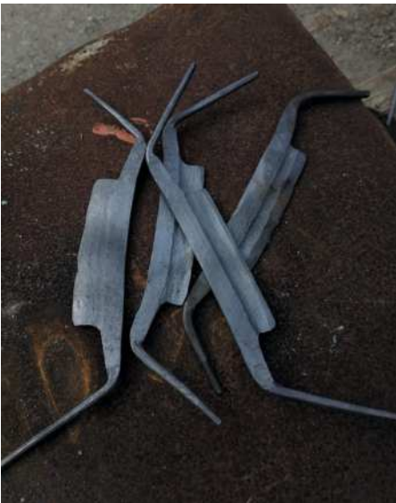
Forged knives before grinding (above). All Benjamin's drawknives are protected by a leather sheath (right). The underside of a knife (below)
