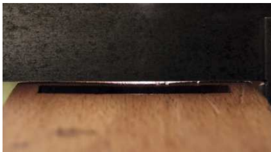
Freshly exposed quarter-sawn beech has a pinkish hue from the boat-shaped Preston smoother (above). Torchlight shows between the Preston wood's sole and the try-square
