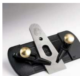
The new Veritas guide comes with a registration plate for setting 30° or 25° bevels, with a shim for honing a micro-bevel
