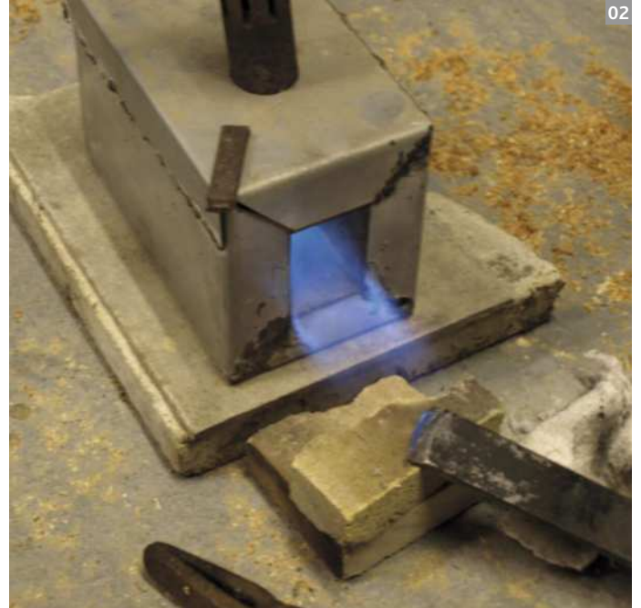
Laminating the body, bed, throat and mouth (Pic.3, above) means there is less chopping to be done. The blade was made from an old Dunlop tyre iron, hardened with Mitch's micro forge (Pic. 4, right)
