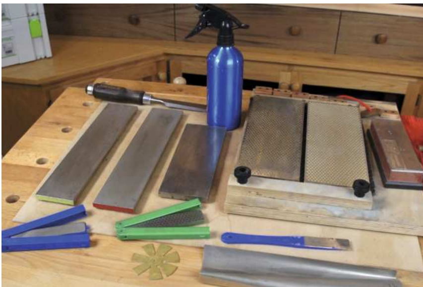
Look for monocrystalline diamond stones for the longest life. With diamond bench stones available in a full range of grits, they cover the gamut of sharpening needs
