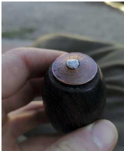
The peened tang holds the handle in place (left) over a coin washer. A forged surface texture (above), and the completed knife over a hand-stitched sheath (right). Drawknives normalizing after forging (below)
