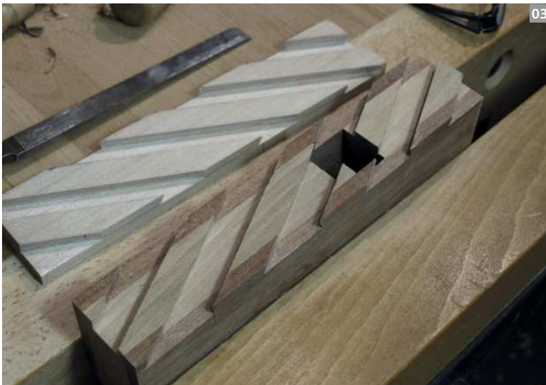
As an added detail Mitch decided to add a dovetailed sole, with the dovetailed grooves (Pic.5, above) set at an angle. The dovetails were sawn by hand, the waste was chiselled out, the bottoms cleaned with a router plane and the sides finished with a side-rebate plane. They didn't need to be angled across the sole, but it does mean the dovetails appear on both sides and ends, which initially looks impossible. After assembly the plane was rasped (Pic.6, right)
