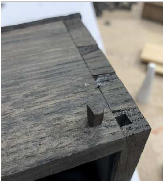
Filling holes left by the 043 plough plane (above), and adding rebates to the boxwood lid (below right). The Fine Old Cannibals Box (below) is the size to fit an LN102 block plane (right), and the size of the plane's cardboard case
