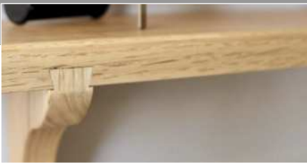
A sliding dovetail joint on a small wall shelf cut with a traditional Gratsäge
