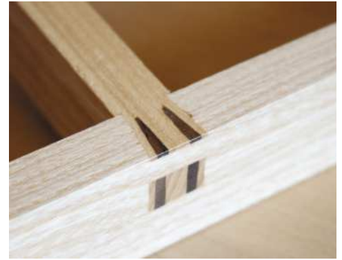
A joinery exercise completed (left) and a dissection of the same joint showing the dovetail shaped tenons (above). Temporary pencil lines (below) show the expansion of the mortises at 1:8 ratio. A knife nick is used to transfer the final lines more precisely
