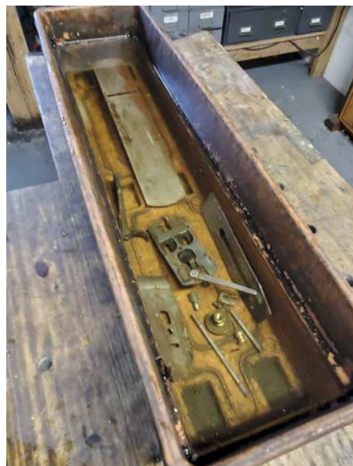
A plane bought with a broken tote (left) and 5lb citric acid bought online (above). A plane disassembled in the citric acid bath (right)
