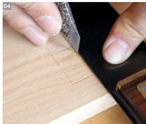
Using the spacer blocks to mark up the joint (left) and tidy marking of the mortises will result in much neater work (above)
