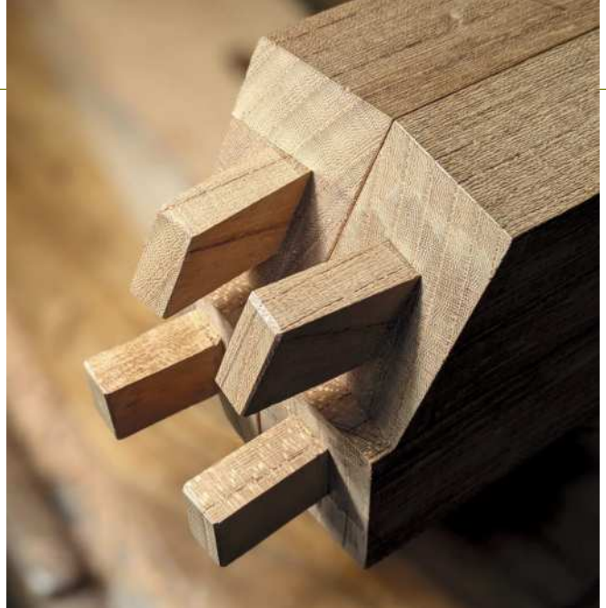
Instead of using typical dowels to connect the legs to the seat, a tenon is cut on the legs for extra strength (above). Getting the angled shoulders to fit flush is the really difficult part
