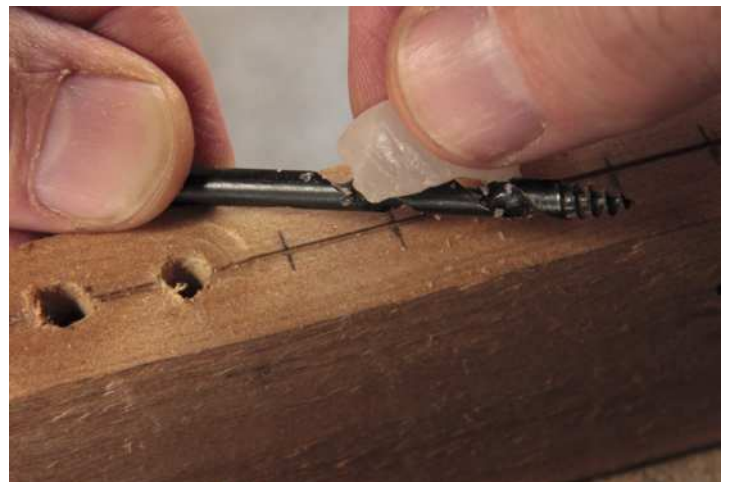
Squaring up the wood for the gimlet caddy (left) with a Stanley 9 1/2 block plane (left), then waxing the gimlet (above) to reduce friction
