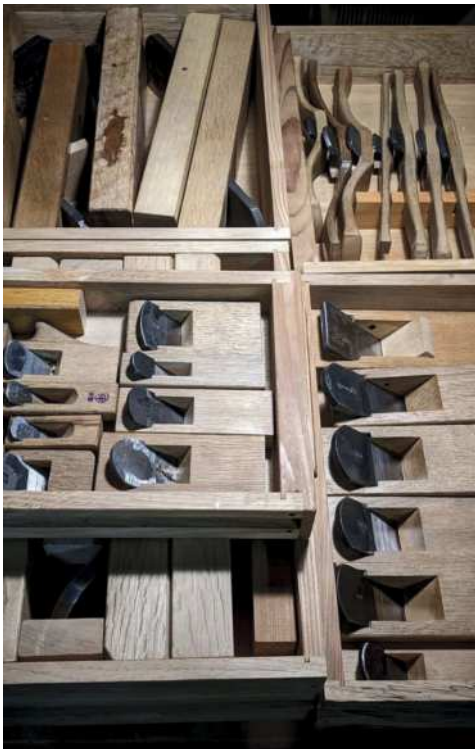
The Kanna (hand planes) Aoki uses to shape and finish his work (above). The various shapes and curvatures in the design mean numerous Kanna are needed, each shaped to create a specific shape or curvature. On top of that, separate Kanna are used for the rough shaping work and the fine finishing work. Many of the Kanna Dai (hand plane body) are made by him to achieve the ideal shape
