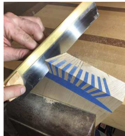
Initial layout drawing of the dovetail (above) and cutting down the sides of the rays (below), just touching the tape
