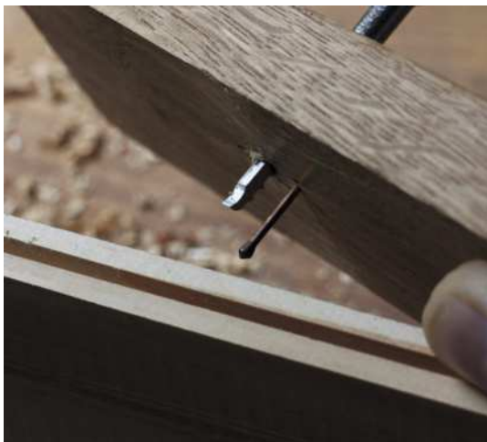
This shows the temporary panel pin fence (above) used in the early stages of grooving the guard
