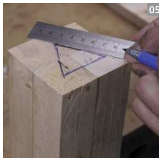
Putting one simple triangle (above, left) on the top is simpler than marking several on the faces. The colour difference (above, right) from the dots makes it easy to pair the mating parts
