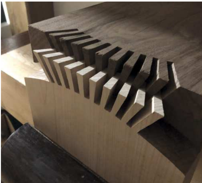
Chiselling out the curved shoulder line (above) and a dry fit pushed together at 45°, before gluing up (below)
