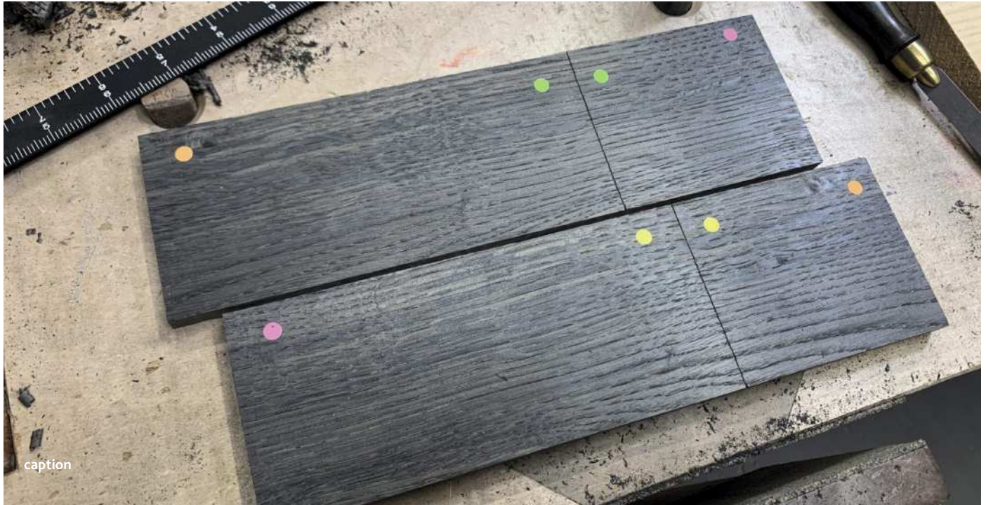
David Barron's coloured dot trick keeps the pieces organised (above). A Record 043 with custom wood fence (left). Making marks with my Philly Planes Superior Marking Gauge (below)
