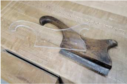
An acrylic template modelled after a 19th Century Weiss & Sohn Austrian Gratsäge (above) and an acrylic template showing the depth of the sawplate into the handle
