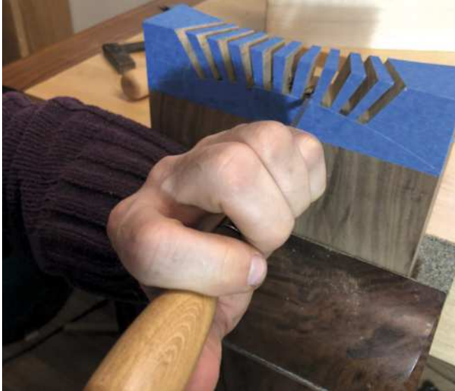
Chiselling out the curved shoulder line (above) and a dry fit pushed together at 45°, before gluing up (below)
