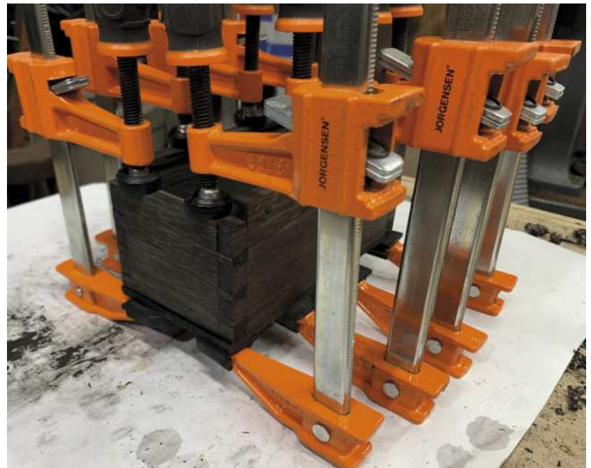
Transferring to the pin board using Ethan's dovetail transfer board (above). Clamping the sides (top right) and checking for square, then clamping the bottom to the sides (right)
