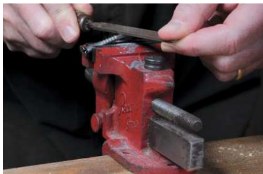
Filing the screw to shape in the Record Imp vice (above), to form the cutter shape (left) after filing but before honing
