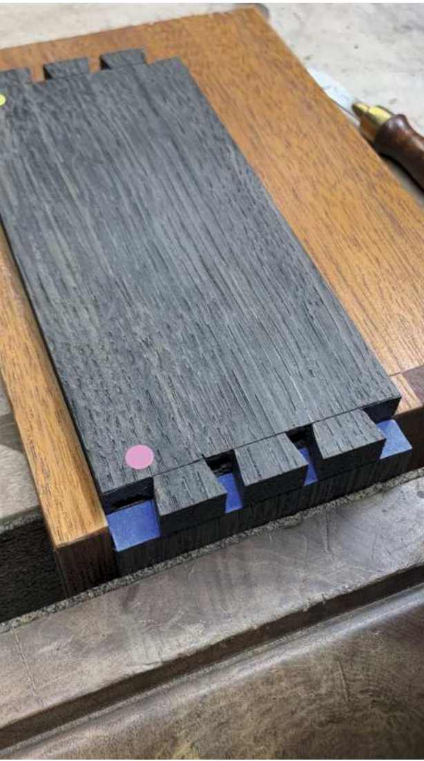
Transferring to the pin board using Ethan's dovetail transfer board (above). Clamping the sides (top right) and checking for square, then clamping the bottom to the sides (right)
