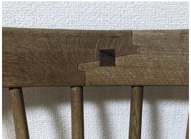
Details of the joinery on the backrest on the Riki Watanabe chair (above). The joinery used on the backrest made the chair irresistible and inspired Takuya to use a similar approach for his chair
