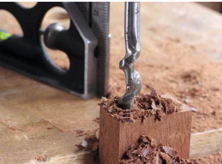
Checking for vertical with a combination square (left) and chamfering the corners (above) to stop splintering
