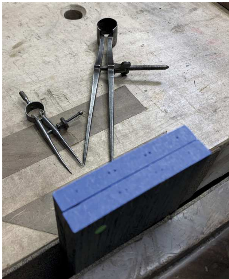
Cutting tails with the author's Bontz Saw Works dovetail saw with bog oak handle (above). Marking out dovetails with two sets of dividers (below) and removing waste with his Knew Concepts fret saw (left)
