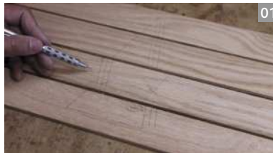
If any lines are misaligned (above), one or more of the parts have been incorrectly assembled. Add lines (right) or make the triangles different when marking similar assemblies
