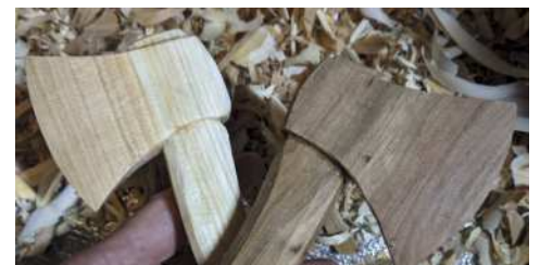
Kaylyn Messer (above) and apple and wild cherry wedge billets (above left) prepared for carving axe spreaders. Lots of stop cuts are recommended for removing material
