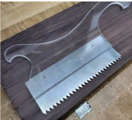
An acrylic template modelled after a 19th Century Weiss & Sohn Austrian Gratsäge (above) and an acrylic template showing the depth of the sawplate into the handle
