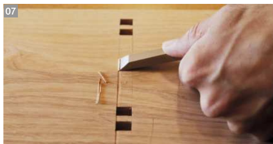
Begin defining the groove by chiselling a step against the knife mark (above) then define the walls of the groove with a chisel and mallet (right) before using a router plane (left) to remove the waste, leaving a flat bottom
