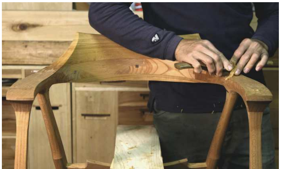
The Kanna (hand planes) Aoki uses to shape and finish his work (above). The various shapes and curvatures in the design mean numerous Kanna are needed, each shaped to create a specific shape or curvature. On top of that, separate Kanna are used for the rough shaping work and the fine finishing work. Many of the Kanna Dai (hand plane body) are made by him to achieve the ideal shape
