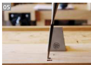
A visual reference is used to do the sloped cuts across the grain (above), with a small square a useful reference for plumb cuts (above right). Secure the square with tape if necessary
