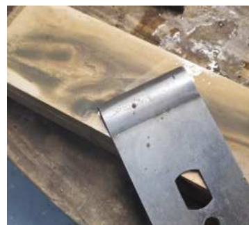
Finalising the fit for the brass nut (left) and honing the edge of the chip breaker
