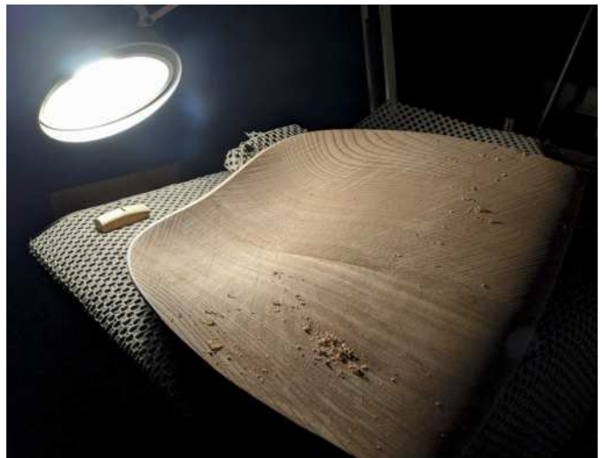
The fine-textured seat (above) is finished using a Shiho Sori Kanna (compass plane) seen on the far left. The light stand is the sole source of light in the dark. Moving the light around and shining light from various angles creates shadows showing the subtle details of the texture
