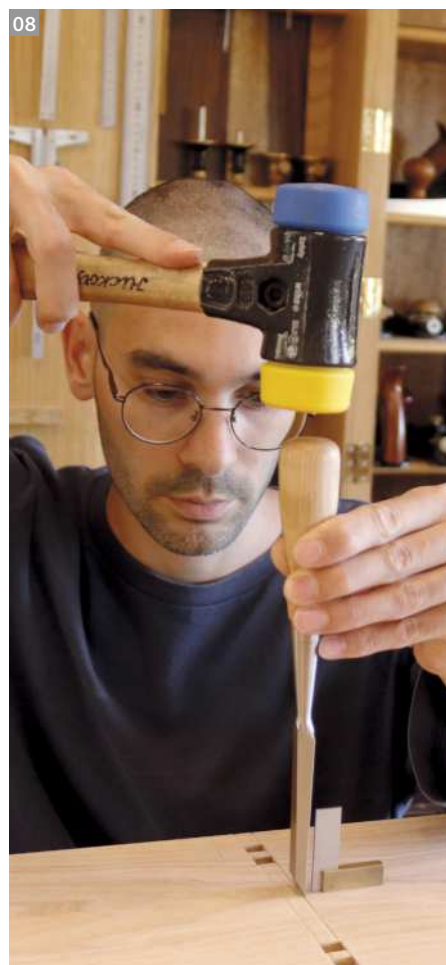
Using the spacer blocks to mark up the joint (left) and tidy marking of the mortises will result in much neater work (above)
