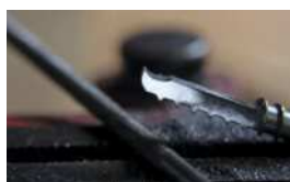
Filing the screw to shape in the Record Imp vice (above), to form the cutter shape (left) after filing but before honing
