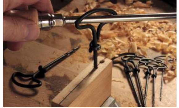
A screwdriver through the loop handle has increased leverage (right) in the production of the gimlet caddy (left)
