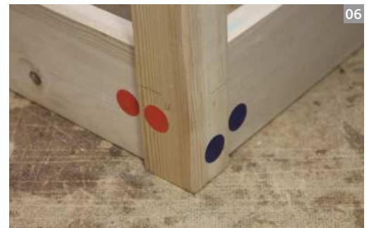
Putting one simple triangle (above, left) on the top is simpler than marking several on the faces. The colour difference (above, right) from the dots makes it easy to pair the mating parts
