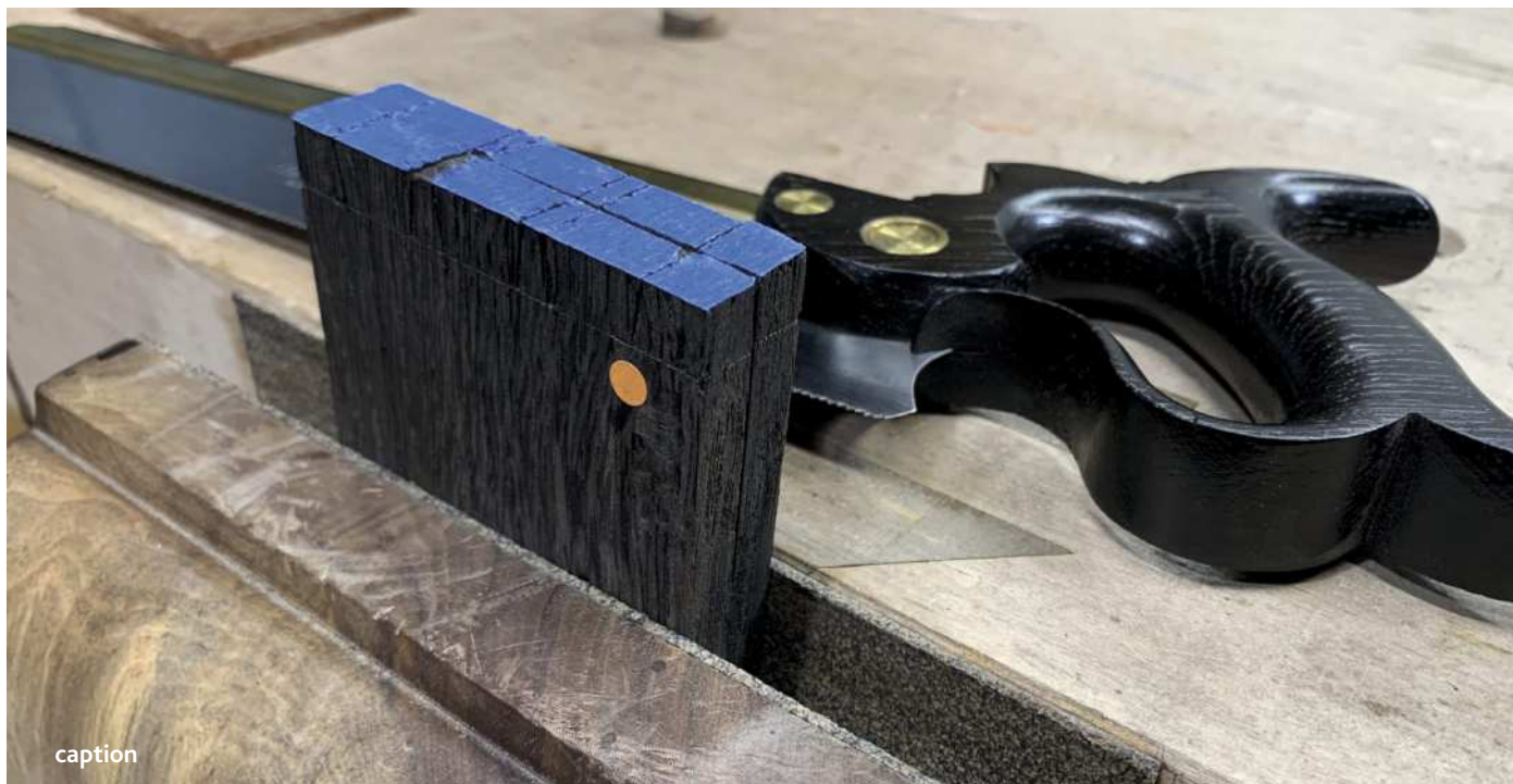
Cutting tails with the author's Bontz Saw Works dovetail saw with bog oak handle (above). Marking out dovetails with two sets of dividers (below) and removing waste with his Knew Concepts fret saw (left)
