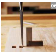
A visual reference is used to do the sloped cuts across the grain (above), with a small square a useful reference for plumb cuts (above right). Secure the square with tape if necessary
