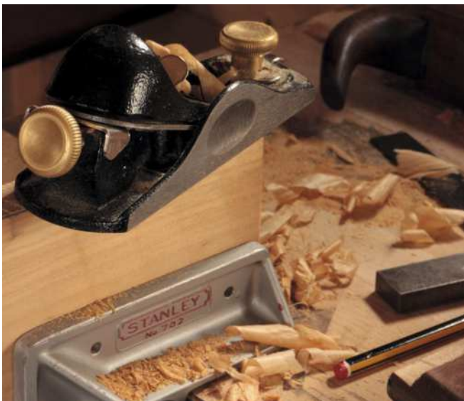
Squaring up the wood for the gimlet caddy (left) with a Stanley 9 1/2 block plane (left), then waxing the gimlet (above) to reduce friction
