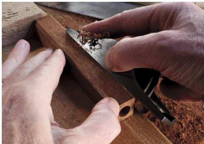
Checking for vertical with a combination square (left) and chamfering the corners (above) to stop splintering
