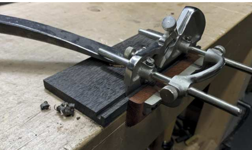
David Barron's coloured dot trick keeps the pieces organised (above). A Record 043 with custom wood fence (left). Making marks with my Philly Planes Superior Marking Gauge (below)
