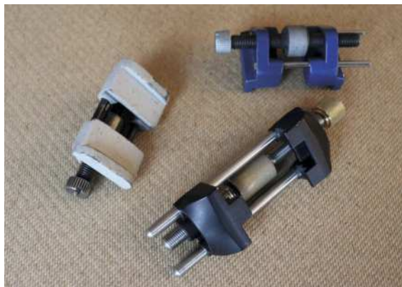
At £33 the new Veritas Side-Clamping Honing Guide is good value considering its versatility, especially the ease of holding chisels effectively. It is far better than an Eclipse clone (left, dark blue), but the original Eclipse is hard to beat for its simplicity. That said the vintage Eclipse shown here cost us £26. There are an upper (above left) and lower (above right) locations for blades on the Veritas to account for different lengths & thicknesses of iron
