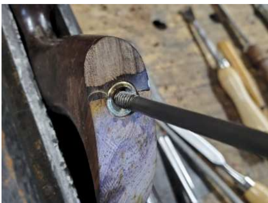
Carving the top of the tote (above) and drilling with a 3/16in bit (right)
