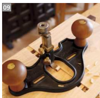
Begin defining the groove by chiselling a step against the knife mark (above) then define the walls of the groove with a chisel and mallet (right) before using a router plane (left) to remove the waste, leaving a flat bottom
