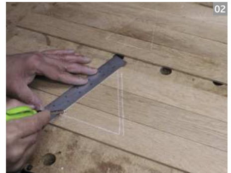
If any lines are misaligned (above), one or more of the parts have been incorrectly assembled. Add lines (right) or make the triangles different when marking similar assemblies
