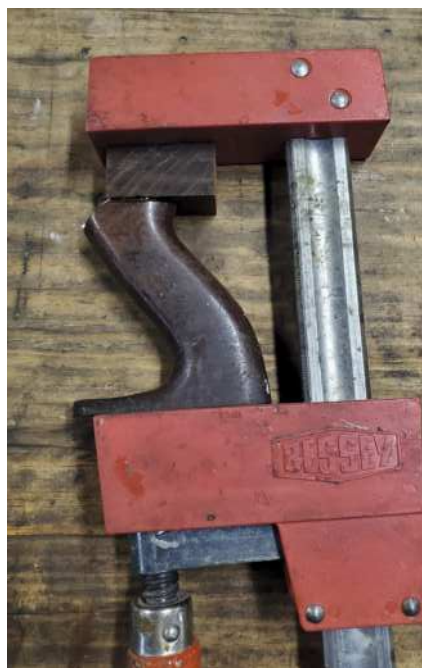
Gluing a new piece of wood on the tote (left) and home-made antique oil (above)
