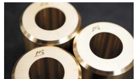
Engraving (above) is done the traditional way with a manual pantograph engraving machine. Matthias uses premium types of metal, from brass to titanium and German silver
