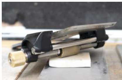
At £33 the new Veritas Side-Clamping Honing Guide is good value considering its versatility, especially the ease of holding chisels effectively. It is far better than an Eclipse clone (left, dark blue), but the original Eclipse is hard to beat for its simplicity. That said the vintage Eclipse shown here cost us £26. There are an upper (above left) and lower (above right) locations for blades on the Veritas to account for different lengths & thicknesses of iron
