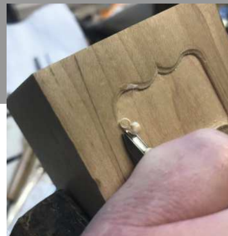
Carving the cove in a recessed Cupid's Bow (above). The English and Dutch styles are inspired by David Snicker's work. A York pitch double iron coffin smoother with hand-carved Fleur-de-lis (left)
