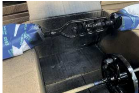
The drive gear and body receive coats of black paint (above). Multiple lighter coats go on easier and look better than one heavy coat (below left). The author's custom 5/16in bearing assembly for the spindle pocket (below)
