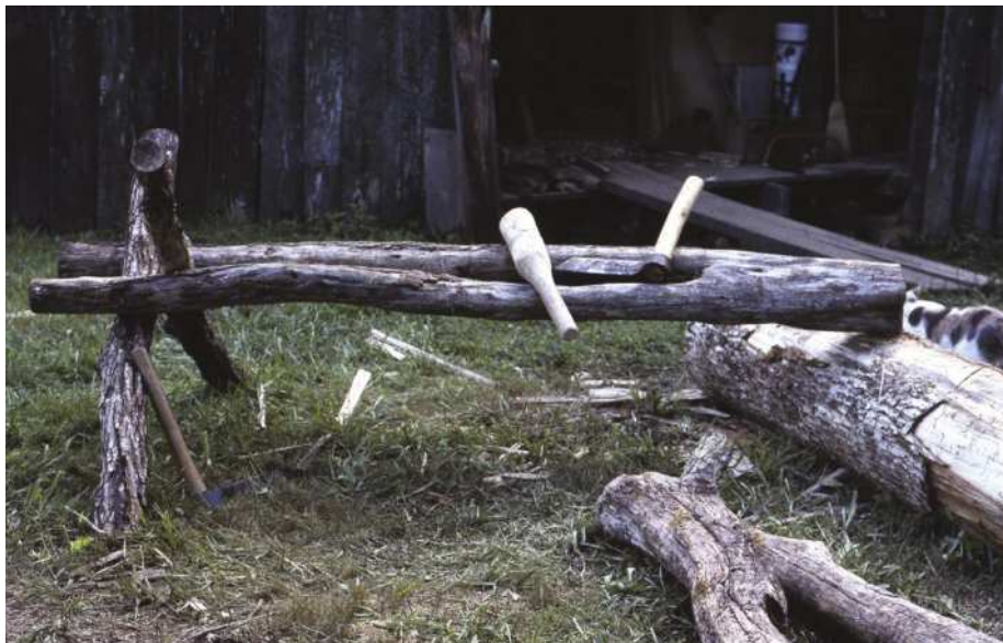
The natural crotch-based riving brake (above, Pic.1) and one built using dimensional lumber (right, Pic.2)
