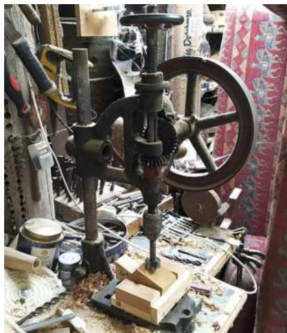
David used his Mancuna pillar drill (above) for accurate drilling of the seat holes
