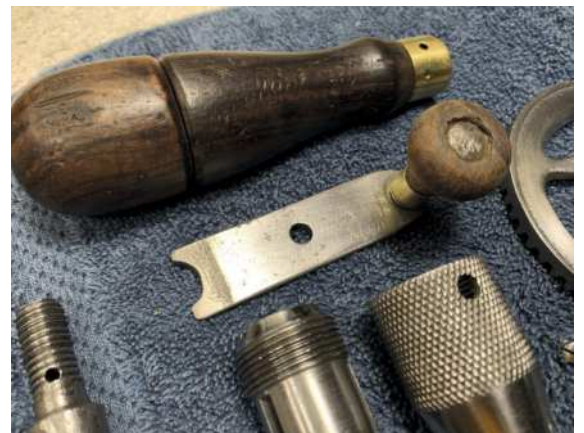
The partially disassembled drill and the tools of the trade (above) and the main handle and crank handle after cleaning (below). The drive wheel after cleaning (bottom) and the parts of the chuck all polished up (below left). The cleaned and disassembled drill (above left)
