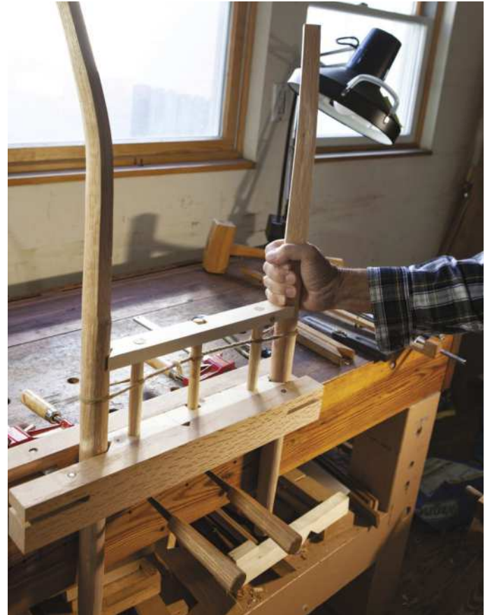
Adjusting the flare of the rear posts (Pic.9, above), which are held in the posts holder, which is in turn held by a double bench clamp. Note the vertical V-notch in the centre of the clamp's front jaw to hold posts vertical for layout). The V-blocks in use (below, Pic.10). Note that the back post is inserted so that all three mortises can be drilled without repositioning the workpiece
