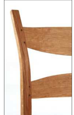
Detail of the slats/posts (above). The flat, or relief, shaved on the rear post makes it easier to bend and more comfortable for the sitter than a fully-rounded post. Big and heavy, this shaving horse (below) made made using a ‘found’ narrow plank was influenced by an old photo of a British shaving horse
