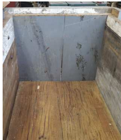
The bottom (above) has swelled, forcing a seam to open in each end
