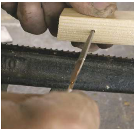
A saw vice (Pic.4, above) holding a 6tpi blade. A file guide can be as simple as a block of wood (Pic.5, left), with a hole to hold the file. Once you have the right angle set the block so that its top surface is parallel with the bench
