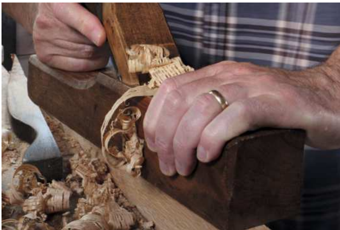
Straightening out a rip-sawn edge with a 14in Emir raze jack plane (above), and final planing of reclaimed oak (right) with an Edward Preston coffin smoother
