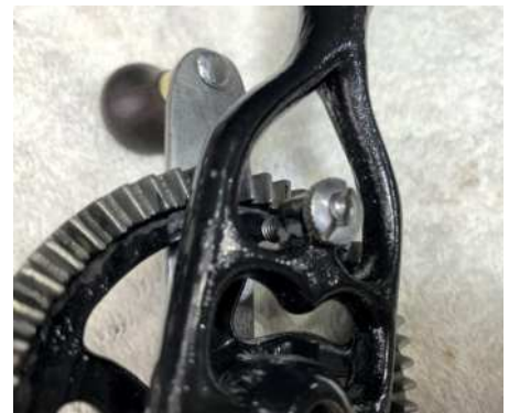
The toaster oven (left) backing a new Rustoleum black finish. The adjustable bearing of the No.1 hand drill (below). The McCoy's springless chuck, polished and fully re-assembled (below left)
