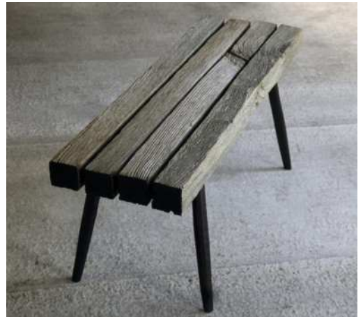
Alex has a choice of materials to use for his bowls and benches, but it is all reclaimed or recycled or harvested from storm-fallen trees. Old field fencing, often oak in reasonable condition beneath the surface, makes an excellent resource for bench tops (above) and you can even see the mortises for rails left on his chopping boards (left). He also scorches ash from Dieback victims
