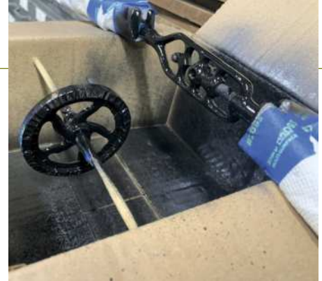
The drive gear and body receive coats of black paint (above). Multiple lighter coats go on easier and look better than one heavy coat (below left). The author's custom 5/16in bearing assembly for the spindle pocket (below)
