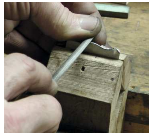
Some mouldings take more than one cutter to achieve the desired finial shape required (above). Once the tape with the profile drawn on it is placed on the metal, it is a simple matter of filing down to the line to make the cutter (right)
