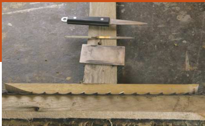
The blade clamped to the front of a bench (Pic.2, above), with the diamond options for filing. The bright, abraded back of teeth (Pic.3, below)
