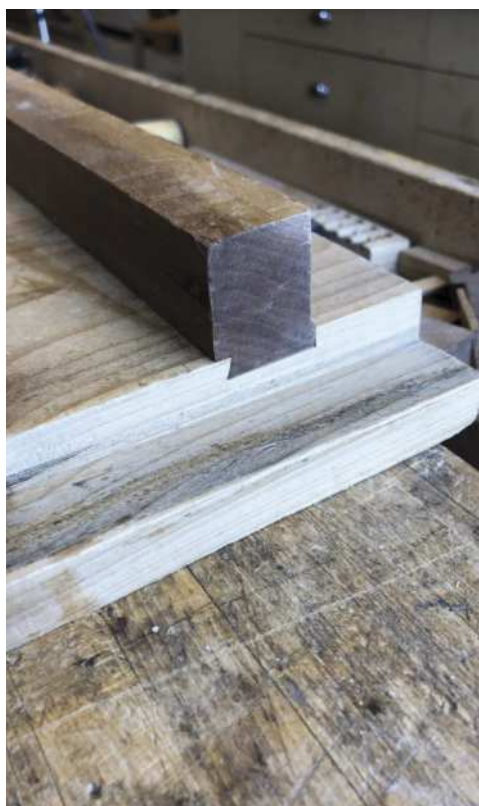
Scott Wynn uses a sliding dovetail for the stop so that it can be adjusted and a new end worked to rectify frequent damage. The straight side of the sliding dovetail is at the rear of the stop (left, Pic.1)
