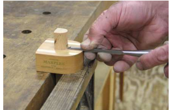
Leveling the mortise with a narrow chisel (above)
