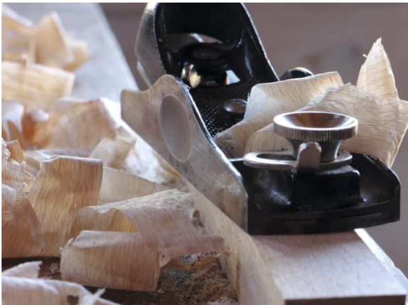
Straightening out a rip-sawn edge with a 14in Emir raze jack plane (above), and final planing of reclaimed oak (right) with an Edward Preston coffin smoother
