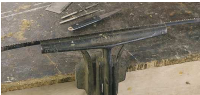
A saw vice (Pic.4, above) holding a 6tpi blade. A file guide can be as simple as a block of wood (Pic.5, left), with a hole to hold the file. Once you have the right angle set the block so that its top surface is parallel with the bench
