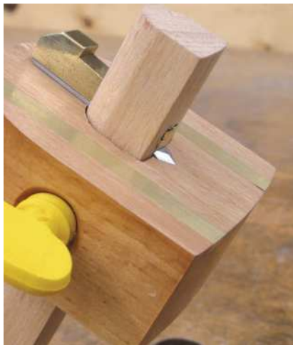
If necessary shorten the brass wedge (above) after fine tuning the mortise. The blade's bevels can be reversed (below), but should always face the waste of a cut
