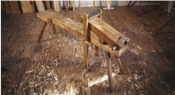
This version (above, Pic.5) of the shaving horse gave me everything I needed. Most important of all is the ease of adjustment. Two notches do it all in this jig (below, Pic.6), the 'notched wooden bench hook', for cutting stock to length
