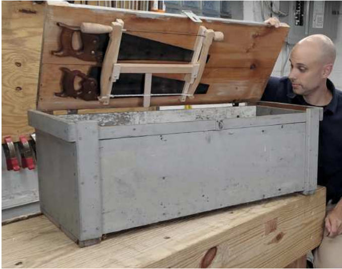
The bottom (above) has swelled, forcing a seam to open in each end
