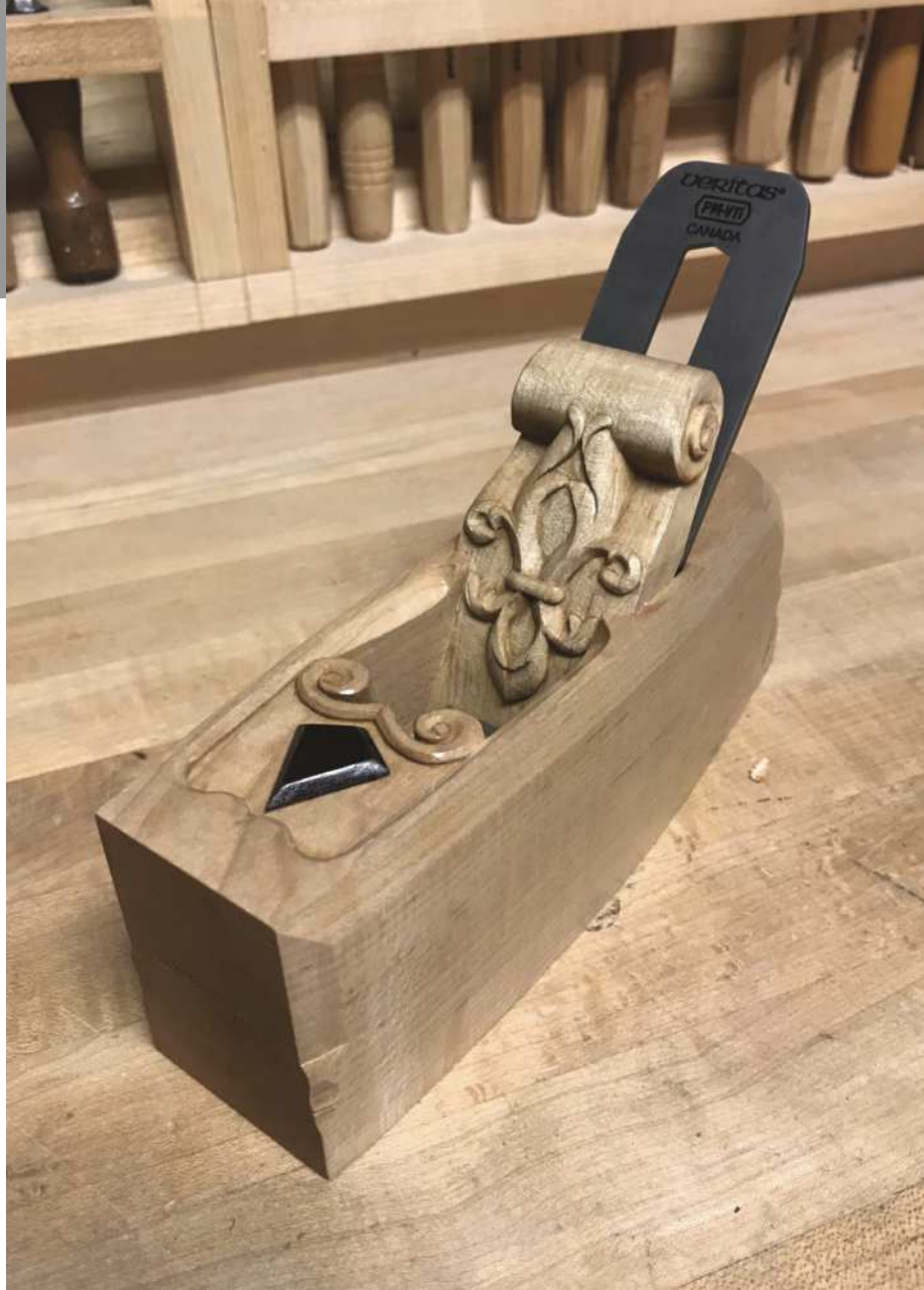
Carving the cove in a recessed Cupid's Bow (above). The English and Dutch styles are inspired by David Snicker's work. A York pitch double iron coffin smoother with hand-carved Fleur-de-lis (left)
