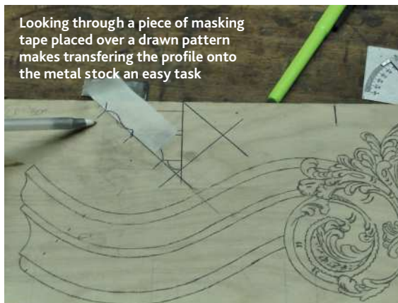
Some mouldings take more than one cutter to achieve the desired finial shape required (above). Once the tape with the profile drawn on it is placed on the metal, it is a simple matter of filing down to the line to make the cutter (right)
