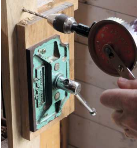
Turned at 90°, the vice exerts grip on wood held vertically (above). The fixed jaw lining meets the edge of the bench (below) and overlaps the leg
