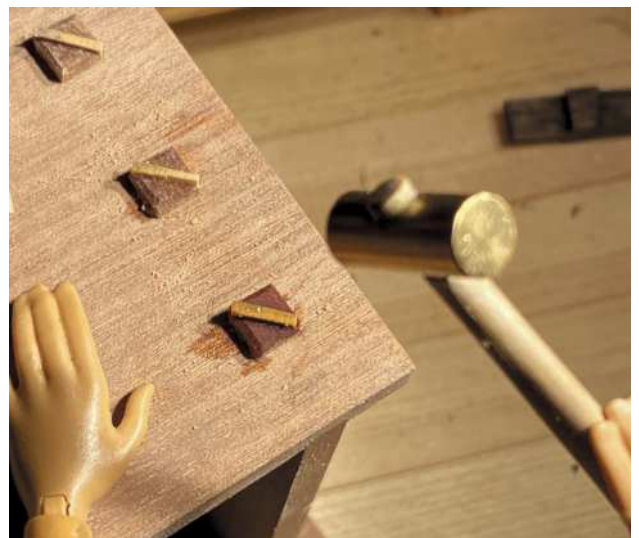
Chopping out of the waste from the through mortises (left). "I love my new wooden plane," the author says.
