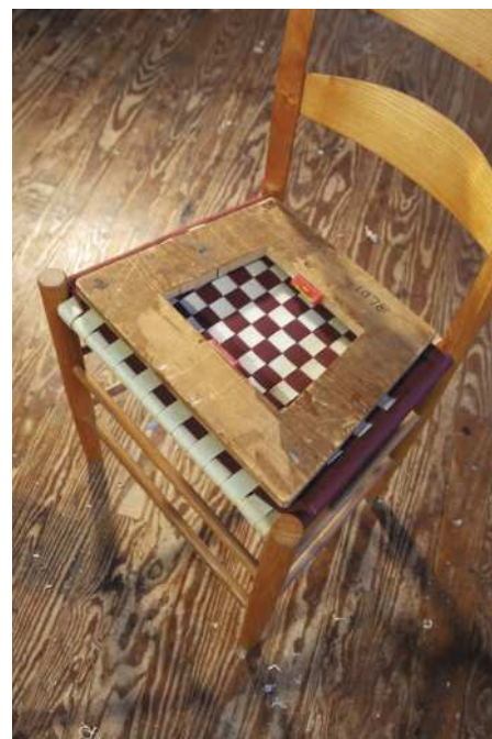
The seat plan in use. Like the centre finder, accuracy when making it is critical
