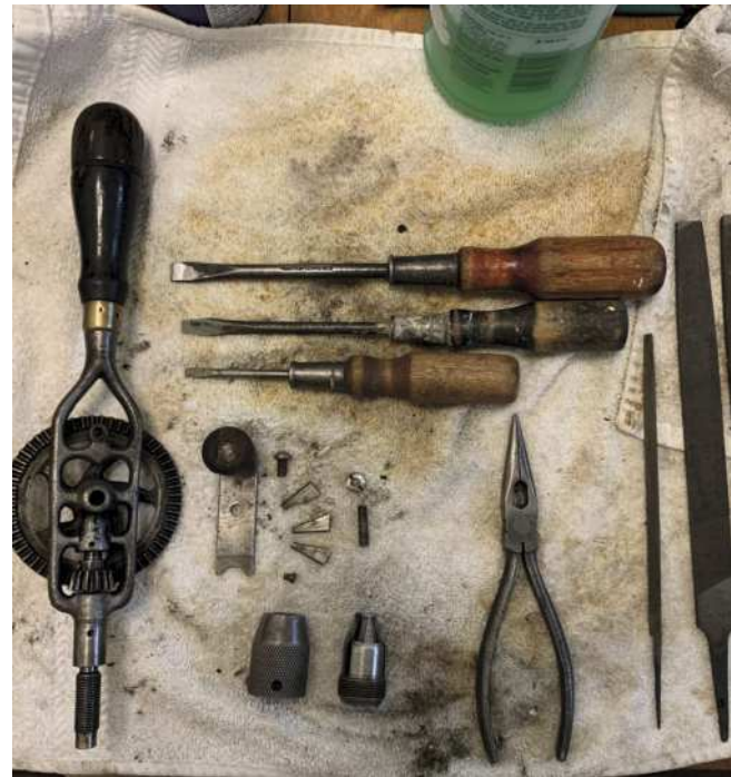
The partially disassembled drill and the tools of the trade (above) and the main handle and crank handle after cleaning (below). The drive wheel after cleaning (bottom) and the parts of the chuck all polished up (below left). The cleaned and disassembled drill (above left)
