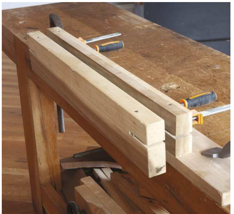
Peter Follansbee uses a riving brake (above, Pic.3) as a large tripod with cross pieces bolted to the front legs. The 'double bench clamp' (below, Pic.4)) used by Mike Siemsen is similar to the one described here, but with 24 \frac{1}{8} in (instead of 10in) between the posts so that it can accommodate casework
