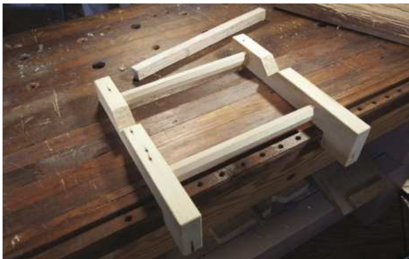
This version (above, Pic.5) of the shaving horse gave me everything I needed. Most important of all is the ease of adjustment. Two notches do it all in this jig (below, Pic.6), the 'notched wooden bench hook', for cutting stock to length
