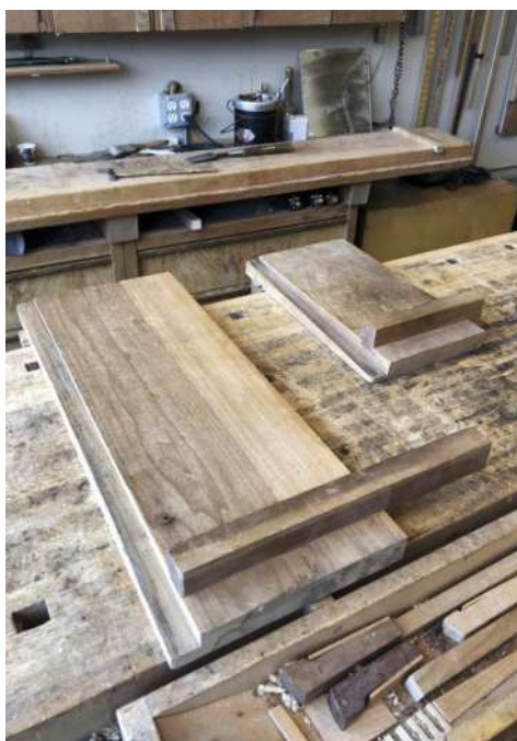
Scott Wynn uses a sliding dovetail for the stop so that it can be adjusted and a new end worked to rectify frequent damage. The straight side of the sliding dovetail is at the rear of the stop (left, Pic.1)
