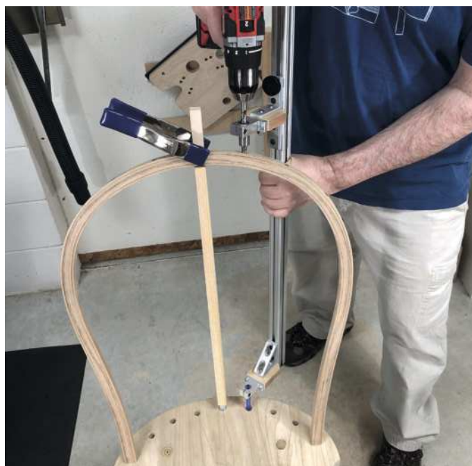
Using the Spindle Drilling Guide to drill the spindle mortise in the bow of a balloon back Windsor chair
