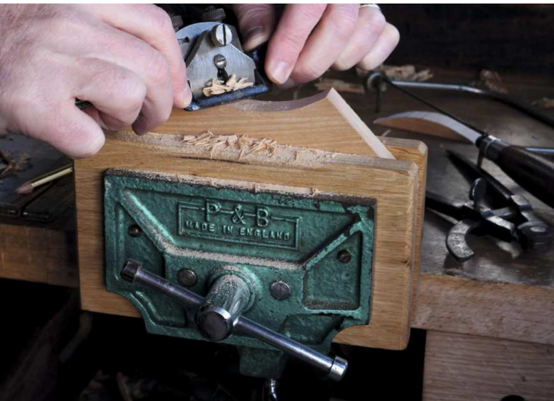
Using a spokeshave with a Parry & Bott table vice mounted as designed (left) and an early experiment (above) with the Rabone Chesterman vice at 90°
