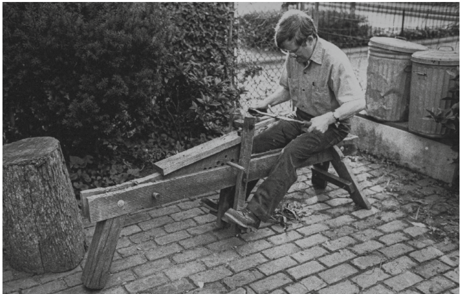
Detail of the slats/posts (above). The flat, or relief, shaved on the rear post makes it easier to bend and more comfortable for the sitter than a fully-rounded post. Big and heavy, this shaving horse (below) made made using a ‘found’ narrow plank was influenced by an old photo of a British shaving horse
