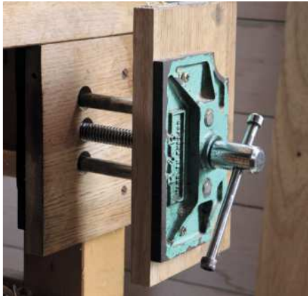
Turned at 90°, the vice exerts grip on wood held vertically (above). The fixed jaw lining meets the edge of the bench (below) and overlaps the leg
