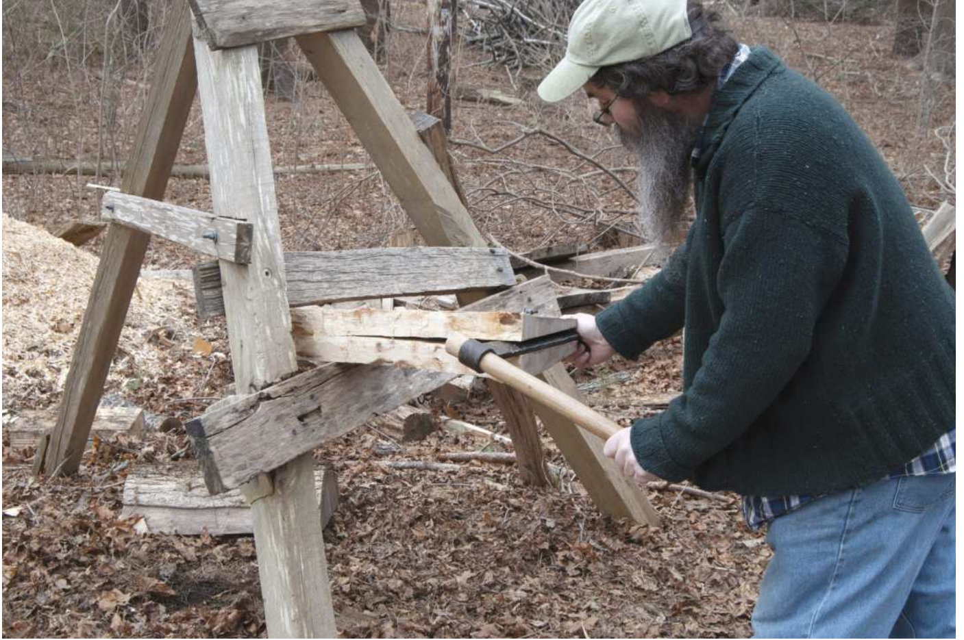
Peter Follansbee uses a riving brake (above, Pic.3) as a large tripod with cross pieces bolted to the front legs. The 'double bench clamp' (below, Pic.4)) used by Mike Siemsen is similar to the one described here, but with 24 \frac{1}{8} in (instead of 10in) between the posts so that it can accommodate casework
