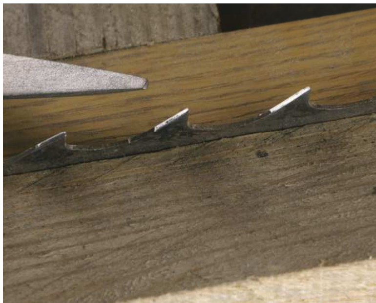
The blade clamped to the front of a bench (Pic.2, above), with the diamond options for filing. The bright, abraded back of teeth (Pic.3, below)
