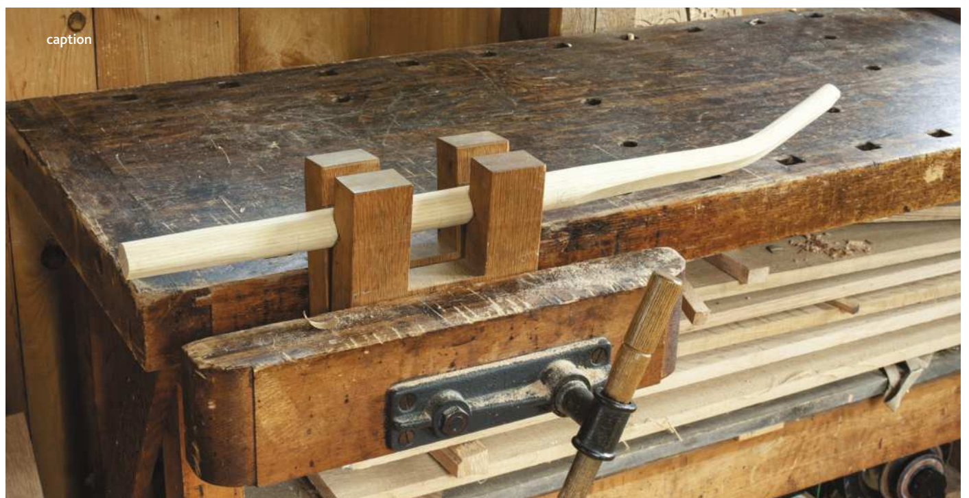
Adjusting the flare of the rear posts (Pic.9, above), which are held in the posts holder, which is in turn held by a double bench clamp. Note the vertical V-notch in the centre of the clamp's front jaw to hold posts vertical for layout). The V-blocks in use (below, Pic.10). Note that the back post is inserted so that all three mortises can be drilled without repositioning the workpiece
