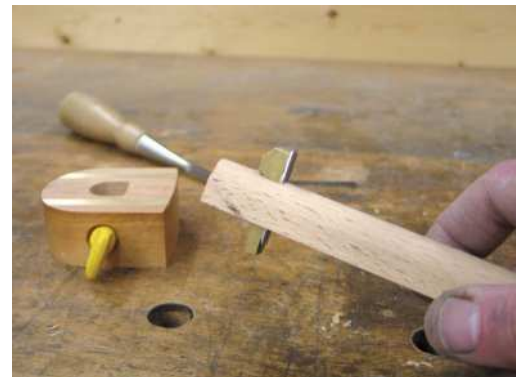
If necessary shorten the brass wedge (above) after fine tuning the mortise. The blade's bevels can be reversed (below), but should always face the waste of a cut
