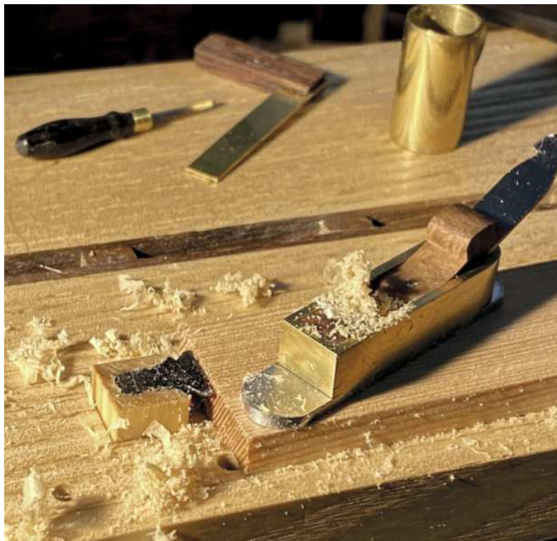
A planing stop (above) is a good introduction to blacksmithing. It can be made from mild steel. Once the end has been flared, the stop can be decorated (left) with files.
