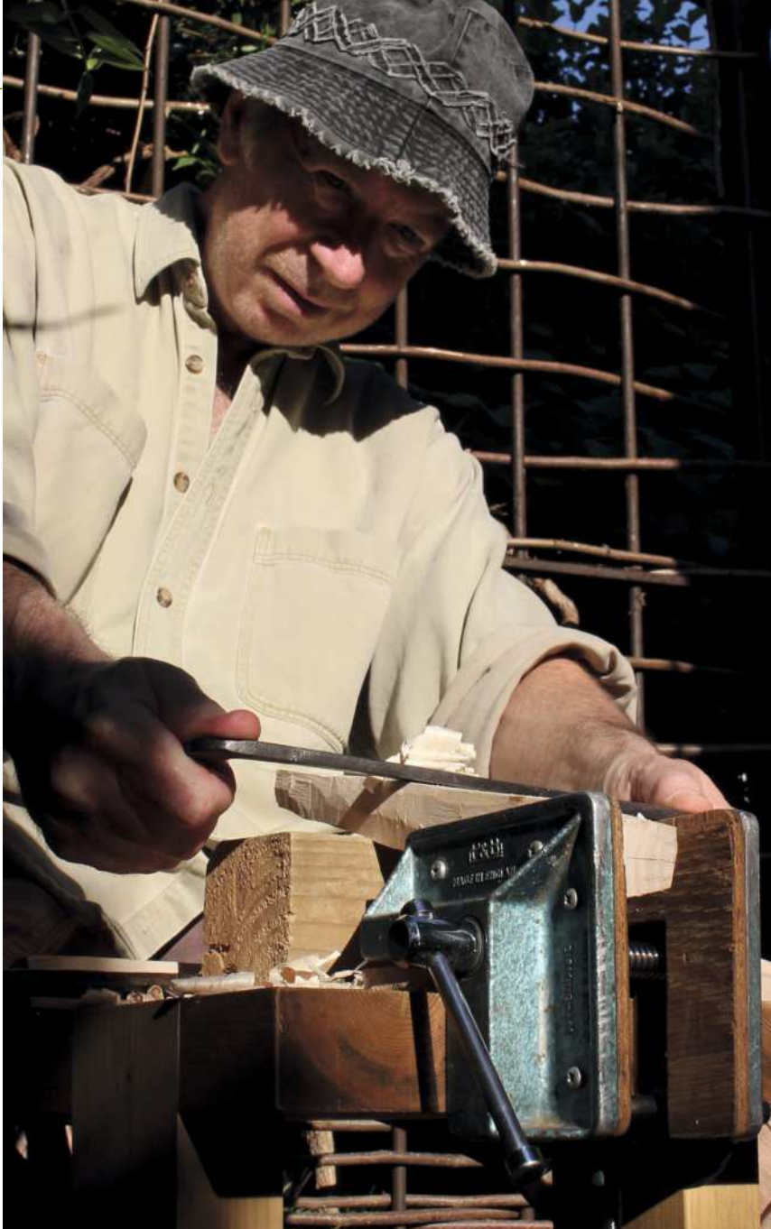
The straight-legged saw bench featured in QM02 becomes a shaving horse with a corner vice (left). The peg is locked in the vice (above) with a wedge and supported by a block
