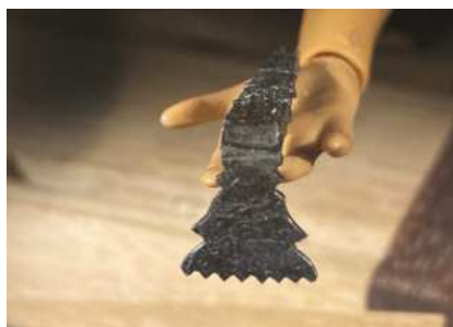
A planing stop (above) is a good introduction to blacksmithing. It can be made from mild steel. Once the end has been flared, the stop can be decorated (left) with files.
