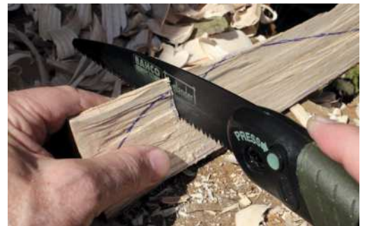
A single cut establishes the beak of the notch (above) and a short knife (right) is used for controlled chamfering around the notch
