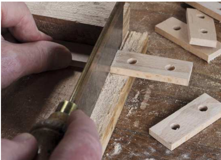
Ripping the block of six tensioners into three pairs (above). Separating pairs of tensioners on the bench hook we featured in QM?? (below) before making hollows for the fingers with a convex file (below right)
