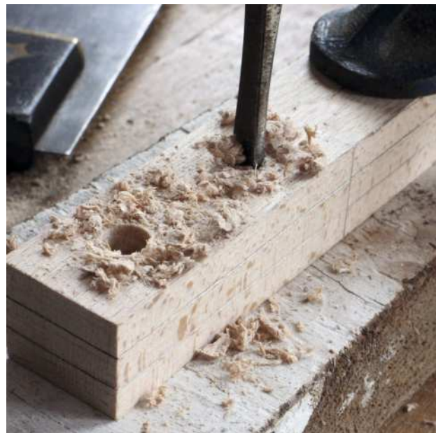
The cleft ash tent peg with a beech tensioner and natural fibre guy rope (left). Marking the block for a tensioner (above) and boring rope holes with a brace and bit
