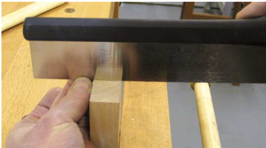
By pinching with the thumb and index finger you get better control at the start, but beware the risks of injury
