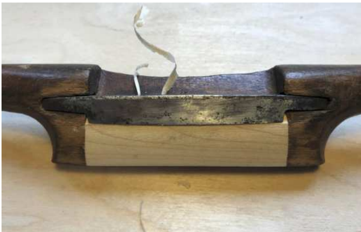
This old wooden spokeshave costing £3 has seen a great deal of use, so it's not surprising that the wood has worn (above left). Having cut and pared away the waste, and inserted a maple wear strip (left), Debs had more power in her elbow and sweet shavings from a happy tool (above)
