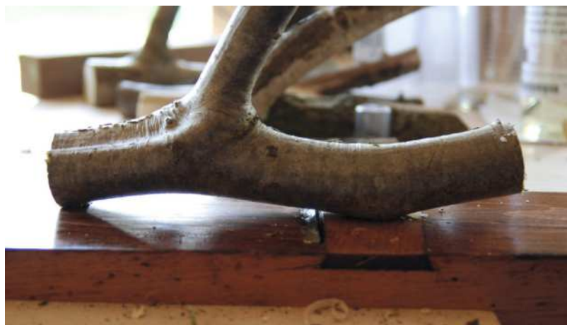
Flattening the back of the hook on a plane fixed in a vice, always working with the grain, this way and that
