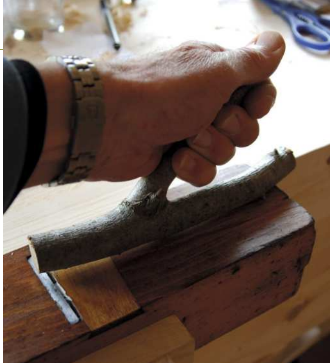
Flattening the back of the hook on a plane fixed in a vice, always working with the grain, this way and that
