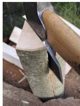
Hewing close to the final shape of the peg with an axe (left). Cross-cutting 5in ash with a Laplander folding saw was hot work (below). The circular log is split (right) to produce eight peg blanks (above)
