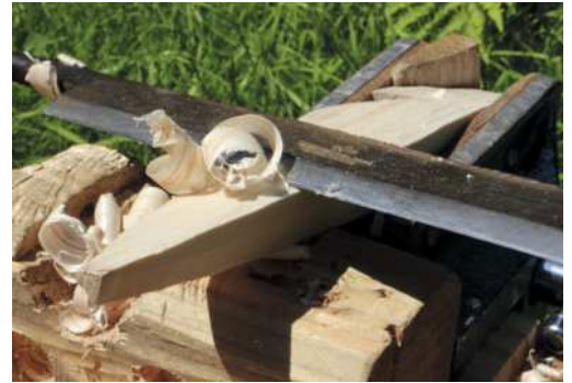
The straight-legged saw bench featured in QM02 becomes a shaving horse with a corner vice (left). The peg is locked in the vice (above) with a wedge and supported by a block
