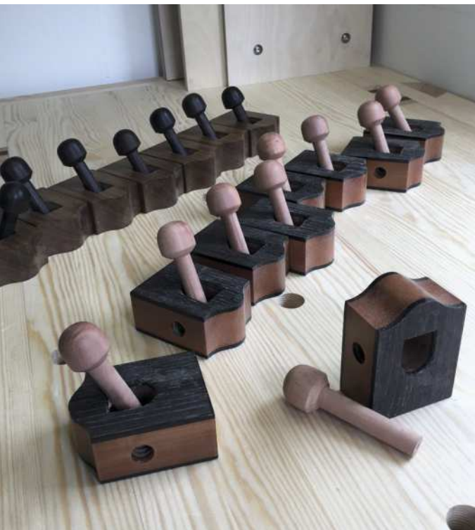
An early batch of pear and bog oak pin gauge stocks (left) and tapping the thread in the gauge stocks for the screw (above). The shape of the stocks (above right) is partly created by drilling with a large Forstner bit. The top part of the shape is roughed out with a rasp (right)
