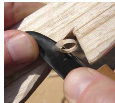
A single cut establishes the beak of the notch (above) and a short knife (right) is used for controlled chamfering around the notch
