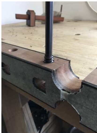
An early batch of pear and bog oak pin gauge stocks (left) and tapping the thread in the gauge stocks for the screw (above). The shape of the stocks (above right) is partly created by drilling with a large Forstner bit. The top part of the shape is roughed out with a rasp (right)
