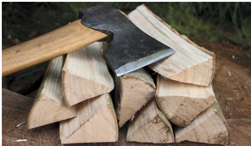
Hewing close to the final shape of the peg with an axe (left). Cross-cutting 5in ash with a Laplander folding saw was hot work (below). The circular log is split (right) to produce eight peg blanks (above)
