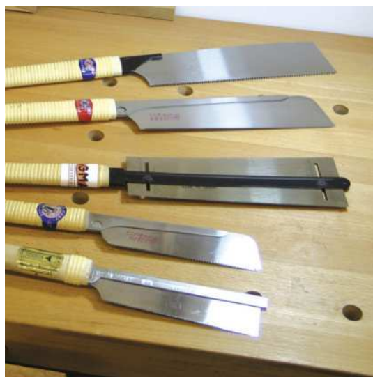
Various styles of Japanese saw. The double-edged ryoba (centre) has rip and crosscut teeth, and a depth setting
