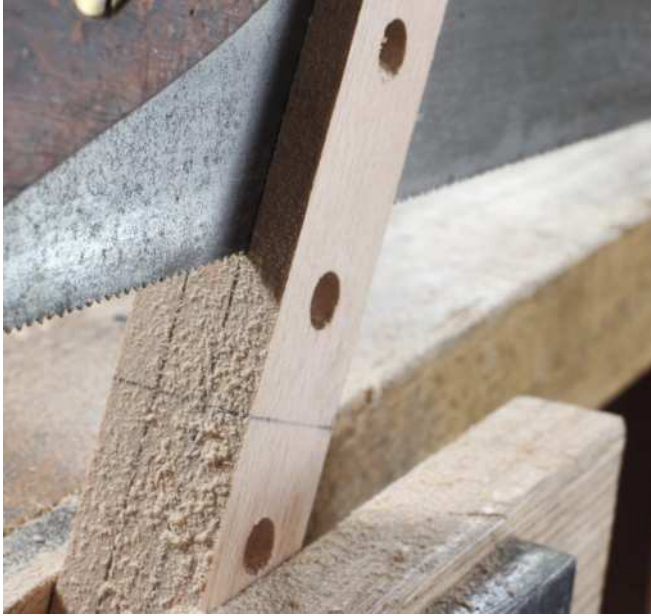
Ripping the block of six tensioners into three pairs (above). Separating pairs of tensioners on the bench hook we featured in QM?? (below) before making hollows for the fingers with a convex file (below right)
