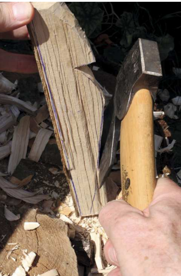
Hewing close to the final shape of the peg with an axe (left). Cross-cutting 5in ash with a Laplander folding saw was hot work (below). The circular log is split (right) to produce eight peg blanks (above)
