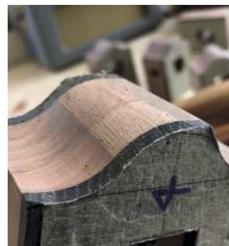
An early batch of pear and bog oak pin gauge stocks (left) and tapping the thread in the gauge stocks for the screw (above). The shape of the stocks (above right) is partly created by drilling with a large Forstner bit. The top part of the shape is roughed out with a rasp (right)
