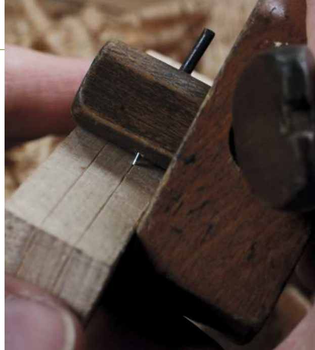
The cleft ash tent peg with a beech tensioner and natural fibre guy rope (left). Marking the block for a tensioner (above) and boring rope holes with a brace and bit
