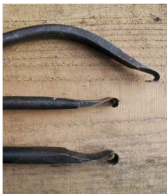
Seen from either side, and from top to bottom, are the crank tool, the finishing hook and the gouging hook. Mandrels with metal teeth (right)
