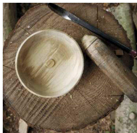
Preparing a bowl blank (left) and then on the lathe with the foot and outside turned (above). The cherry bowl detached (right) from the mandrel with a bottoming knife
