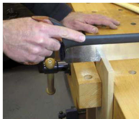
John extends his index finger for both Japanese and Western saws (above & below)
