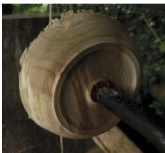
Preparing a bowl blank (left) and then on the lathe with the foot and outside turned (above). The cherry bowl detached (right) from the mandrel with a bottoming knife
