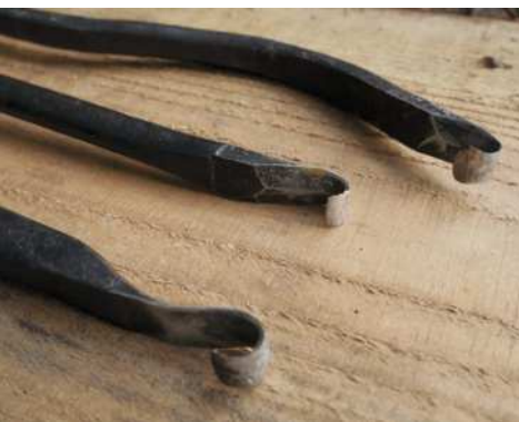
Seen from either side, and from top to bottom, are the crank tool, the finishing hook and the gouging hook. Mandrels with metal teeth (right)
