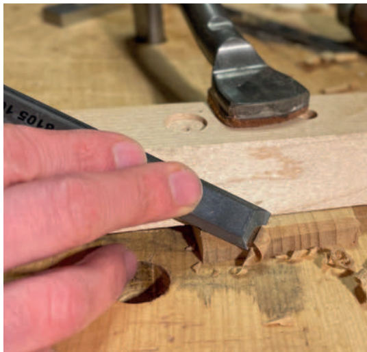
Christopher prefers scoring a line to using a pencil to mark up the mitres (above). Heavy cuts from the side with a skewed angle (right) making for quick work and no splinching
