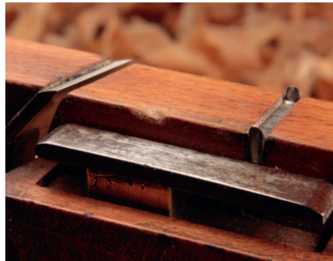
Cutting a drawer bottom groove with a newly restored grooving plane (above). Twin spurs preceding the iron score the surface fibres (left) of a dado, and the arrangement of spurs, iron and depth stop on the dado plane (below)
