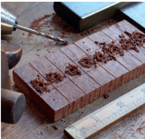
The 'mother piece' marked and drilled for eight door buttons (left). Carving textured wings (above) while the work is attached to the backing board. Sawing the buttons free (right) one by one on the bench hook
