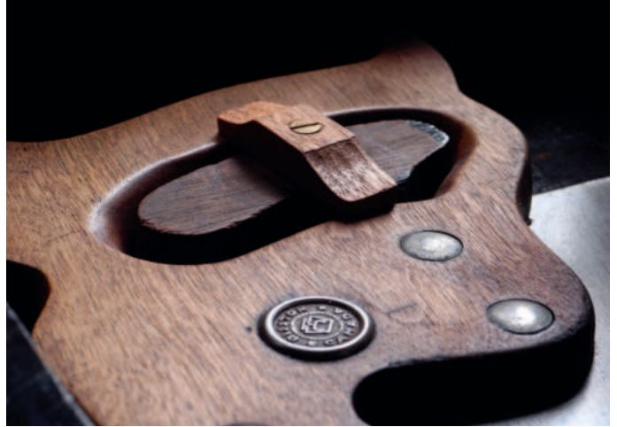
A panel saw secured by a button in the lid of a joiner's toolbox (above). A button (below) ready for fitting with the corners and edges rounded
