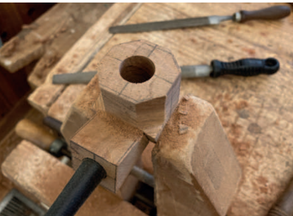
Steve uses five main tools (above left) for shaping a pipe: a large and small half-round rasp, a large and small half-round file, and a round file. Shaping the pipe (left) is just like shaping the stem's tenon. Steve begins by taking off the four corners to make an octagon. Then he takes off the remaining 16 corners to bring the shape close to round (above)
