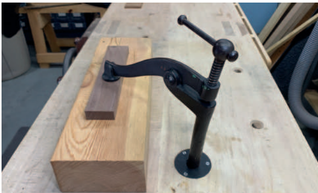
Ethan snagged his antique bench holdfast (above) from Patrick Leach a few years ago, so he can hold down a workpiece without the need for a noisy whack. But his favourite upgrade has been a brass disc (right) engraved by Jenny Bower
