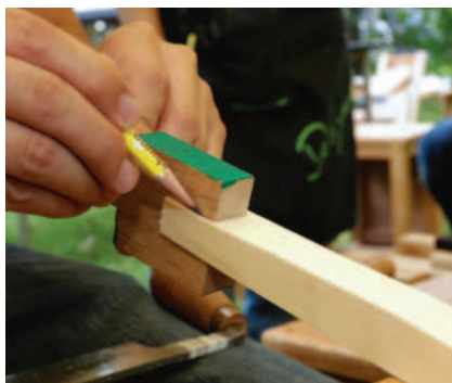
A special little jig (below left) was made to prepare tenons exactly 16x19mm for a squeeze fit into a 19mm diameter mortise (below right). Participants worked in pairs for drilling the frames (right)
