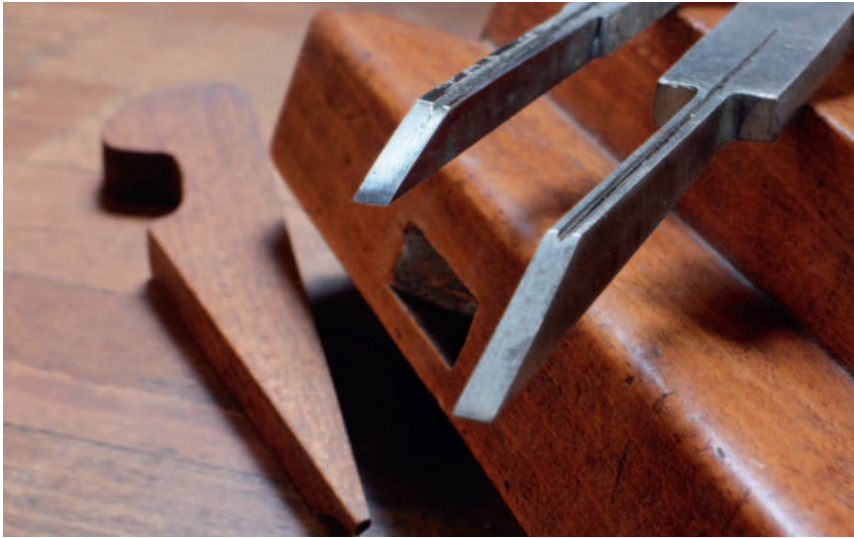
The replacement wedge stained with strong coffee to match the colour of the stock (above). The set of eight plough irons belonging to the Greenslade plane (below left). Grooving planes (below) with adjustable fence (left) and fixed fence (right)
