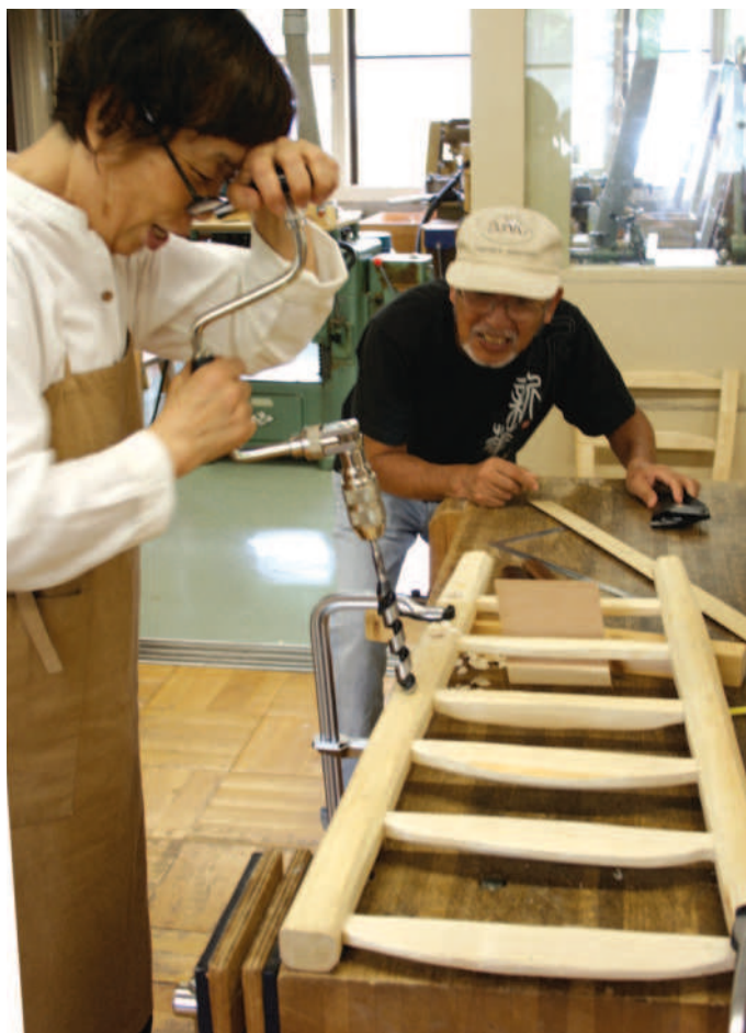
A special little jig (below left) was made to prepare tenons exactly 16x19mm for a squeeze fit into a 19mm diameter mortise (below right). Participants worked in pairs for drilling the frames (right)
