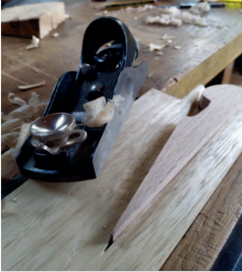
Supporting the wedge in its cradle while planing to thickness (above). The tip of the wedge is carved with a curiously skewed hollow (right). The iron of a wooden plough (on the right, below) is too wide for the grooving plane
