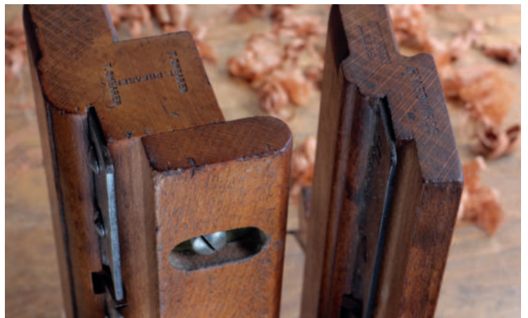
The replacement wedge stained with strong coffee to match the colour of the stock (above). The set of eight plough irons belonging to the Greenslade plane (below left). Grooving planes (below) with adjustable fence (left) and fixed fence (right)
