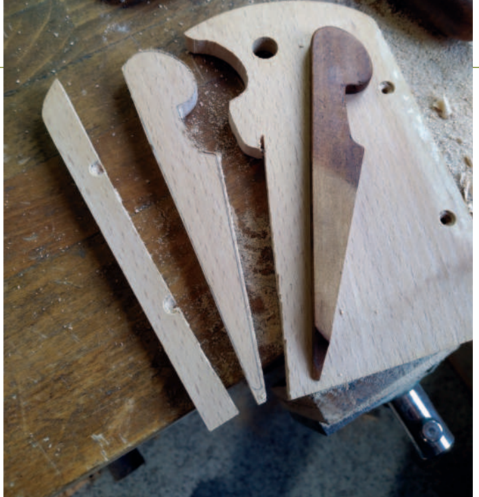
A contemporary wedge was used as the profile pattern for a replacement
