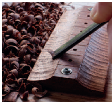
The 'mother piece' marked and drilled for eight door buttons (left). Carving textured wings (above) while the work is attached to the backing board. Sawing the buttons free (right) one by one on the bench hook
