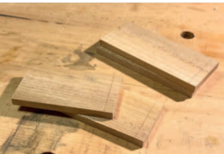
Christopher prefers scoring a line to using a pencil to mark up the mitres (above). Heavy cuts from the side with a skewed angle (right) making for quick work and no splinching
