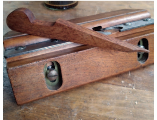
The replacement wedge stained with strong coffee to match the colour of the stock (above). The set of eight plough irons belonging to the Greenslade plane (below left). Grooving planes (below) with adjustable fence (left) and fixed fence (right)
