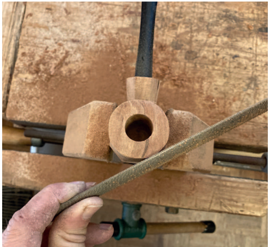
Steve uses five main tools (above left) for shaping a pipe: a large and small half-round rasp, a large and small half-round file, and a round file. Shaping the pipe (left) is just like shaping the stem's tenon. Steve begins by taking off the four corners to make an octagon. Then he takes off the remaining 16 corners to bring the shape close to round (above)
