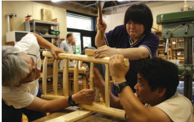
A square tenon into a round hole can be a tight fit, especially when the legs then shrink to hold the rung tenons even more tightly
