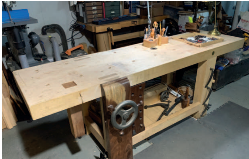
Ethan accidentally left the new workbench's planing stop at Plate 11, but it was easy to replace with a mahogany block (above). As well as a new Benchcrafted leg vise, The Kilted Woodworker added a stool to one side inspired by an antique cast iron swing-out seat (below) discovered on ebay ramblings and only needing a wooden seat
