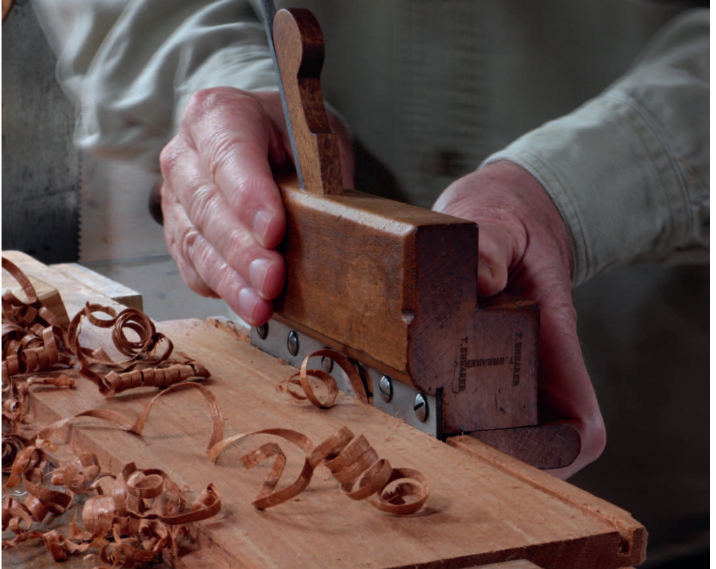
Cutting a drawer bottom groove with a newly restored grooving plane (above). Twin spurs preceding the iron score the surface fibres (left) of a dado, and the arrangement of spurs, iron and depth stop on the dado plane (below)
