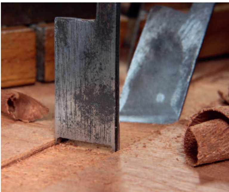
Cutting a drawer bottom groove with a newly restored grooving plane (above). Twin spurs preceding the iron score the surface fibres (left) of a dado, and the arrangement of spurs, iron and depth stop on the dado plane (below)
