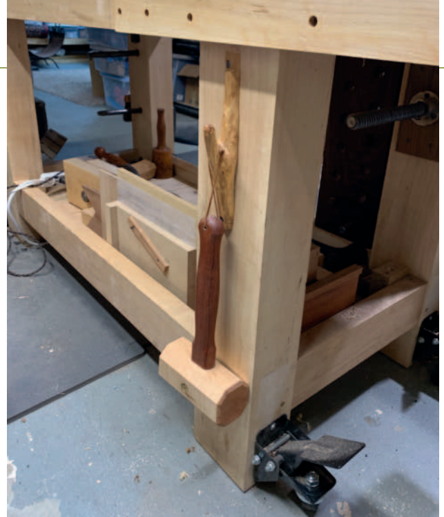
The most useful addition to the new bench was the light/small tool holder featured in QM04 (left). A 16oz mallet hangs from a hook made from a Y fork (above) from a pruned plum tree.
