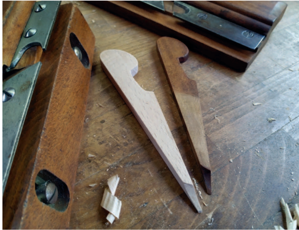
Supporting the wedge in its cradle while planing to thickness (above). The tip of the wedge is carved with a curiously skewed hollow (right). The iron of a wooden plough (on the right, below) is too wide for the grooving plane
