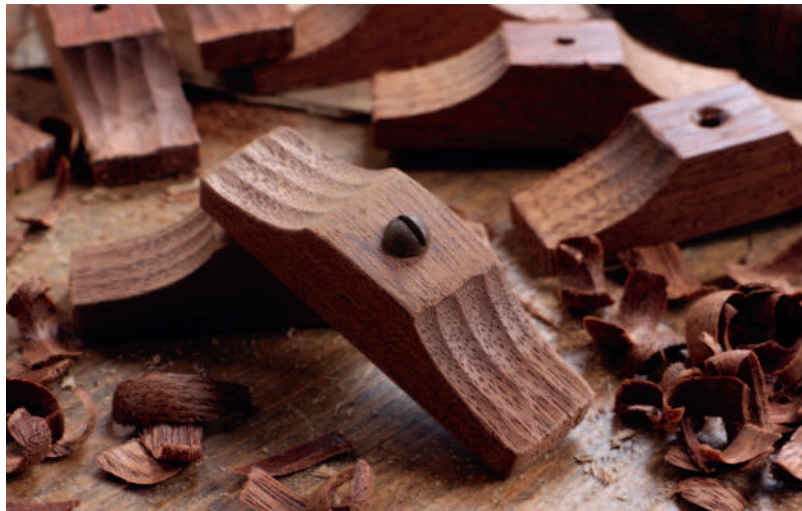
A panel saw secured by a button in the lid of a joiner's toolbox (above). A button (below) ready for fitting with the corners and edges rounded
