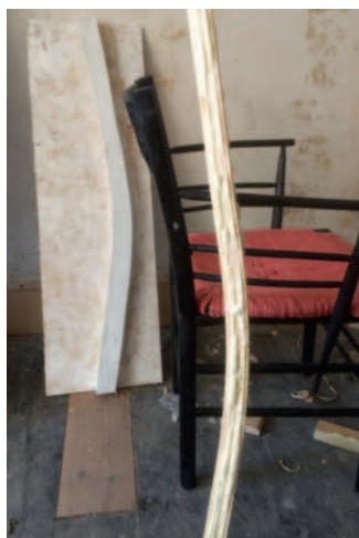
Using strips of 6mm pine from B&Q has meant the back legs can be shaped by laminating (left). The former has recently been adapted to make the curve tighter, particularly below the seat rails (above)
