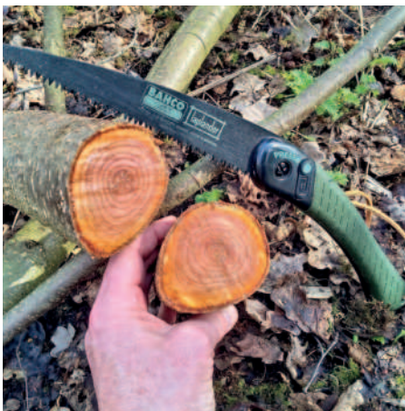
Tightening the screw (above) on the Bahco Laplander eliminates wobble for cutting hazel (below right) and 3in alder fast and easily
