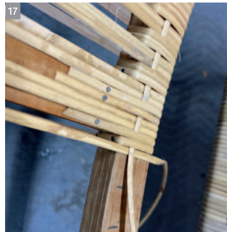
17 Once the centre support is reached use short pieces tacked to the center rail to continue the pattern. This step can be confusing but working slowly and thoughtfully will help get through it with minimal frustration
