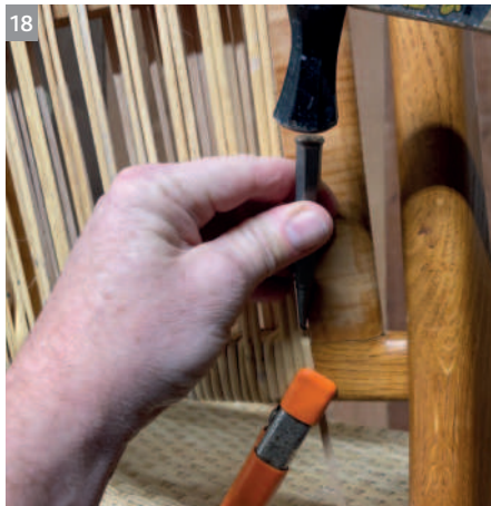
18 Continue on until the last warps and, like on the seat, pay attention to how the trim strip ends. Finish with a single wrap around the back of the bottom rail. A nail set can reduce the challenge of nailing in this tight space
