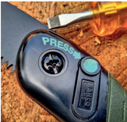
Tightening the screw (above) on the Bahco Laplander eliminates wobble for cutting hazel (below right) and 3in alder fast and easily
