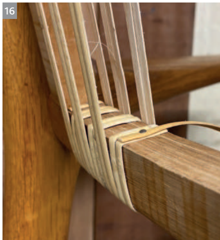
16 Continue until the centre rail is reached. If a new piece of cane is needed add it by nailing the new over the old then trimming the ends. One nail holds both pieces
