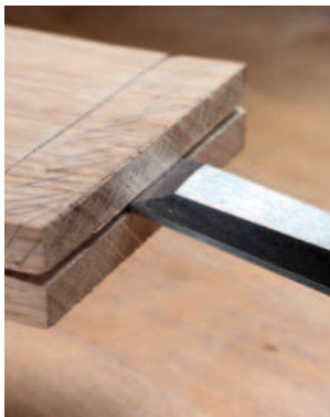
Breaking out waste from a sawn rebate (left), ripping a rebate with a Double Century tenon saw (right) and driving copper boat nails with a pin hammer
