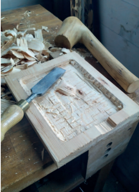
The blade of a Hall's 'Modern' spokeshave is adjusted by flush-mounted captive screws (above). Waste for a useful wood tray (below) is cleared with a firmer chisel (left)
