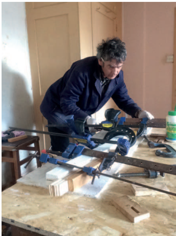
Using strips of 6mm pine from B&Q has meant the back legs can be shaped by laminating (left). The former has recently been adapted to make the curve tighter, particularly below the seat rails (above)
