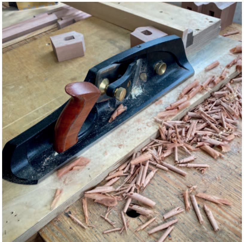
Use a sacrificial board made of softwood (above) to support the back face of your workpiece rather than remake with a new back stop. The Veritas Shooting Plane in situ (right)
