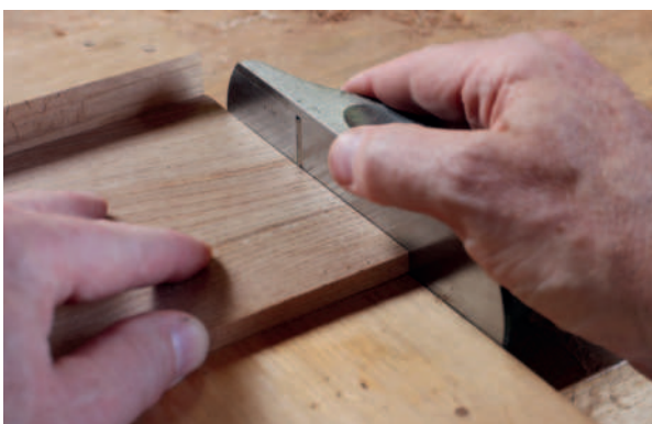
Shooting a square end for the elm base (left) and scribing a rebate to accommodate the lid pull (right)
