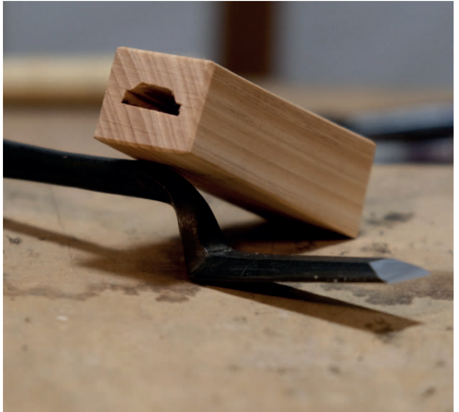
The case I will be making is for this Kote Nomi (goose-neck chisel). This chisel is used in places where the handle on a standard chisel would interfere, such as when cleaning grooves. For the wood, I had picked up a scrap piece of Hinoki (Japanese cypress)
