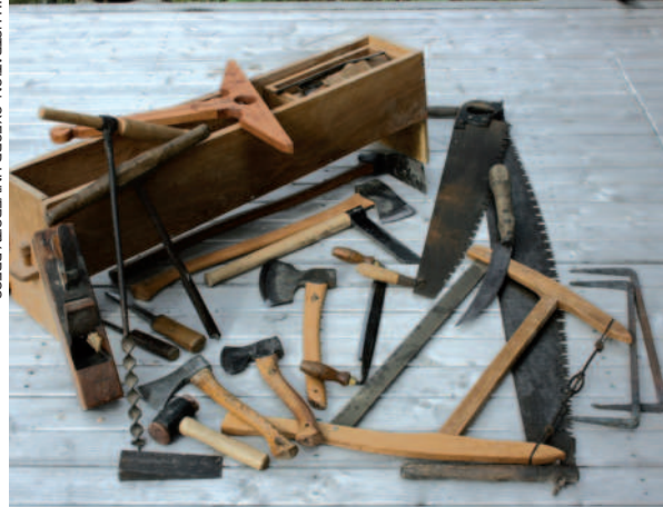
Illustration (left) from Building in England Down to 1540 by Salzman (with permission of Oxford University Press (oup.com)). A medieval carpenter's toolbox was likely to include: cross-cut saws; a frame saw; hand saw; felling axe; hewing axe; hand axes; drawknife; adze; froe; chisels; holding dogs; spoon bits; drilling augers; level; pairs of compasses; marking awl; string and chalk lines; square; and plumb bob. A Carpenters Fellowship course in 2008 (left) at Cressing Temple, Essex was a biblical scene, with a small building being constructed with traditional techniques and green timber. The tools were much the same as those to be found in a medieval toolbox
