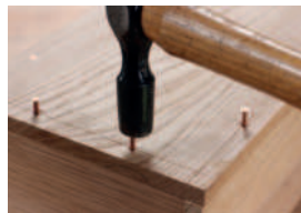
Breaking out waste from a sawn rebate (left), ripping a rebate with a Double Century tenon saw (right) and driving copper boat nails with a pin hammer
