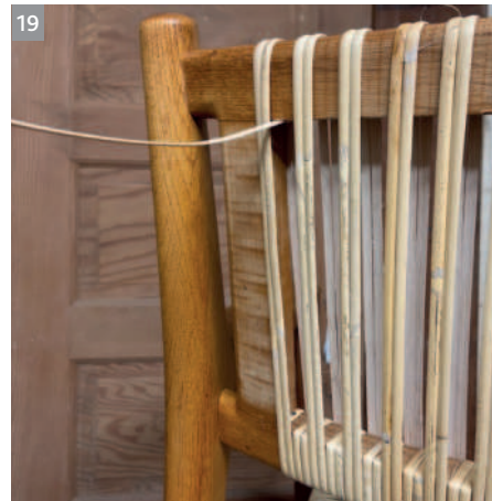
19 Wrap the spaces between the warps of the top rail. Begin by nailing a piece of cane to the bottom of the top rail at the left side between the first and second warp sets with the working end going out toward the back
