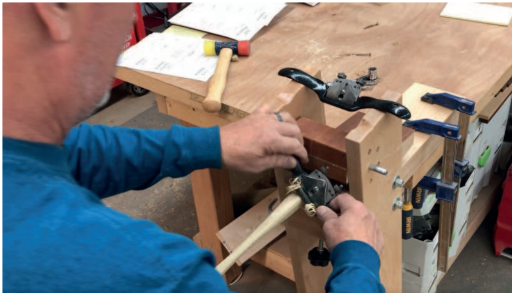
The jaws of the shaving pony can be adjusted to vary the angle. Follow Dan on Instagram @seasmokedesign for more details
