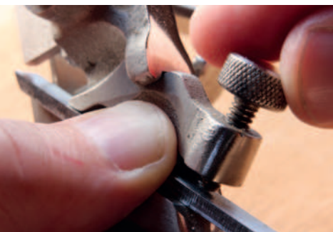
A thumb secures the lever cap while the cutter is adjusted (left) and clearing jammed shavings with a lolly stick (above)
