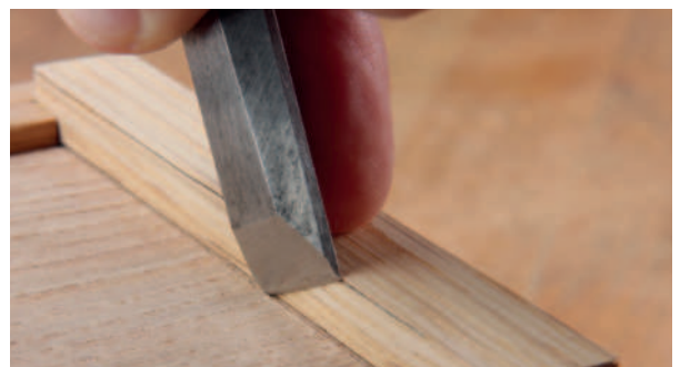
Shooting a square end for the elm base (left) and scribing a rebate to accommodate the lid pull (right)
