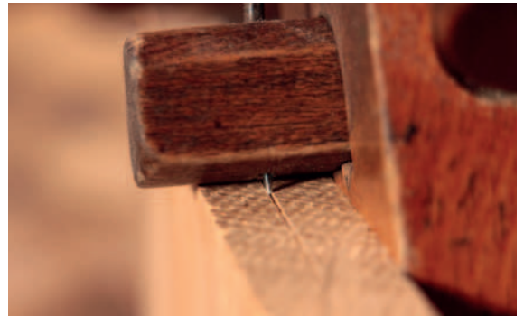
Scribing the depth of a corner rebate (left) and using a marking gauge on the end-grain (right). Test fitting of a chiselled corner rebate (below left) and chiselling waste from a corner rebate (below right)
