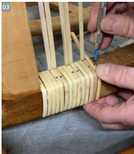
03 Nail on the inside of the rail. The nails will be covered with a piece of split rattan so be sure to keep the nails in line
