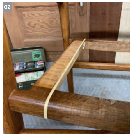
02 Tack a piece of cane on the back rail 1/2in from the bottom edge in the corner with the working end down. Bring it over the outside of the rail, across the seat, around the front, and tack it down as you do on the back
