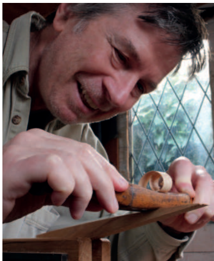
Shavings curl like butter from the 'Modern' spokeshave (above). Carving characteristic grooves for a Wagatabon with a 3/4in gouge (below)
