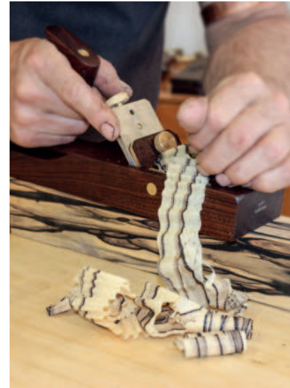
A Dado Plane (left) and an A55 Plane (above) smoothing some black and white ebony
