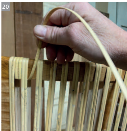
20 Don't forget the trim piece. Simply wrap the top rail until there are at least two wraps on both sides then pass the cane over to the next area to be wrapped and continue
