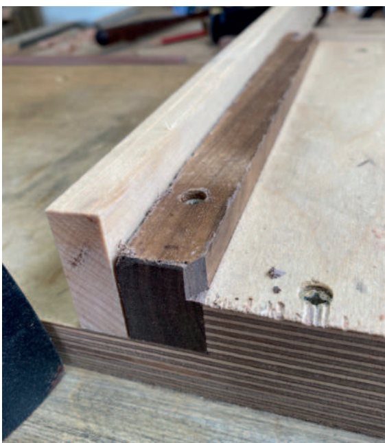
Use a sacrificial board made of softwood (above) to support the back face of your workpiece rather than remake with a new back stop. The Veritas Shooting Plane in situ (right)
