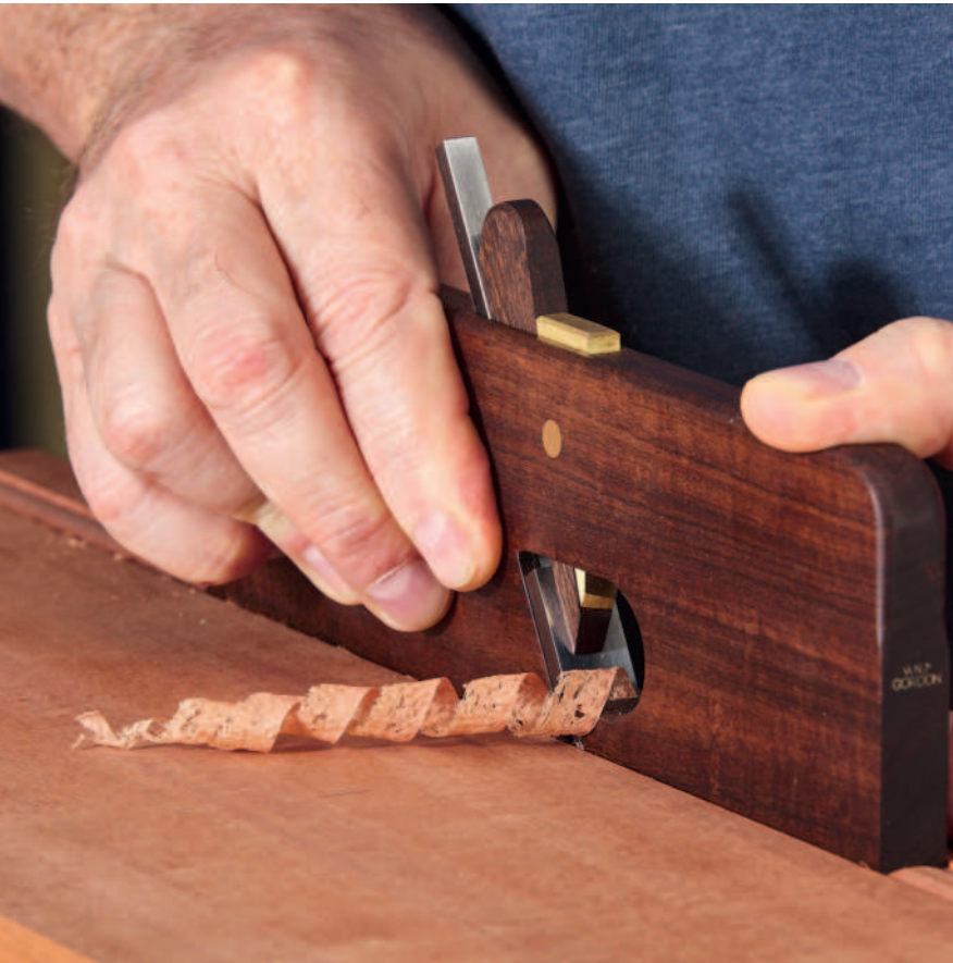
The 1/2in hollow plane (left) being used to make a bead, 1/8in dado plane (above) and a ringed gidgee A55 smoothing plane (below)
