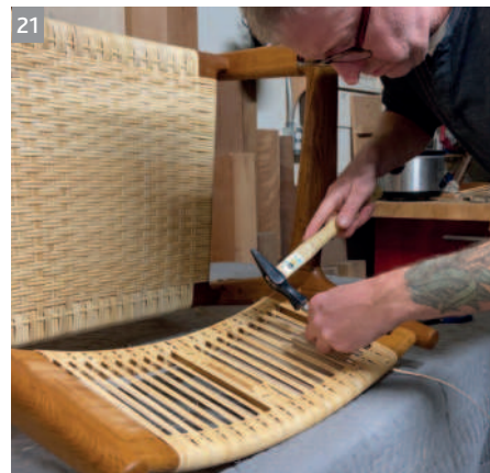
21 When a new piece is needed nail it on over the old one on the inside of the rail. At the center support use short pieces nailed to the support to continue the pattern. Finish by nailing the end to the underside of the top rail
