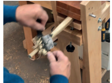
The jaws of the shaving pony can be adjusted to vary the angle. Follow Dan on Instagram @seasmokedesign for more details
