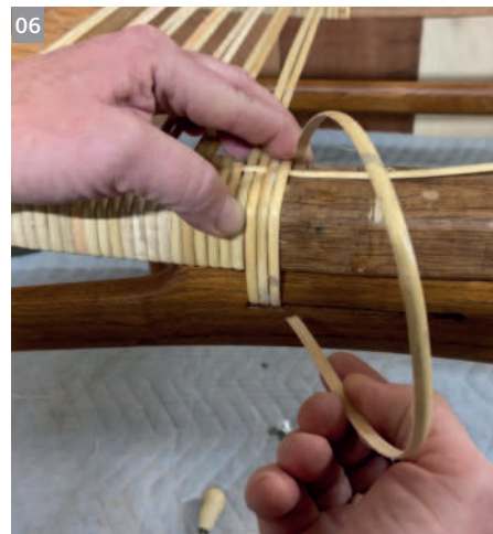
06 The centre detail is easily managed. Just continue over the rail until the slot is reached, then go through the slot
