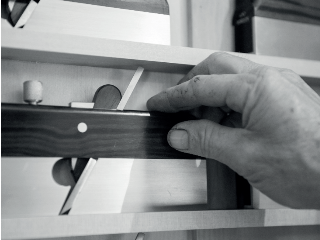
A Dado Plane (left) and an A55 Plane (above) smoothing some black and white ebony
