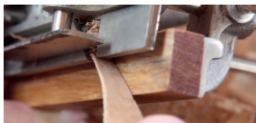
A thumb secures the lever cap while the cutter is adjusted (left) and clearing jammed shavings with a lolly stick (above)
