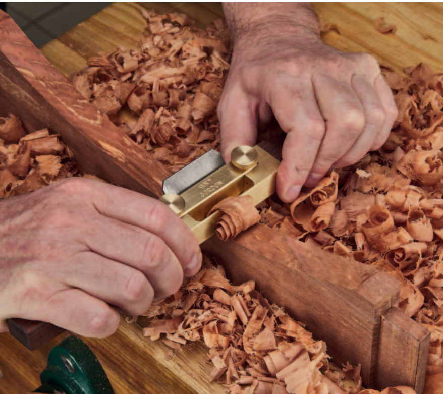
A customer using a Curved Sole Spokeshave (left) in some Tasmanian Myrtle, and the HNT Gordon Pattern Makers Vice (above)
