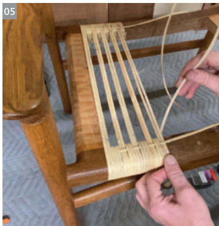
05 Pay close attention to your layout marks and try to follow them as best as possible while also keeping the cane packed tightly next to each other so the rail cannot be seen
