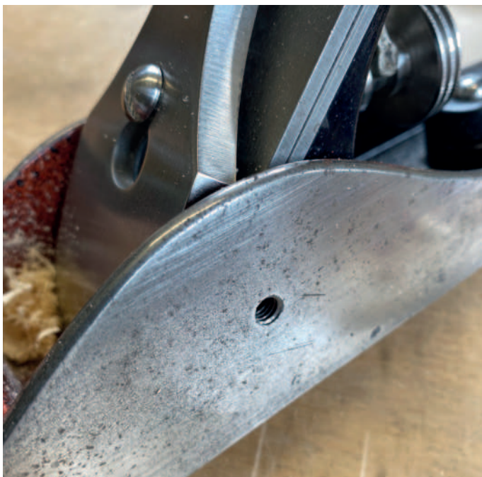
Drill a 5mm hole in the side wall of a bench plane (above) and tap for a 6mm thread. A home-made version of a T5 (right)
