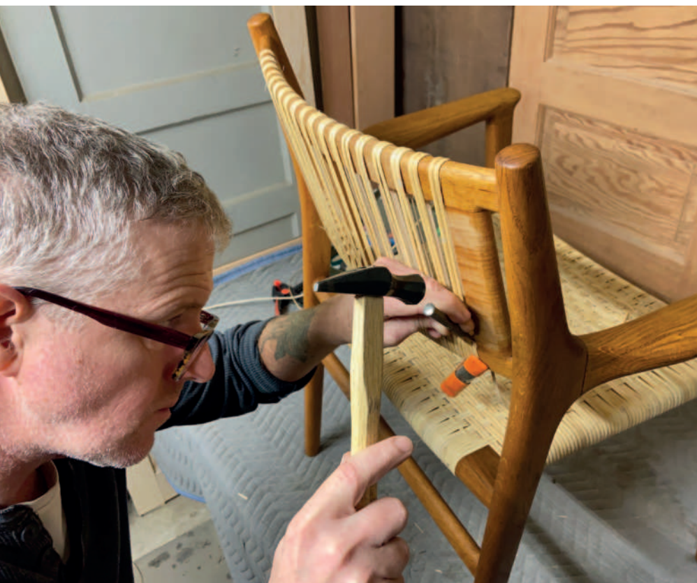
A nail set can reduce the challenge of nailing in a tight space
