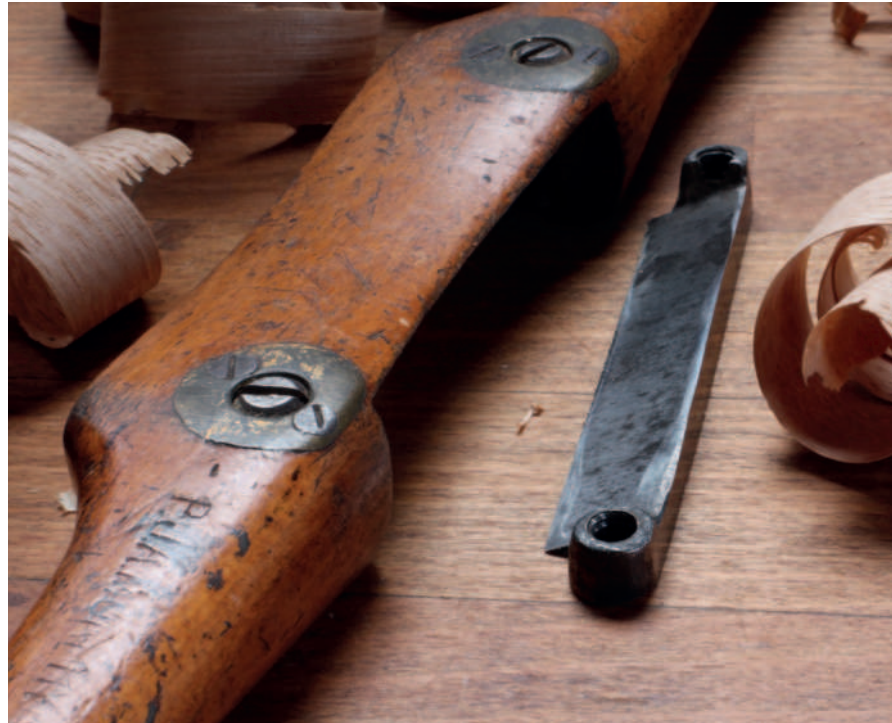
The blade of a Hall's 'Modern' spokeshave is adjusted by flush-mounted captive screws (above). Waste for a useful wood tray (below) is cleared with a firmer chisel (left)
