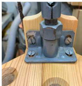
An upstand strengthens the lamp to the base (left) with a peg at the back as a fixing -pivot (above)
