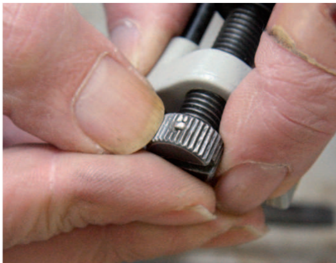
David has his waterstone sitting on a rubber mat available in the 'home & leisure' section of the medical products shop, dycem.com . His measured 35x25cm. On the original Eclipse version of the honing guide there is a pin you can tap out so the knurled knob can be removed
