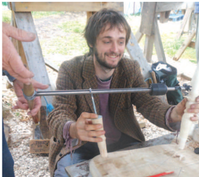
Peter using the Westonbirt Woodworks hook tool (in his right hand) to help level the extended auger to drill chair legs. A model of the seat & legs inspired by Quercus , and his milk paint
