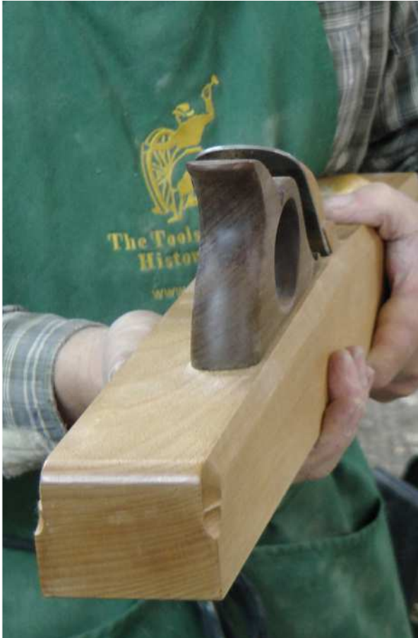
Holding the handle with your fingers along the side of the plane (right) is even more comfortable when the tote is offset (above).
