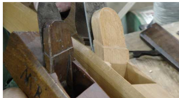
The original panel-raising plane by Robert Wooding of London dating to around 1710. This was the inspiration for my own wedge pattern (left). Note how the upper portion of the wedge is relieved across its width. This has an advantage when laterally adjusting the iron as there is less chance of accidentally striking the side of the wedge with a hammer
