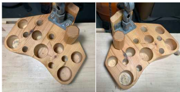
The peg is used to locate the base in three angles on the bench
