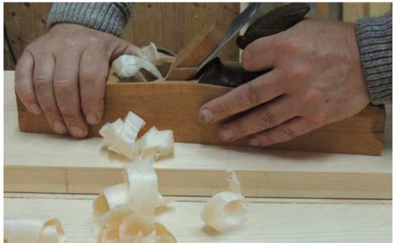
Holding the handle with your fingers along the side of the plane (right) is even more comfortable when the tote is offset (above).
