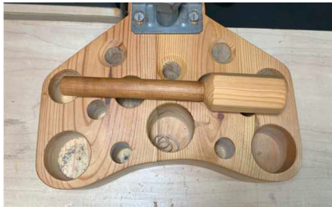
The peg is used to locate the base in three angles on the bench
