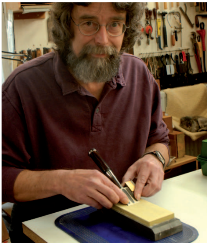
David has his waterstone sitting on a rubber mat available in the 'home & leisure' section of the medical products shop, dycem.com . His measured 35x25cm. On the original Eclipse version of the honing guide there is a pin you can tap out so the knurled knob can be removed
