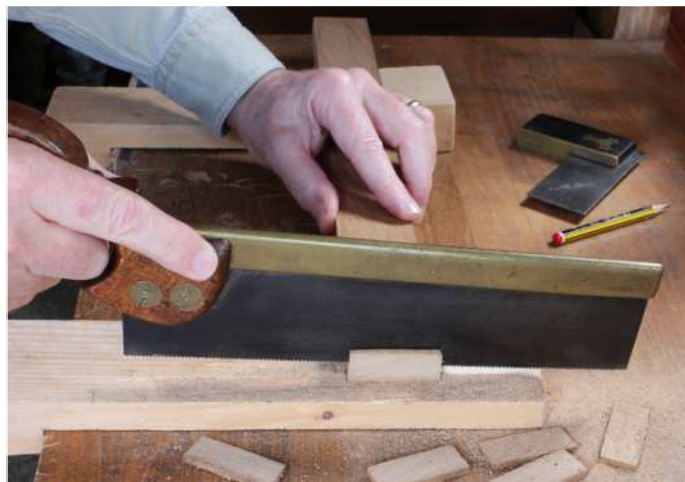
The basic idea of making a pair of bench hooks is not new, shown (right) in a 1902 edition of The Woodworker . With the improved version (above) the kerf doesn't foul on the workbench
