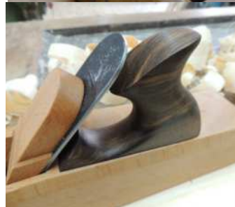
The original panel-raising plane by Robert Wooding of London dating to around 1710. This was the inspiration for my own wedge pattern (left). Note how the upper portion of the wedge is relieved across its width. This has an advantage when laterally adjusting the iron as there is less chance of accidentally striking the side of the wedge with a hammer
