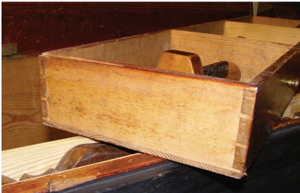
Richard has made a holder for saws (above) to fit in the gap at the front of the tool chest, beneath the trays of other tools (below). The drawers are all dovetailed, with nailed-on bottoms (left) and provide good access (below)
