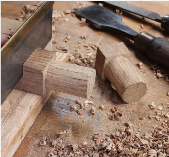
Planing oak with the wooden stop and bench dogs (above). The dogs need to be cut to the required length (left). The wooden planing stop (below) and the blind mortise
