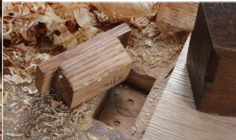
Planing oak with the wooden stop and bench dogs (above). The dogs need to be cut to the required length (left). The wooden planing stop (below) and the blind mortise
