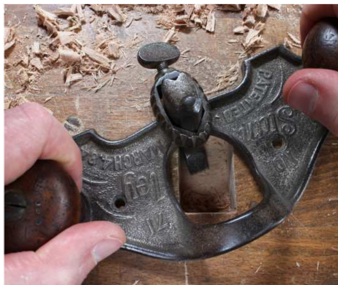
Boring the bench for a blind mortise (above), and then levelling the mortise floor with a Stanley 71 router (below)
