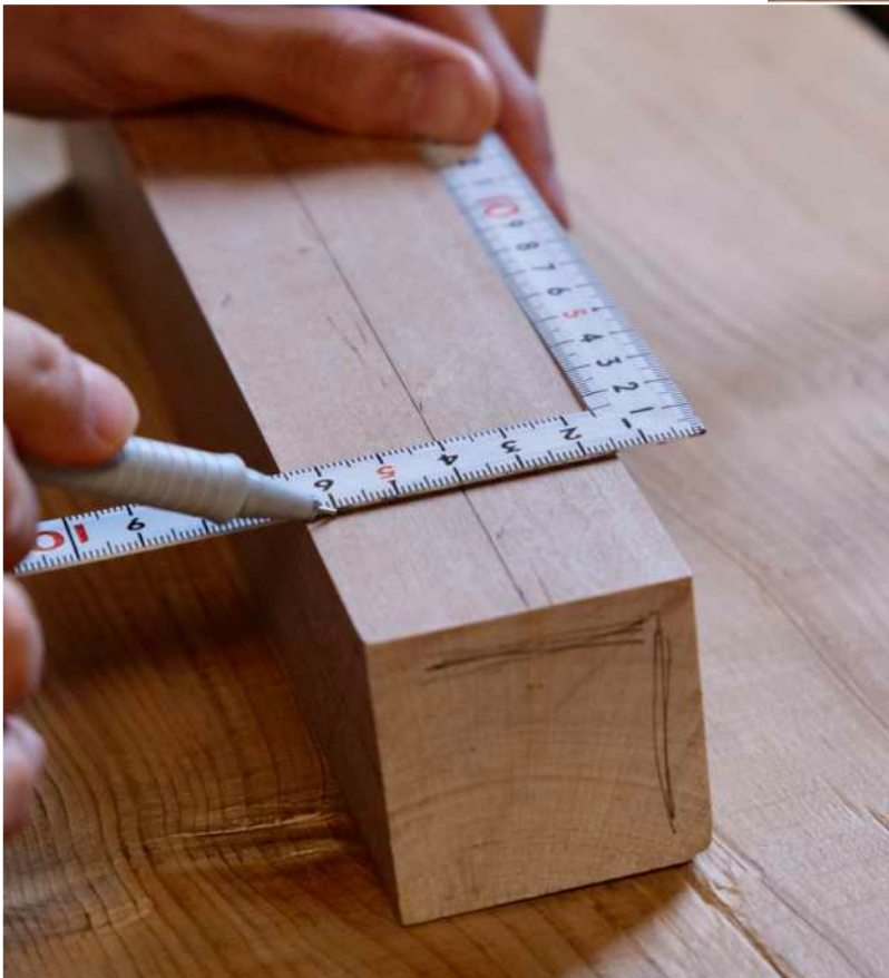
Pic.3 The lines on the end-grain (below) show the reference surfaces I decided on. Making sure always to place the square against one of the reference sides reduces the margin for inaccuracy.
