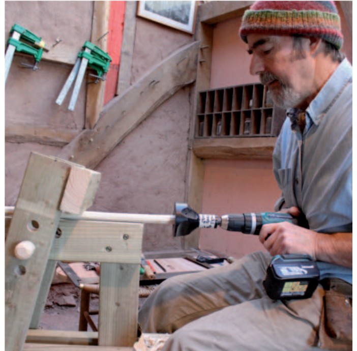
By keeping the bed horizontal you can keep a tenoner level
