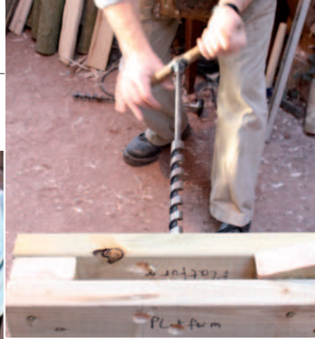
Drilling the platform with a Forstner bit (above) for the pivot, or use and auger (left)
