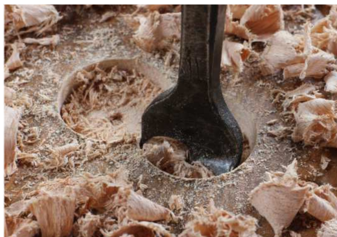
Boring the bench for a blind mortise (above), and then levelling the mortise floor with a Stanley 71 router (below)
