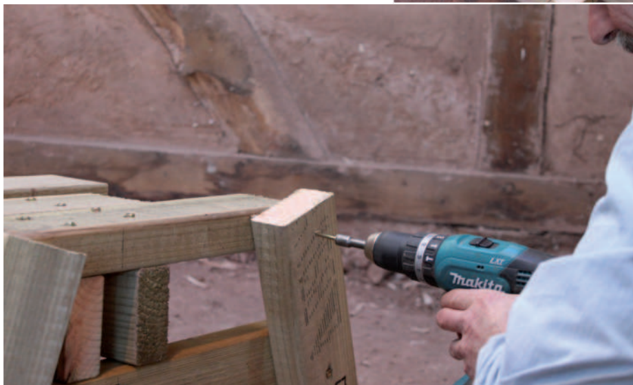
Fixing the bed to the riser (above). The pivoting clamp (right) is made from the same stock as the rest of the shaving horse, with the top bar or jaw screwed to the arms. Screwing the back legs in position (below)
