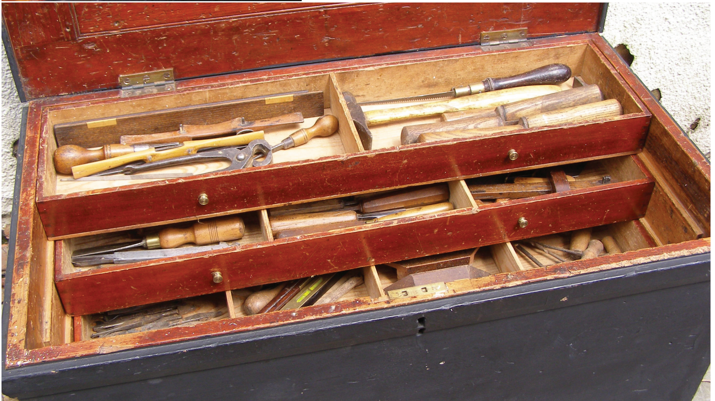
Richard has made a holder for saws (above) to fit in the gap at the front of the tool chest, beneath the trays of other tools (below). The drawers are all dovetailed, with nailed-on bottoms (left) and provide good access (below)
