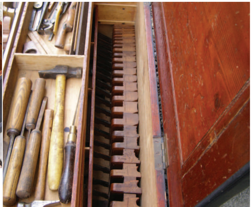
Beneath the three open-topped drawers are divisions for rows of moulding planes (right). Richard thinks the chest was made for a joiner as so many of the tools would have been used for making sash windows
