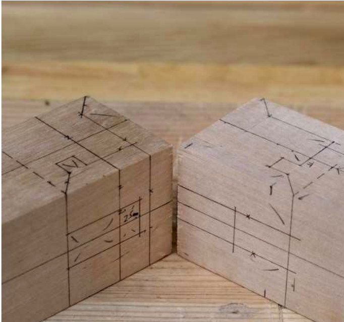
Pic.2 The different symbols in the markings (above) show the tasks to be done. The 'X' represents the cut lines and the 'flicks' show the parts to be removed. An exciting part of making joinery for the first time is never completely knowing if the markings are correct until it is cut.
