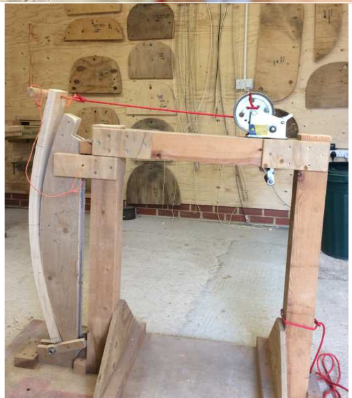
The arm-bending jig (above) and the rocker-bending jig (below right)
