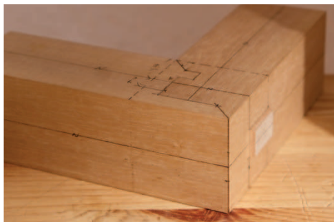
Pic.8 It's important to take your time when marking the lines (left). Once marked, visualise the completed shape and make sure the lines are marked where they need to be. A mistake at this step can have consequences later
