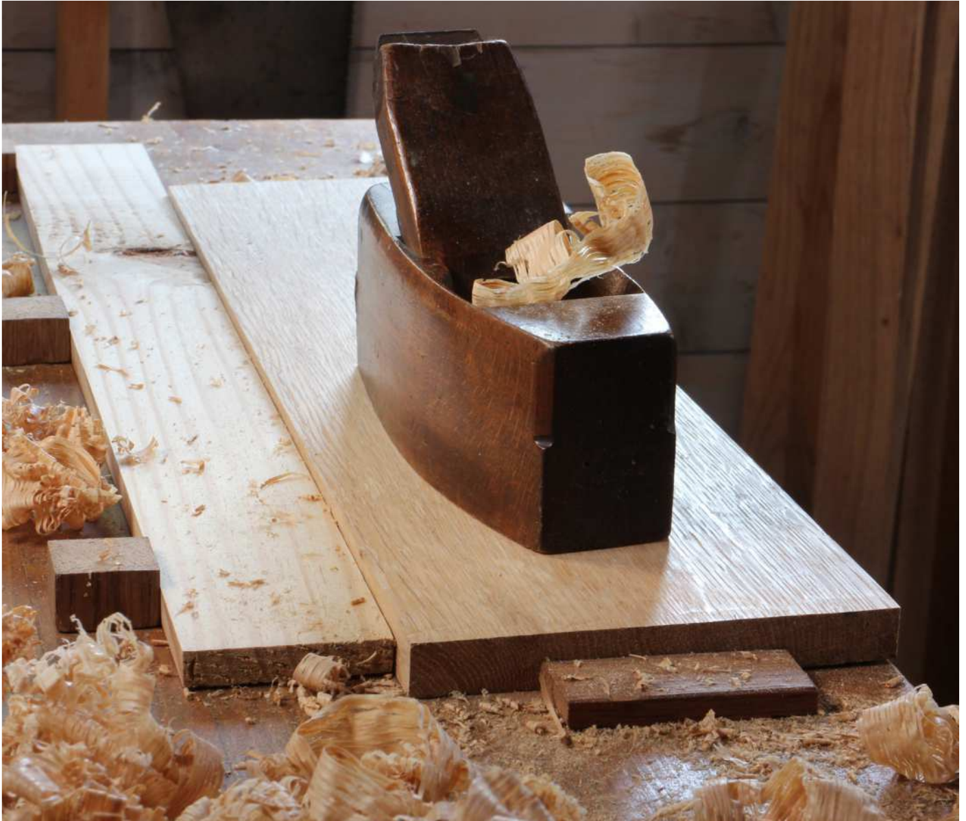
Planing oak with the wooden stop and bench dogs (above). The dogs need to be cut to the required length (left). The wooden planing stop (below) and the blind mortise
