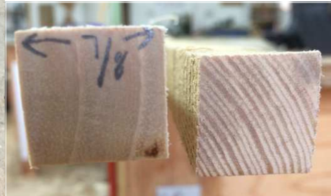
James Mursell's crest-bending jig (above). Fast-grown ash (on left, below) is easier to bend than slow-grown ash (on the right, below)
