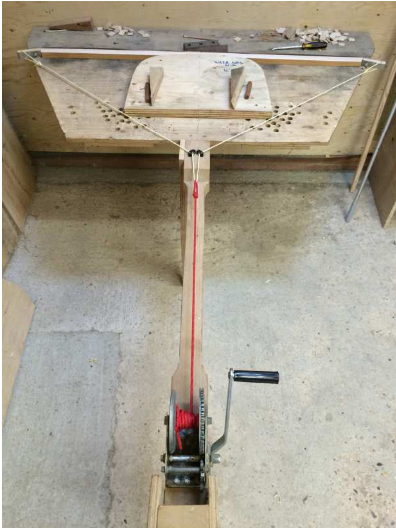
The arm-bending jig (above) and the rocker-bending jig (below right)
