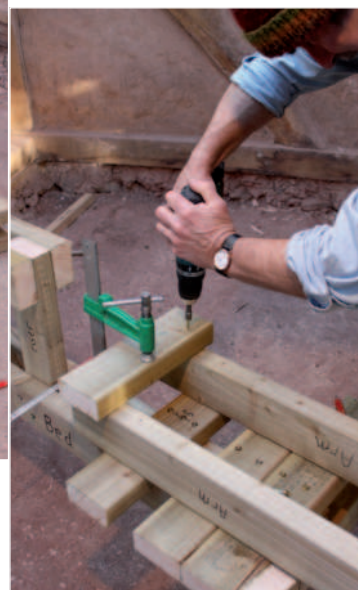
Check the spacer at the rear (above left) is square to the bed. Fixing the longest of the seat components to the back end of the bed (above)
