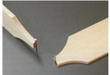
Rare earth magnets are embedded into the simple tool for holding small nails or pins while they are started in wood
