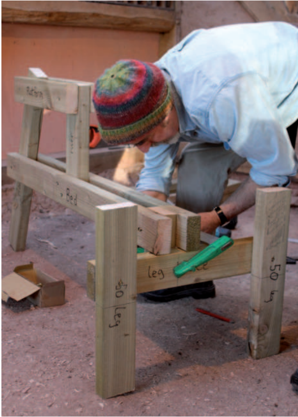
The back leg assembly is offset from the bed by 10cm (above) and taking a test ride with a soft saddle
