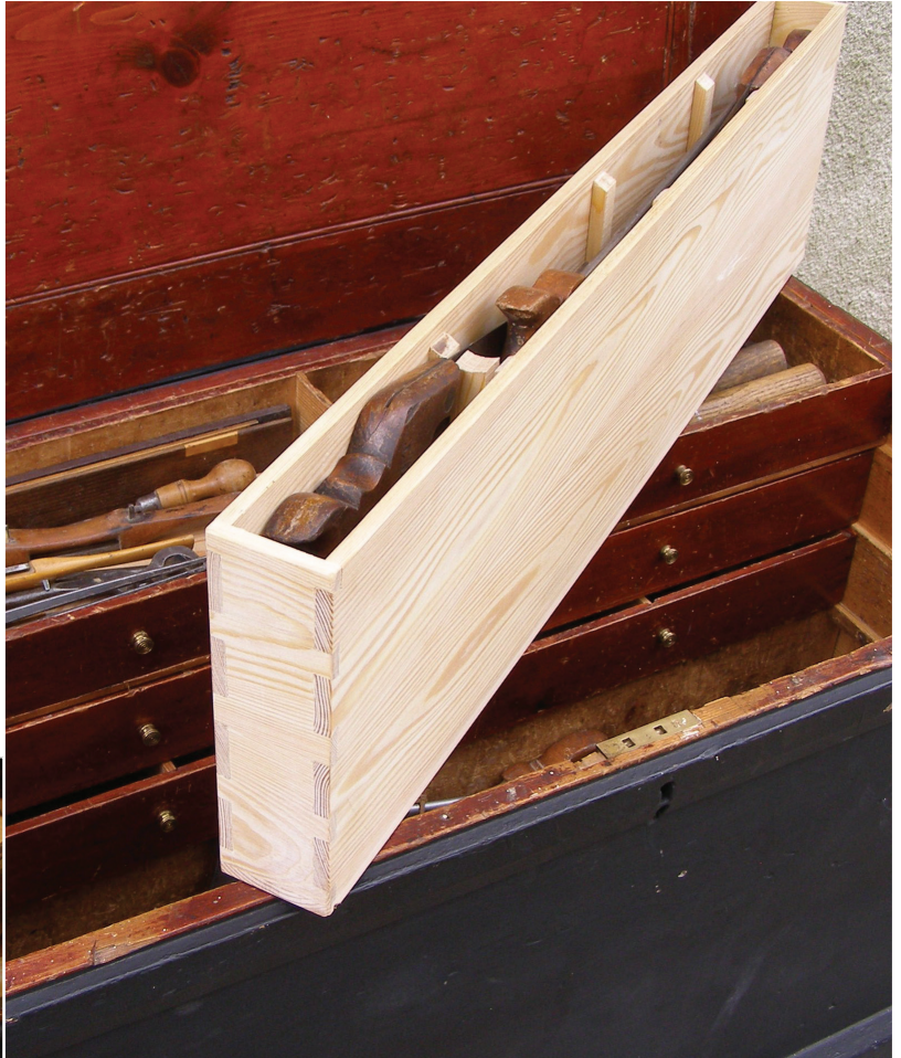
Richard has made a holder for saws (above) to fit in the gap at the front of the tool chest, beneath the trays of other tools (below). The drawers are all dovetailed, with nailed-on bottoms (left) and provide good access (below)
