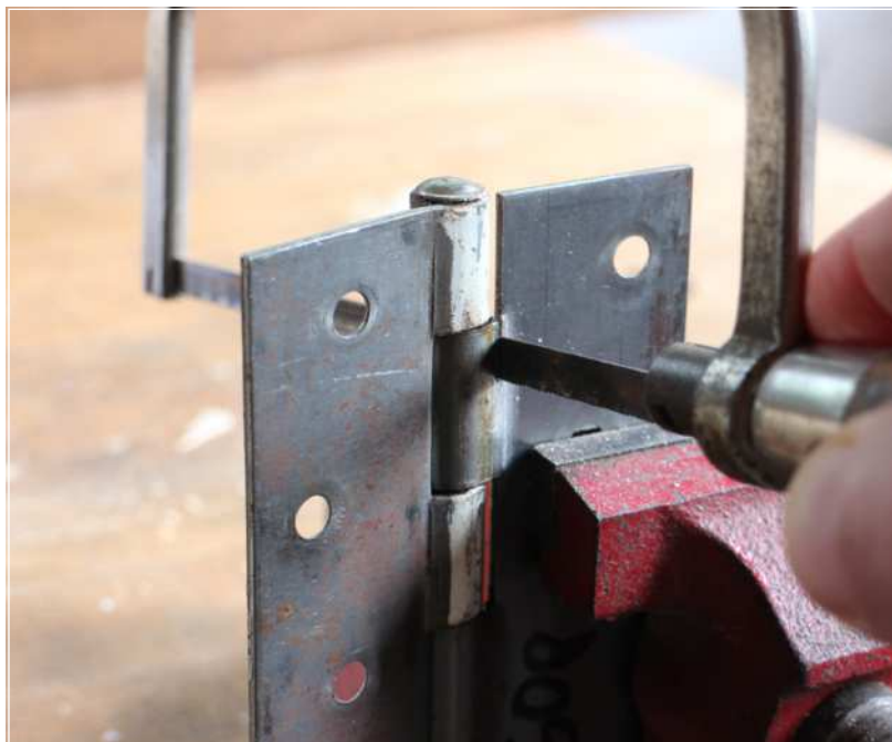
Cutting the steel hinge with a Junior 670 hacksaw for the toothed stop
