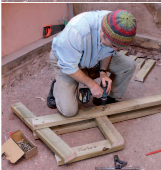
Fixing the bed to the riser (above). The pivoting clamp (right) is made from the same stock as the rest of the shaving horse, with the top bar or jaw screwed to the arms. Screwing the back legs in position (below)
