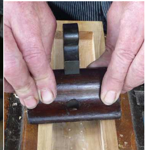
A Granny's tooth (below) was used to level the base of the oilstone box
