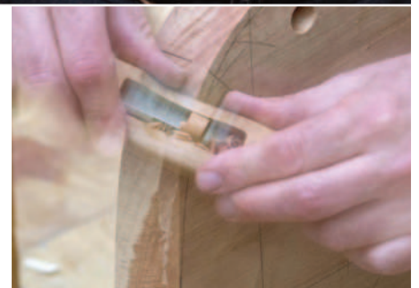
When James Mursell uses a wooden spokeshave he has his thumbs very close to the blade and holds the tool very lightly
