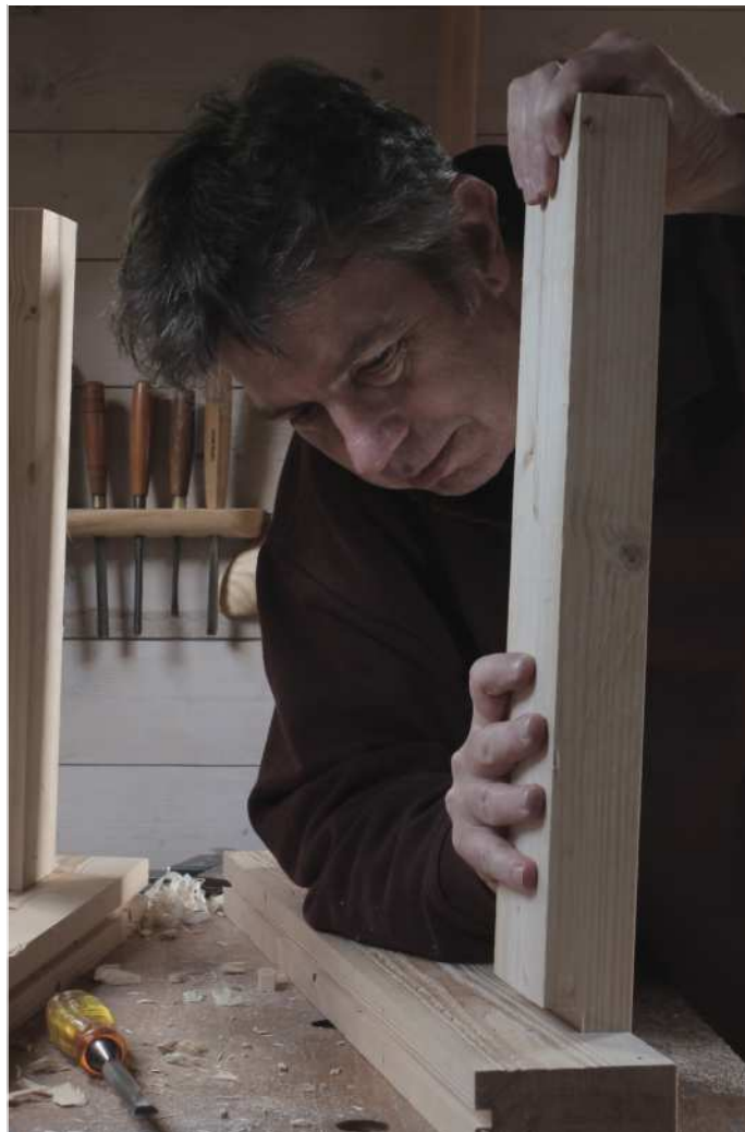
Test fitting the legs before assembling the top (above) and flattening the top with a Marples jack plane (below)
