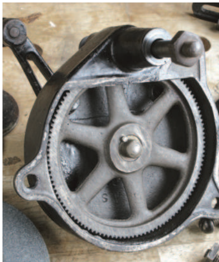
A plywood swarf-catcher (above) clamped beneath the wheel contains the mess and prevents damaging the wheel. Removing the grinding wheel and side plate (left) gives access to the main drive wheel
