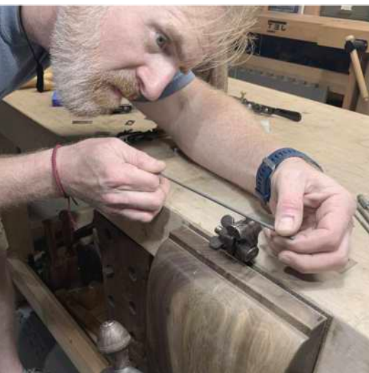
The author touches up a bead cutter with a chainsaw file (left). Files can be used to create your own profiles (above). The original Preston 1393S with the original No.6 cutter and an example of the profile it cuts (right)
