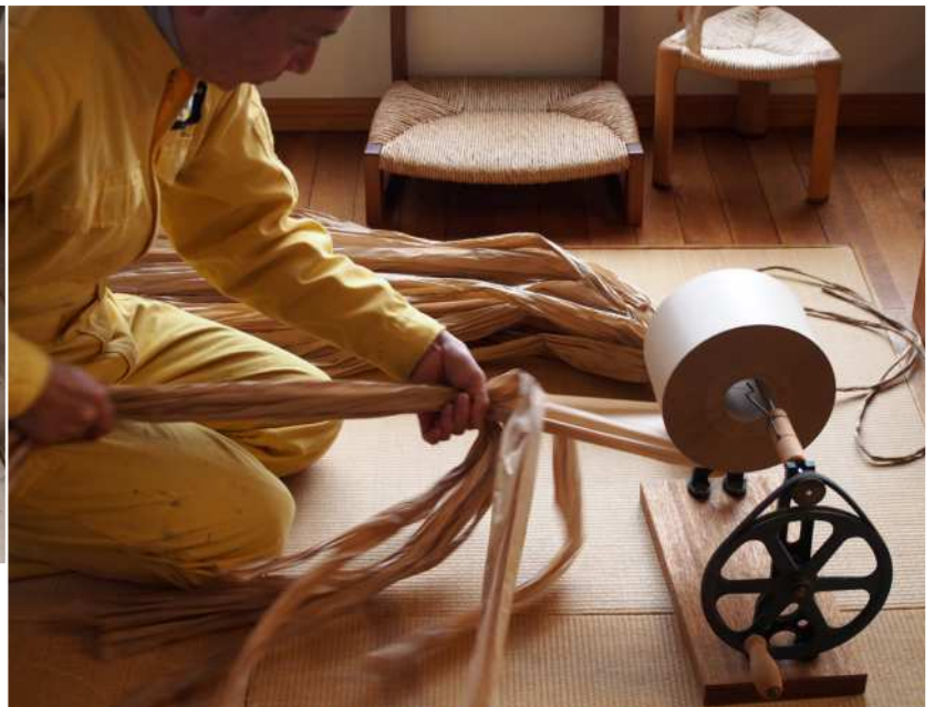
Mitsuru uses Japanese slit tape about 12.5cm wide (above). The slit tape is cut into 2.3m lengths, using a bobbin tool because it is convenient. The tape is wrinkled (right) to make twisting into string easier
