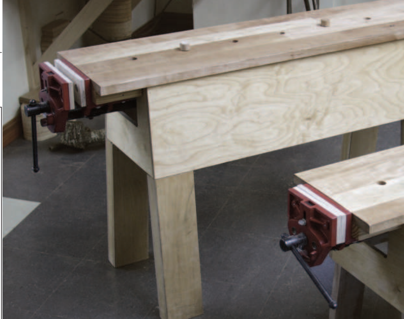
Benches at Clear Spring School are designed to raise the height of the workbench for the height of larger children. A vise at each end allows the bench to be used by two students at a time. Blocking (left) is necessary on the underside for the vice to sit flush with the benchtop. Note the cutout in the end of the bench frame for the mechanism to move through it
