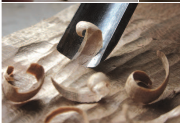
The chipped gouge (above left) and after grinding (above) is then honed for carving (left)
