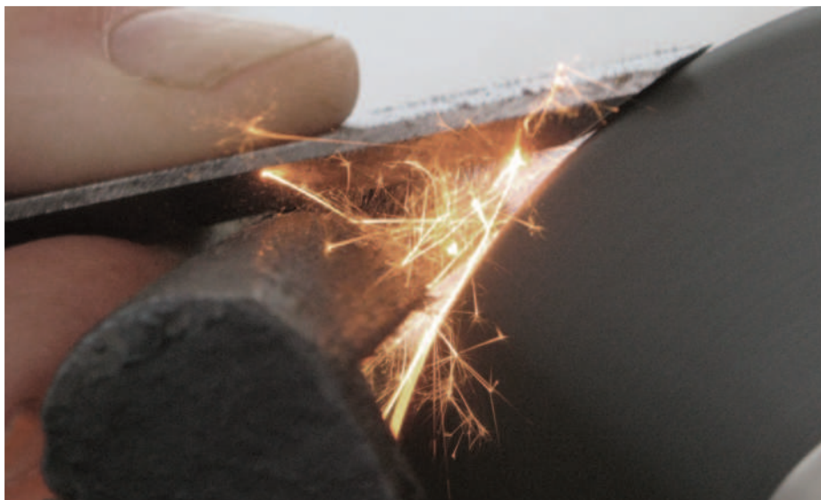
The sparks fly downwards (above). Swarf stuck to the wheel may go in any direction. The maker's plate (left). Silicon carbide developed by Edward Acheson's Carborundum Company was the first synthetic abrasive
