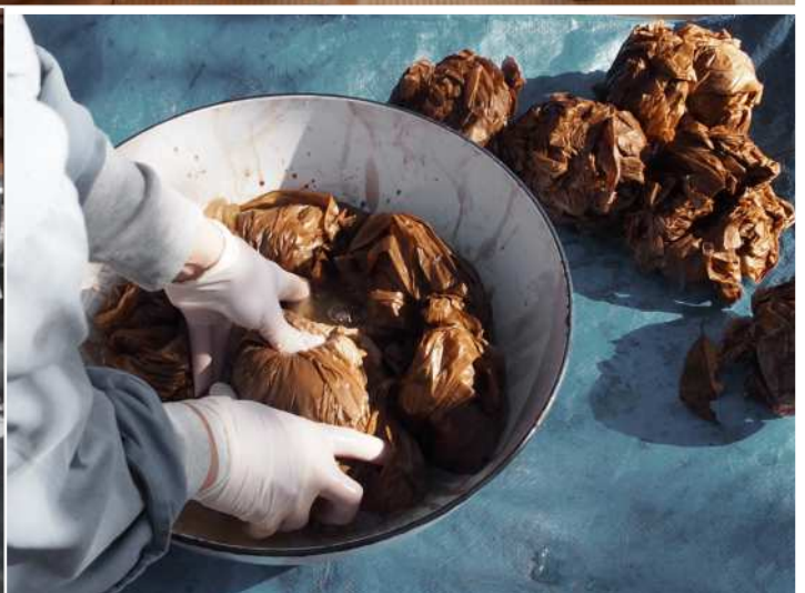
Having been wrinkled the tape is dyed with persimmon astringent (above). Each block is made up of 10 slit tapes. After that mordant is added to change the colour. The mordant can be sodium carbonate, titanium liquid or wood iron acetate liquid. Afterwards the tape is dried (left) outdoors and the colour will improve when exposed to sunlight and oxygen. When it dries the slit tape will be wrinkled, ready to be twisted into string for weaving
