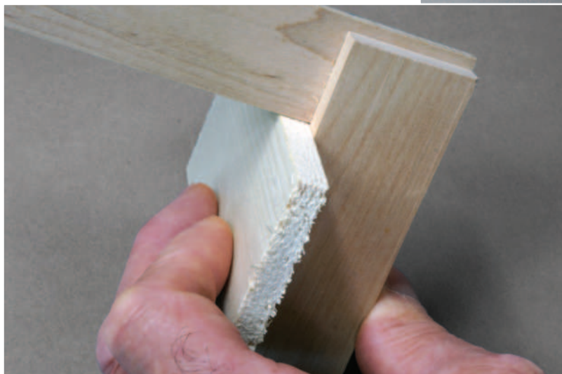
The square is useful when planing wood to make certain that the edge is kept square to the face (above). The students are encouraged to hold the square tightly against the wood so that it can be used on the edge for planing and the end to square up the ends of a workpiece (right)
