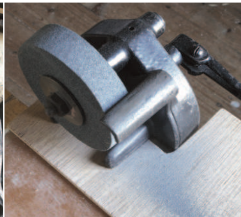
A plywood swarf-catcher (above) clamped beneath the wheel contains the mess and prevents damaging the wheel. Removing the grinding wheel and side plate (left) gives access to the main drive wheel
