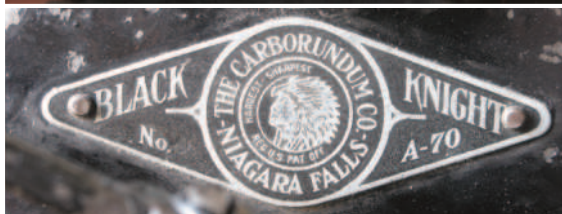
The sparks fly downwards (above). Swarf stuck to the wheel may go in any direction. The maker's plate (left). Silicon carbide developed by Edward Acheson's Carborundum Company was the first synthetic abrasive
