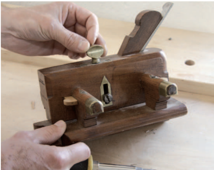
With the cutter removed and the fence drawn back (above) you can see the depth plate. Setting the depth stop (left) on a plough with a screw adjuster
