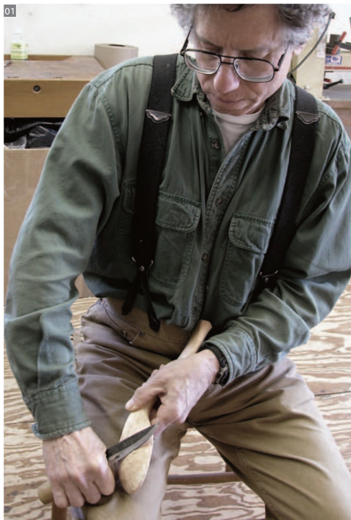
To remove wood from the outside of the bowl you hold the knife so the blade is facing away from you. Have the blade at a skew angle to the wood then use your elbow or shoulder for power
