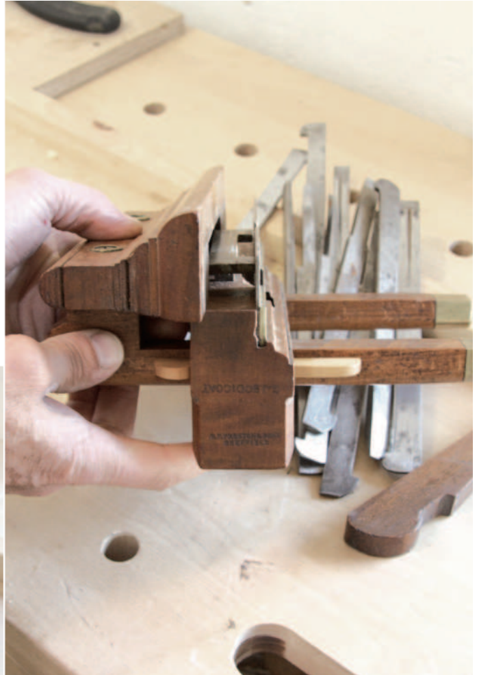
With the cutter removed and the fence drawn back (above) you can see the depth plate. Setting the depth stop (left) on a plough with a screw adjuster
