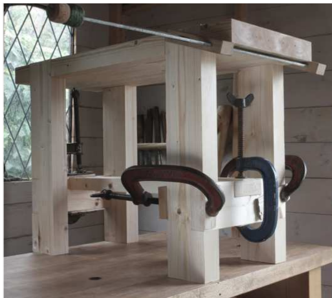
Test fitting the legs before assembling the top (above) and flattening the top with a Marples jack plane (below)
