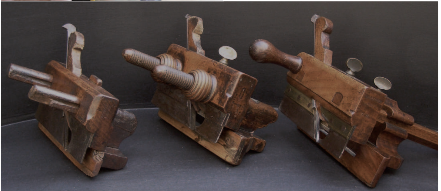
Three generations of plough plane (above), from an early model circa 1710 by Robert Wooding of London (above left), with a simple wooden depth stop. The screw-stemmed plough (above centre) by John Green of York is circa 1790, while the bridge plough (above right) is circa 1800
