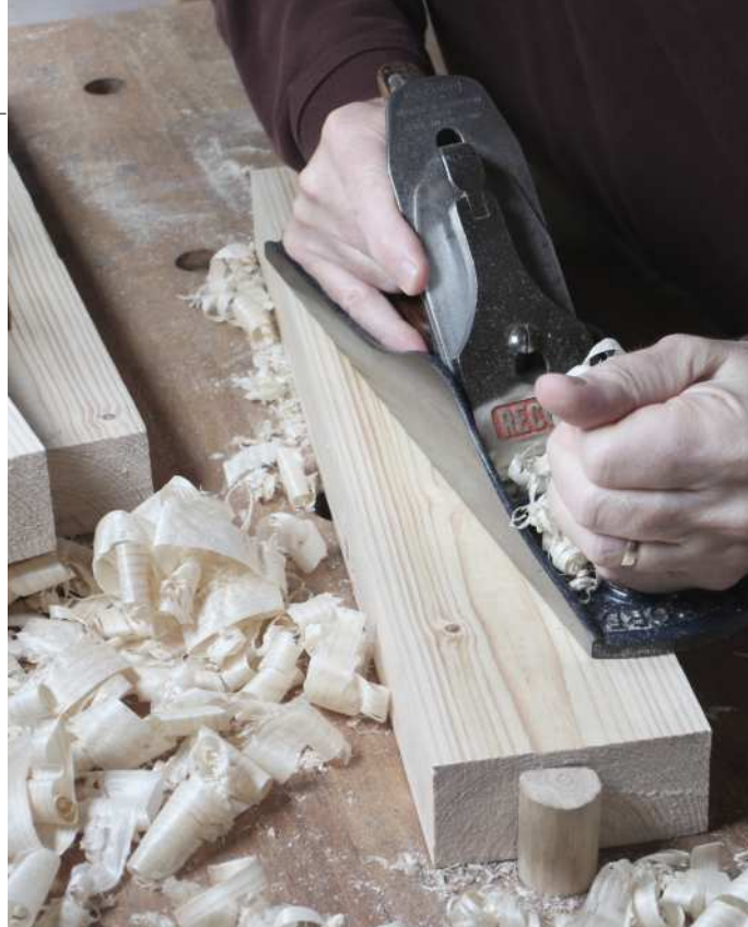
Flattening cupped faces with the Record 51/2 jack plane
