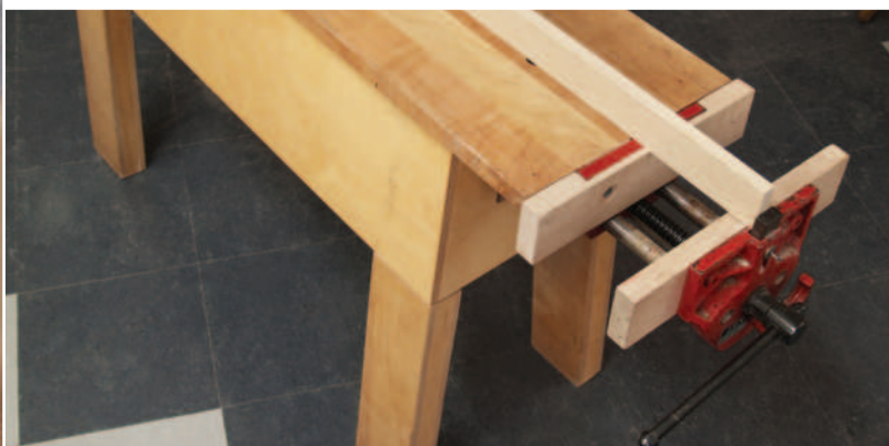
Benches at Clear Spring School are designed to raise the height of the workbench for the height of larger children. A vise at each end allows the bench to be used by two students at a time. Blocking (left) is necessary on the underside for the vice to sit flush with the benchtop. Note the cutout in the end of the bench frame for the mechanism to move through it
