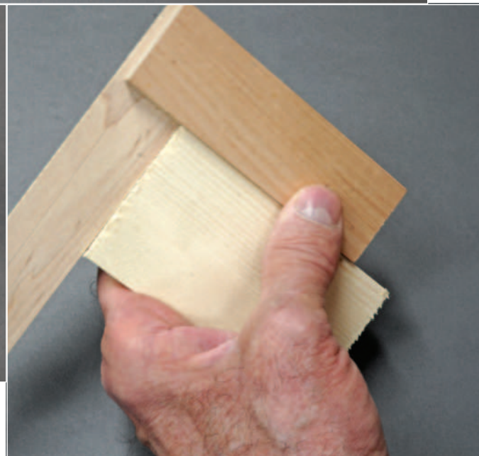
The square is useful when planing wood to make certain that the edge is kept square to the face (above). The students are encouraged to hold the square tightly against the wood so that it can be used on the edge for planing and the end to square up the ends of a workpiece (right)
