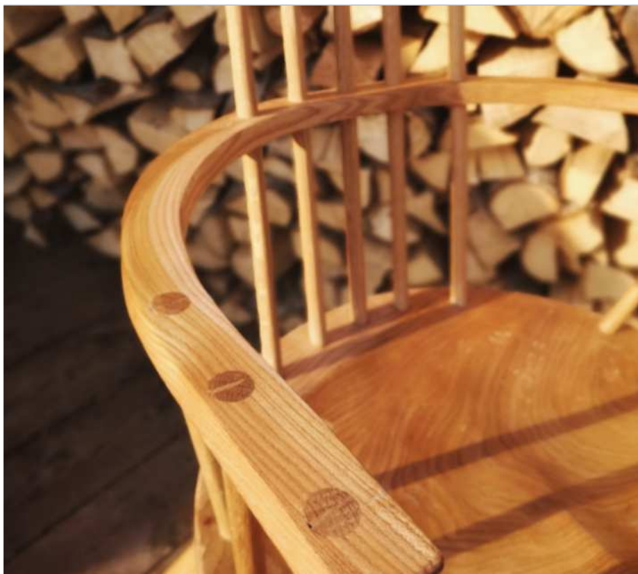
Klaus octagonises a tapers his chair legs with a jack plane on his workbench (left). The short sticks (above) are mortised through the steam-bent armbow and wedged from the top
