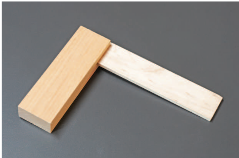
The two parts of the square are easy to make, and can be assembled by the students for their own use and to take home in their toolboxes
