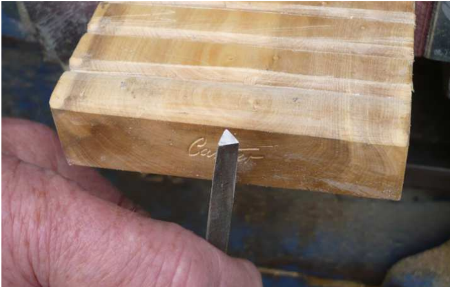
A Granny's tooth (below) was used to level the base of the oilstone box
